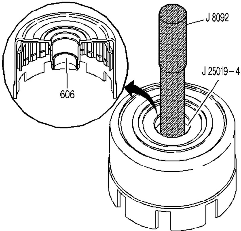
**Fig. 192: Locating Reverse Input Clutch Rear Bushing**
