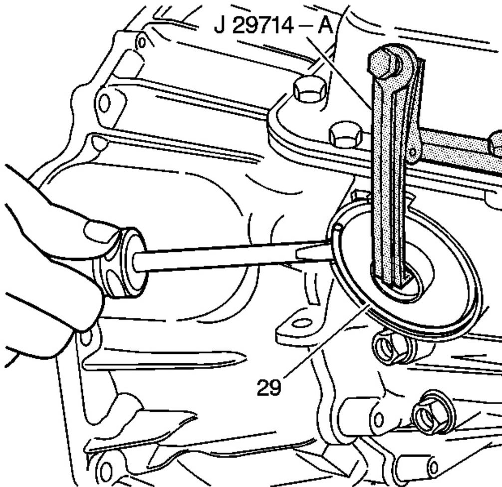
**Fig. 309: Locating Servo Cover Retaining Ring**
