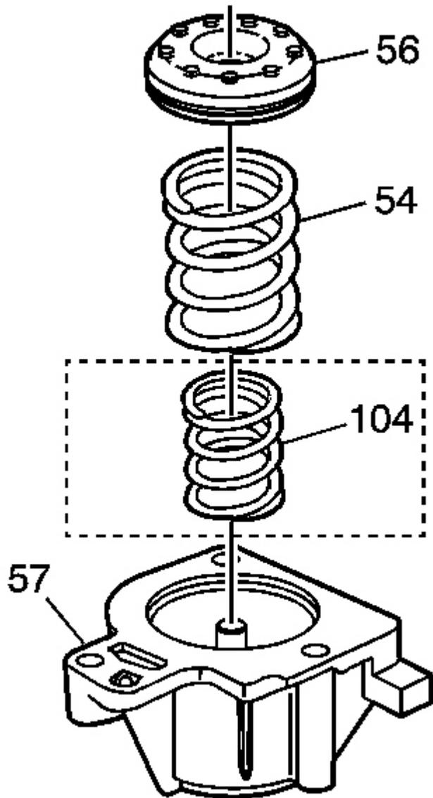
**Fig. 277: View Of 1-2 Inner & Outer Springs**
