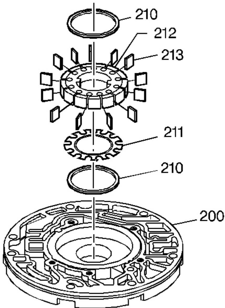
**Fig. 209: Identifying Pump Vane Ring Assemblies**
