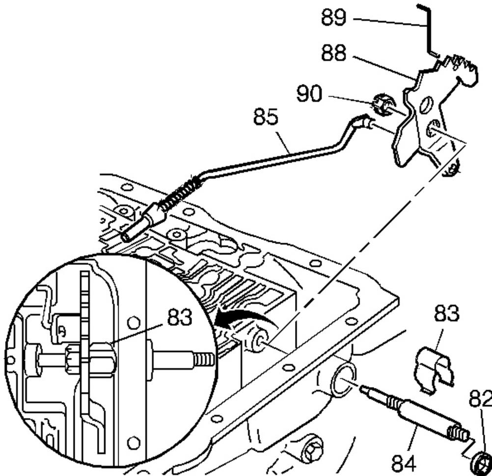
**Fig. 104: Identifying Inner Manual Linkage Inspection Areas**
