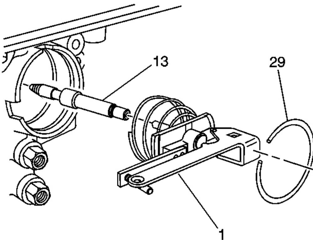
**Fig. 301: Locating Servo Cover Retaining Ring**
