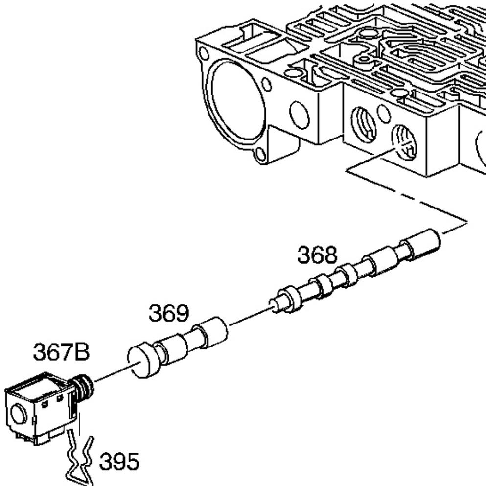
**Fig. 268: Identifying 2-3 Shuttle Valve & Solenoid Components**
