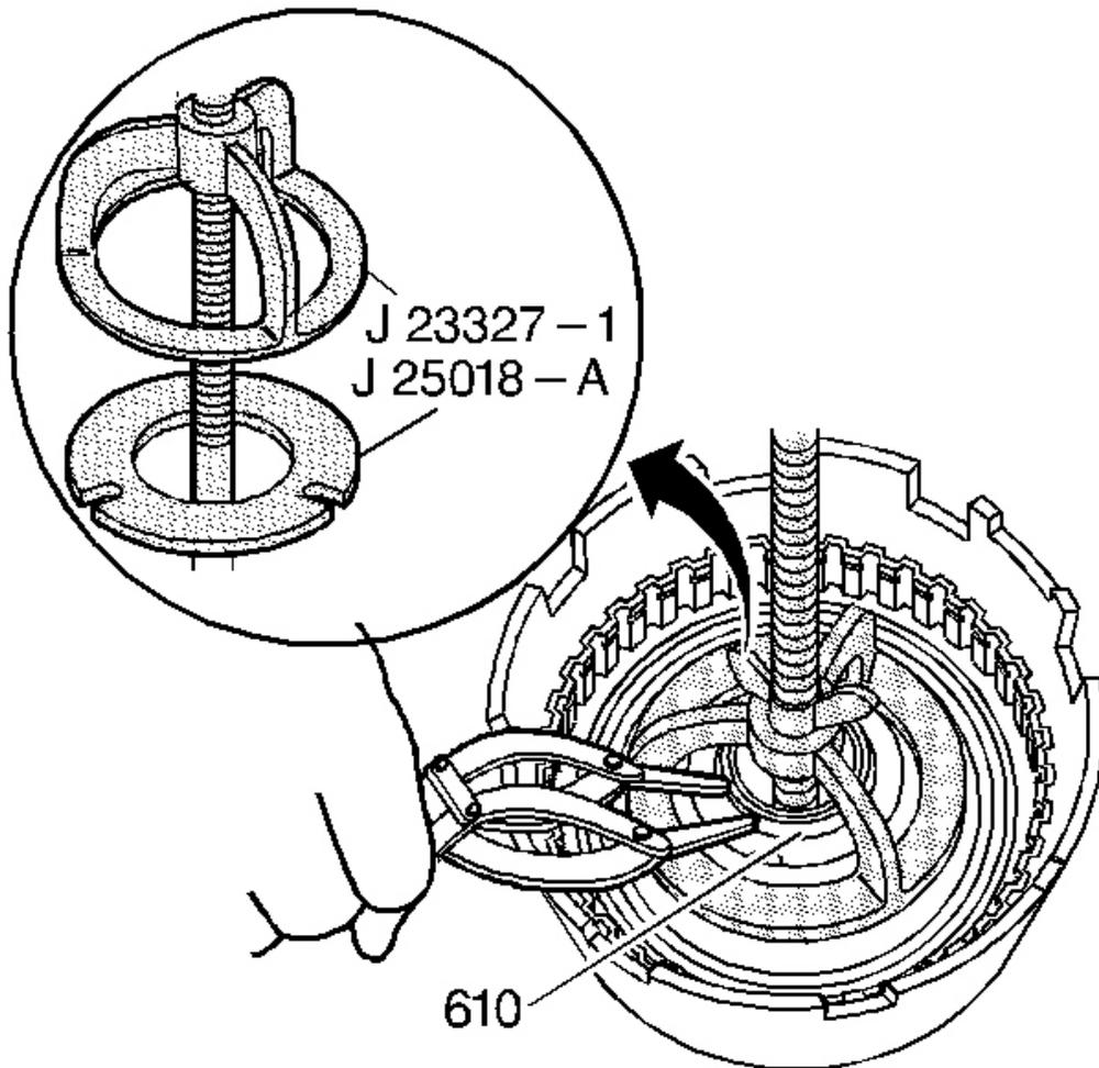
**Fig. 198: View Of Reverse Input Clutch Spring Retainer Ring**
