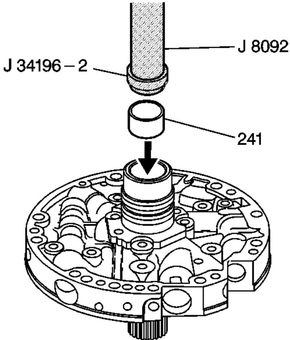
**Fig. 231: Installing Stator Shaft Rear Bushing**
