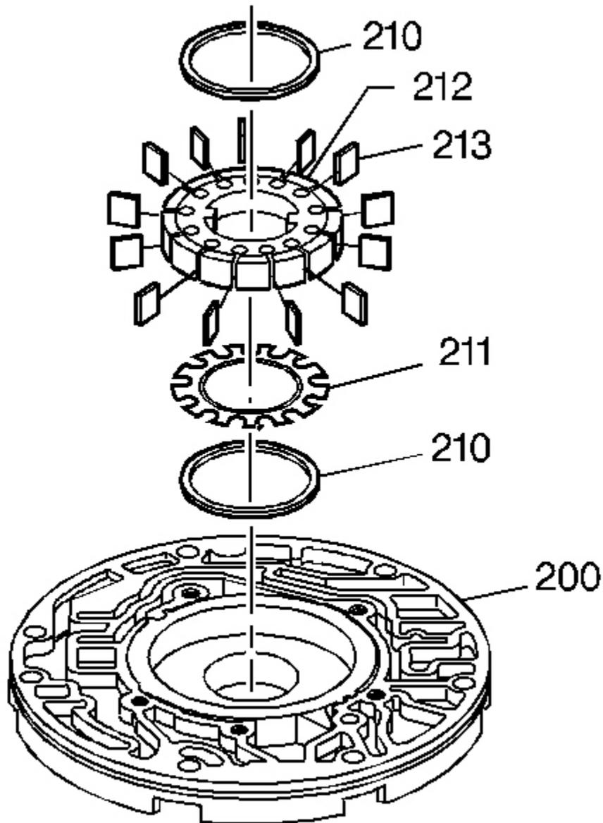
**Fig. 221: Identifying Pump Vane Ring Assemblies**
