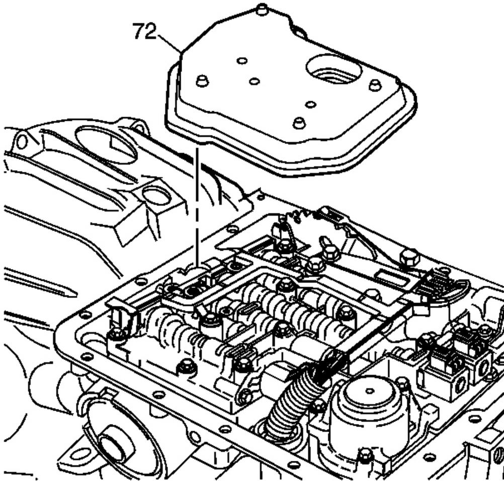
**Fig. 37: Identifying Transmission Oil Filter Assembly**
