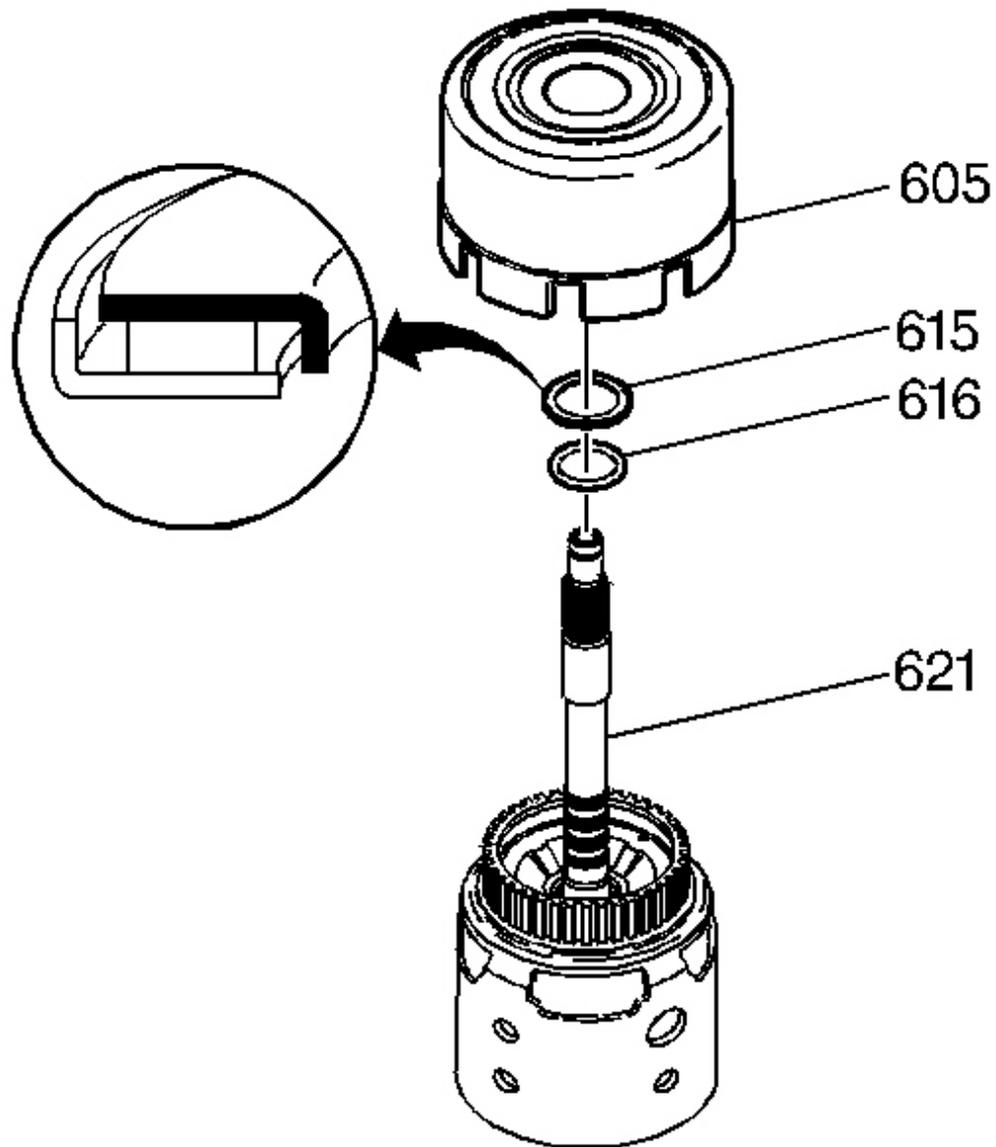
**Fig. 202: Locating Selective Thrust Washer**
