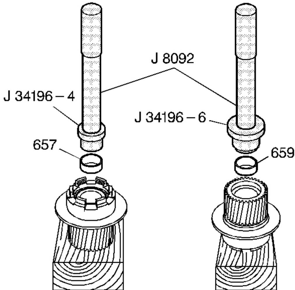
**Fig. 140: Installing Input Sun Gear Front Bushing**
