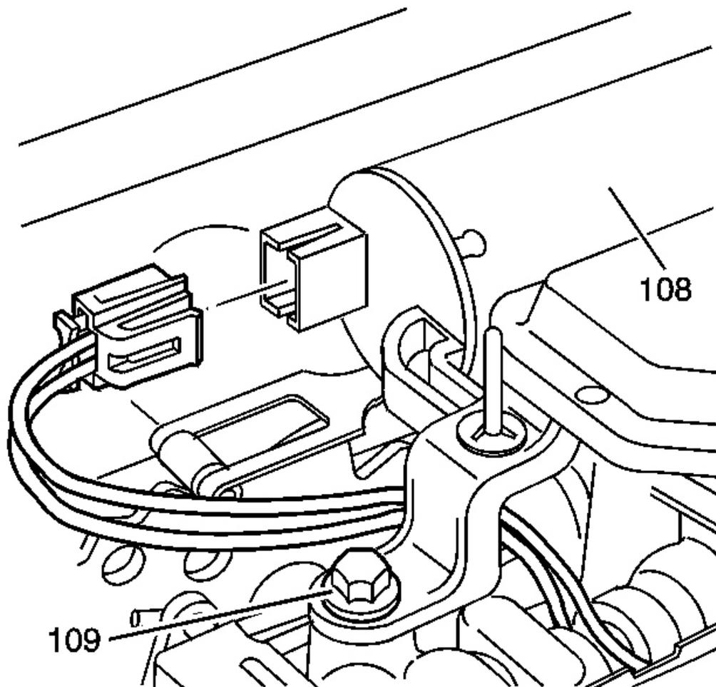
**Fig. 295: View Of Wiring Harness Connector For Secondary Fluid Pump**
