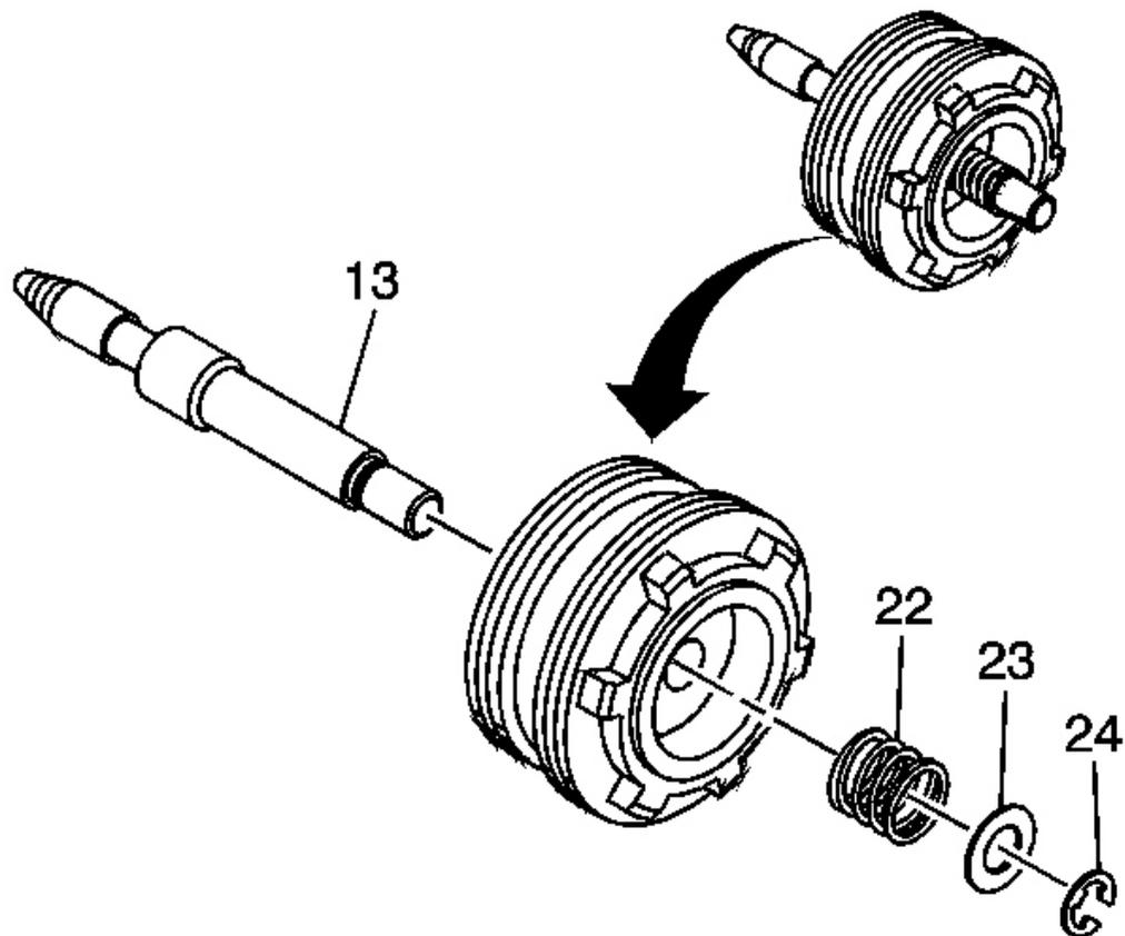
**Fig. 30: 2-4 Servo Assembly**
