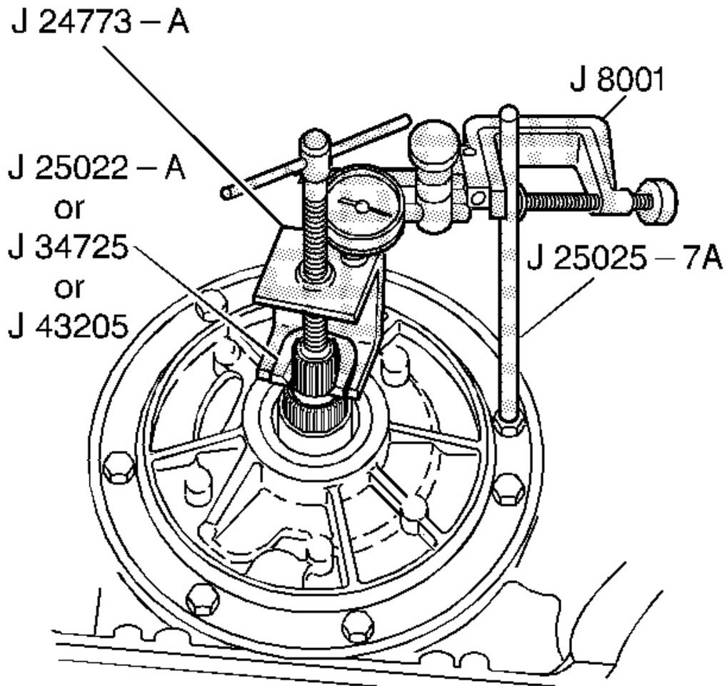
**Fig. 58: Installing J 25025-7A With J 8001**
