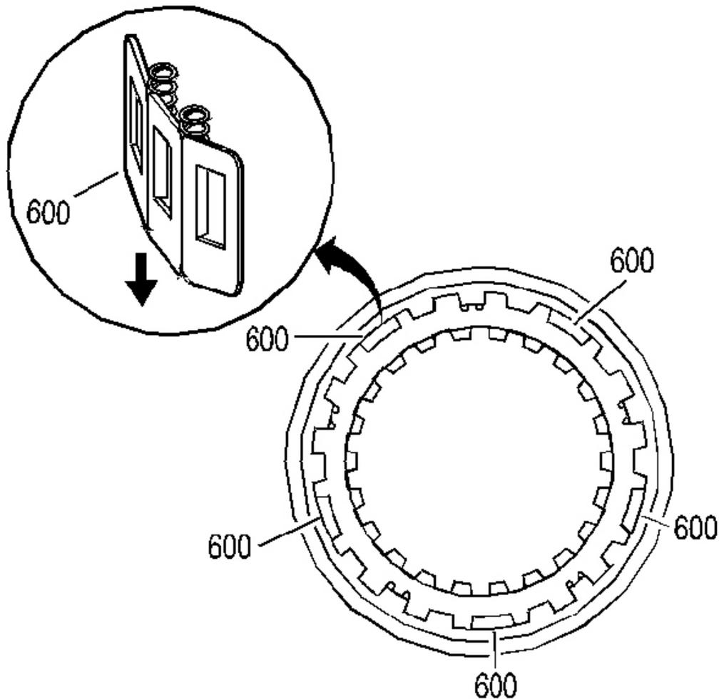
**Fig. 182: Identifying 3-4 Clutch Boost Spring Assemblies**
