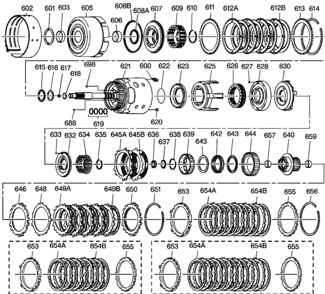
**Fig. 8: Internal Parts Disassembled View (1 Of 2)**
