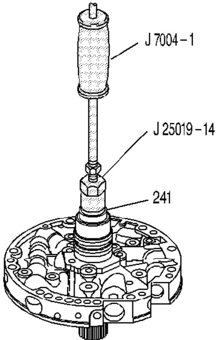
**Fig. 229: Removing Stator Shaft Rear Bushing**
