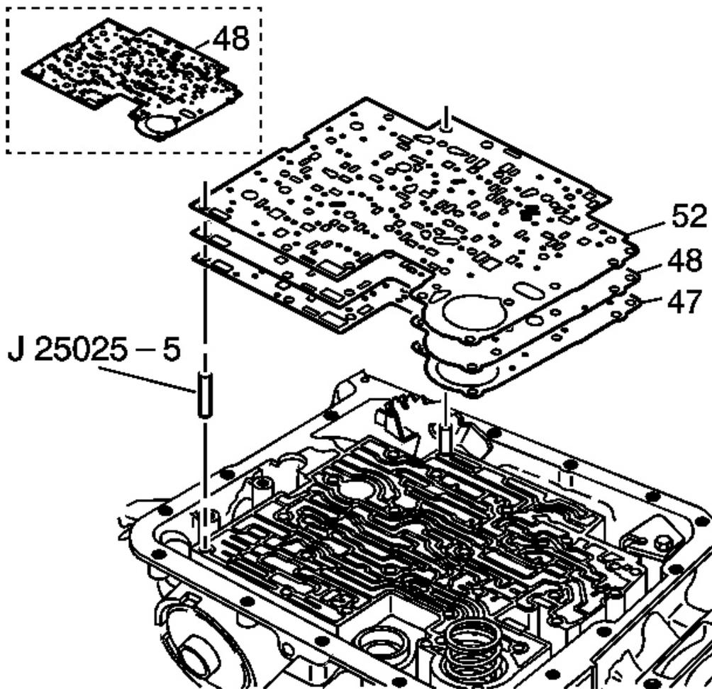
**Fig. 280: Using J 25025-5 To Install Spacer Plate**
