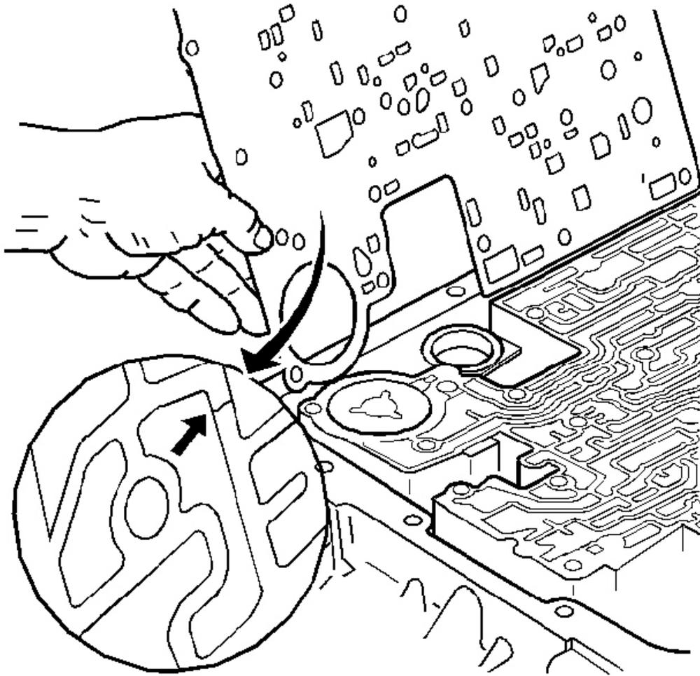
**Fig. 85: Inspecting Spacer Plate To Case Gasket For Witness Marks**
