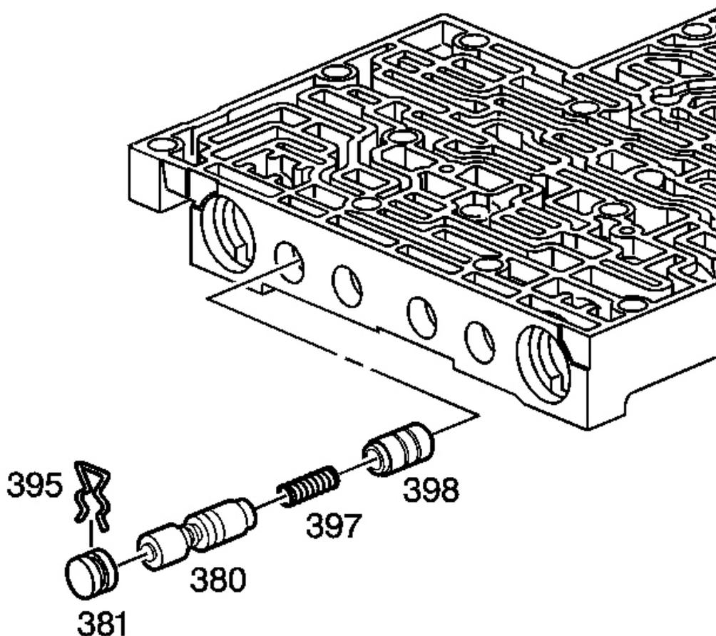
**Fig. 261: Identifying Isolator Valve & Regulator Apply Valve**
