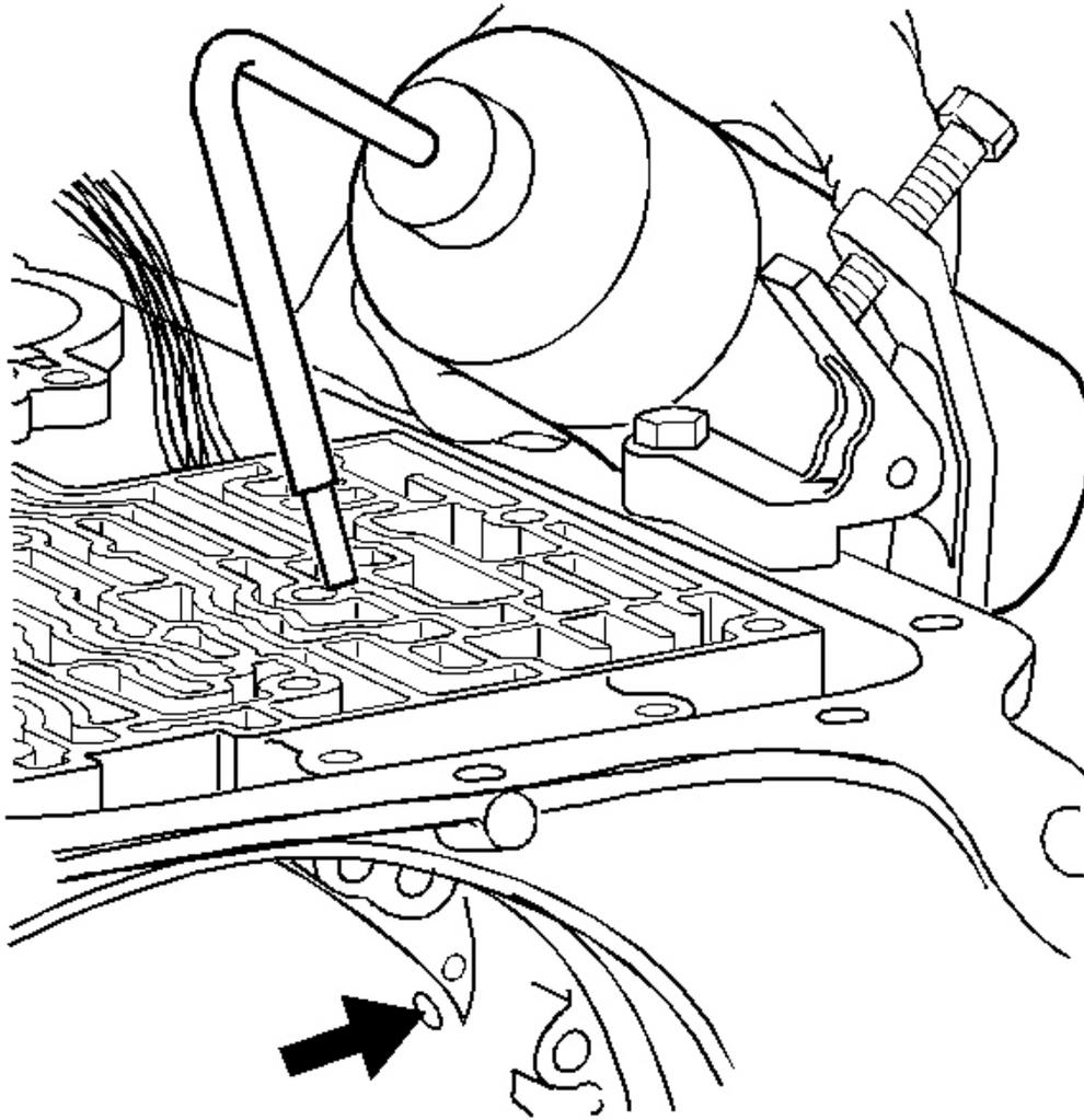
**Fig. 91: Locating Small Hole In Accumulator**
