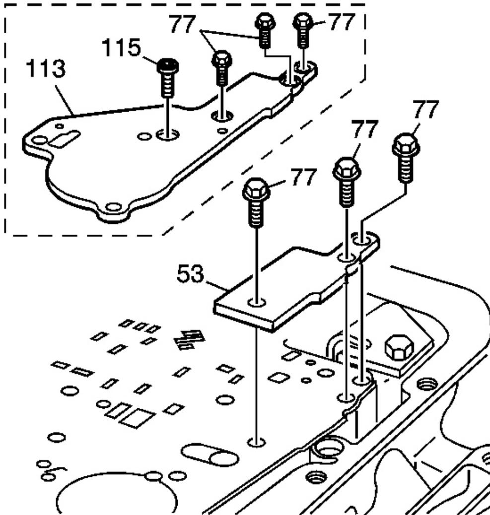
**Fig. 281: View Of Spacer Plate Support Plate & Bolts**
