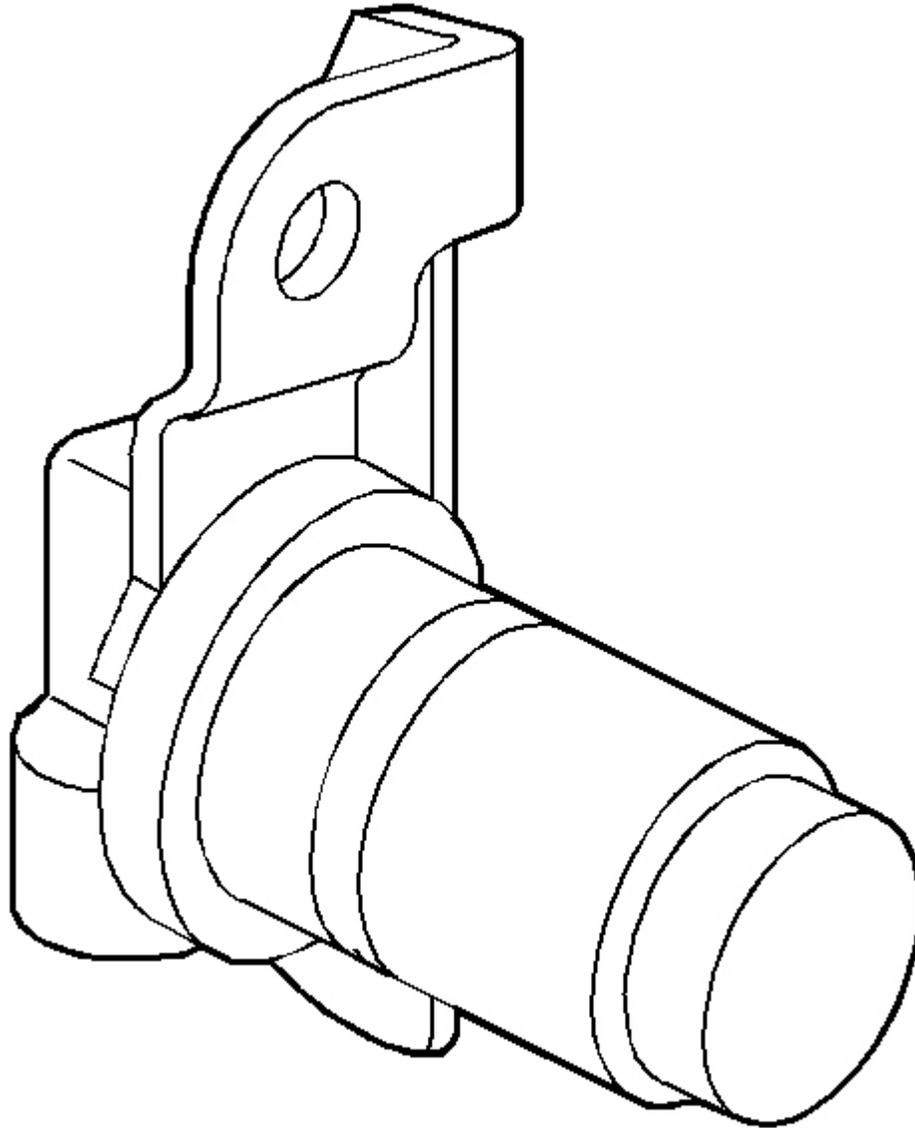
**Fig. 316: Identifying Transmission Speed Sensor**
