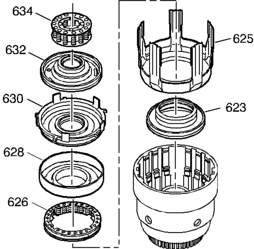
**Fig. 150: Input Clutch Assembly**
