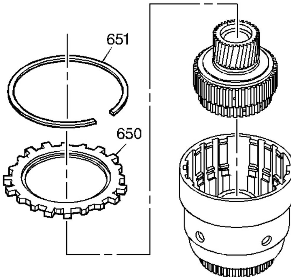
**Fig. 147: Identifying Forward Clutch Selective Backing Plate & Retainer Ring**
