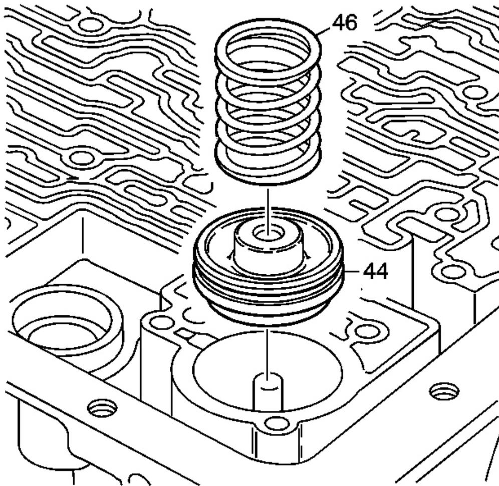
**Fig. 273: View Of 3-4 Accumulator Piston & Seal Assembly**
