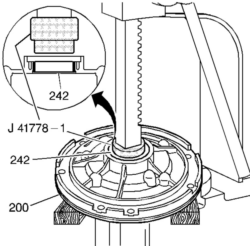
**Fig. 214: Removing Pump Body Bushing**
