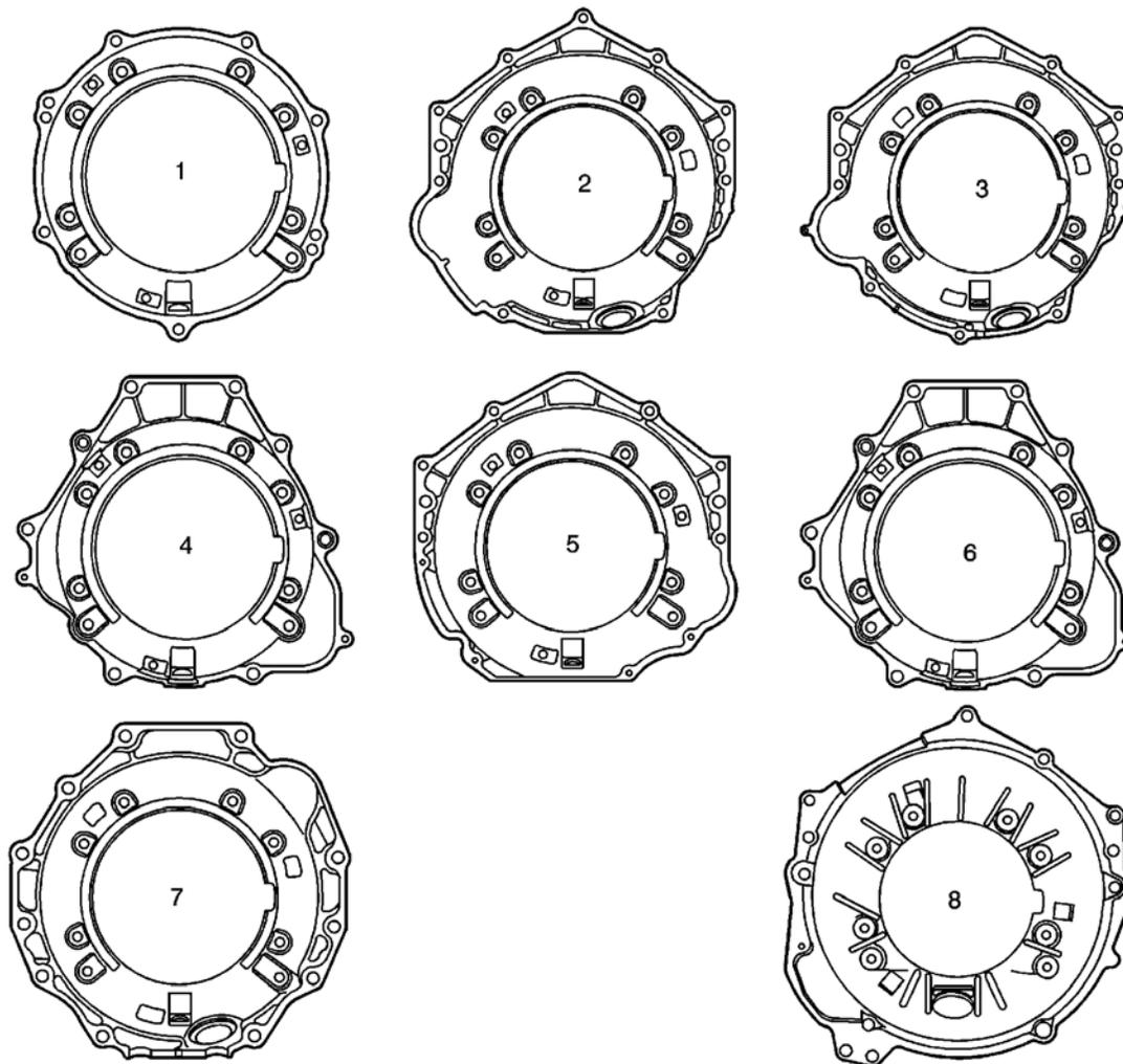
**Fig. 19: Torque Converter Housing Identification**
