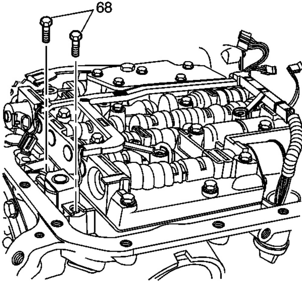
**Fig. 43: Identifying TCC Solenoid Valve Mounting Bolts**
