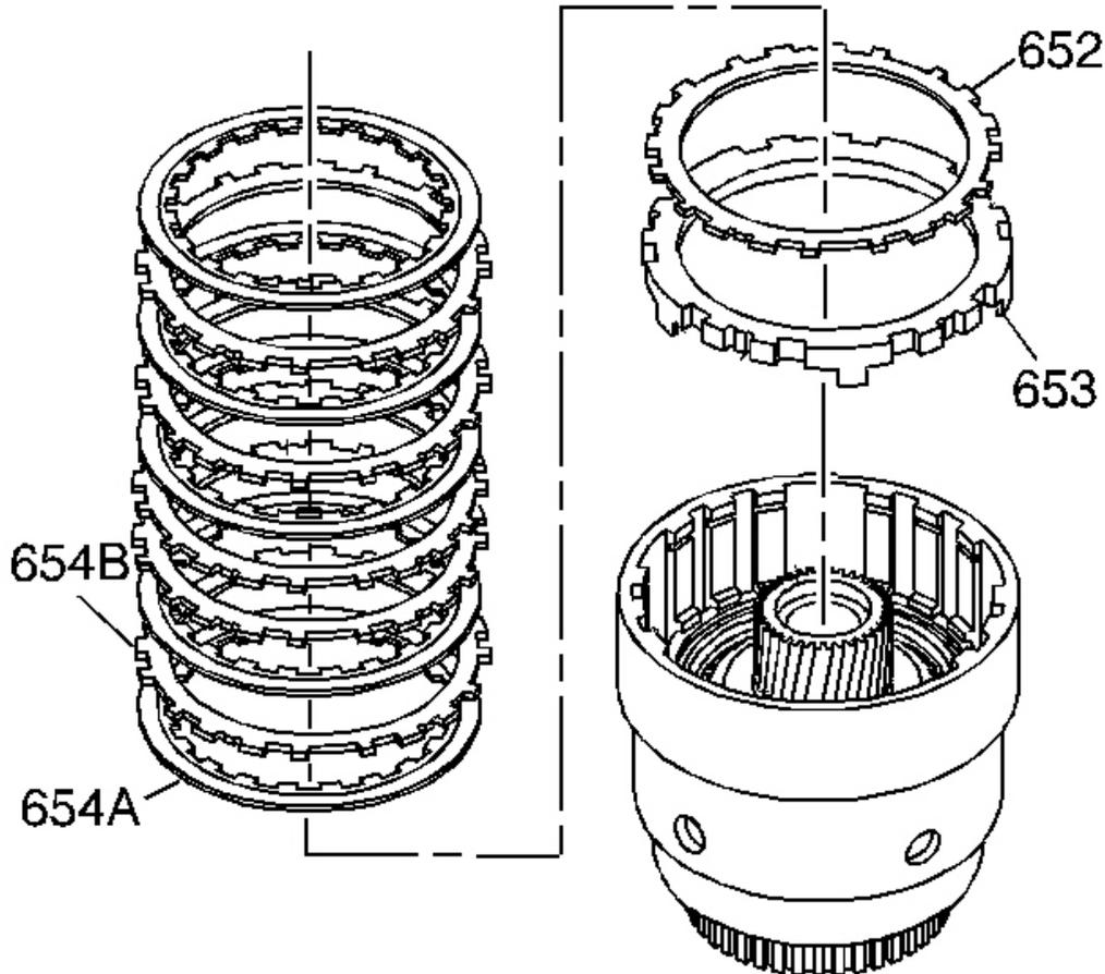
**Fig. 181: Illustrating Clutch Plate Assembly**
