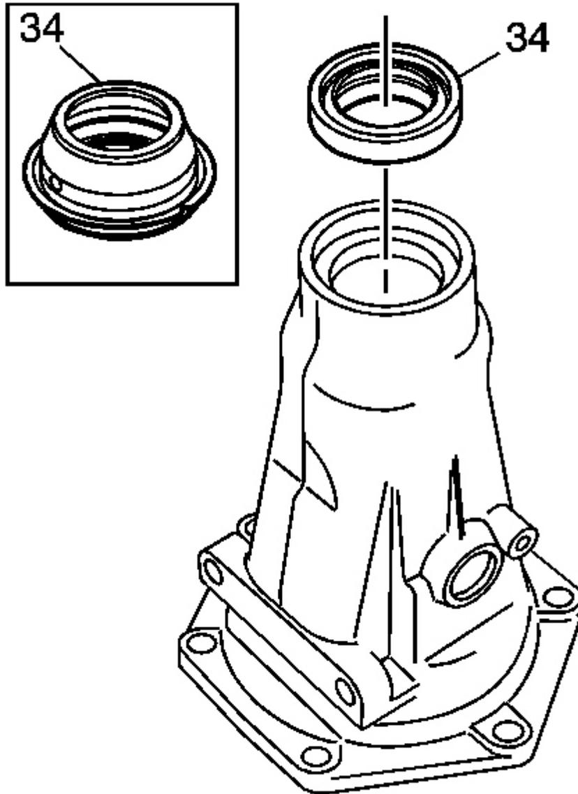
**Fig. 311: View Of Case Extension Oil Seal Assembly**
