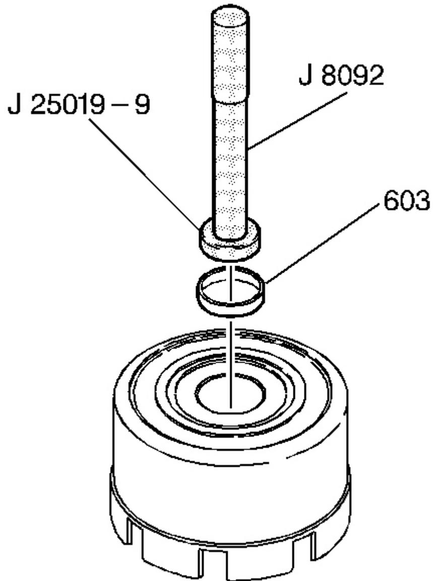
**Fig. 193: View Of Reverse Input Clutch Front Bushing**
