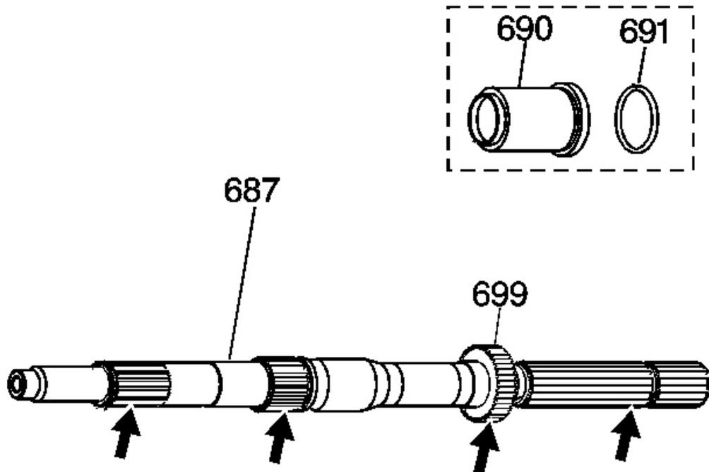
**Fig. 133: Identifying Output Shaft Seal & Output Shaft Sleeve**
