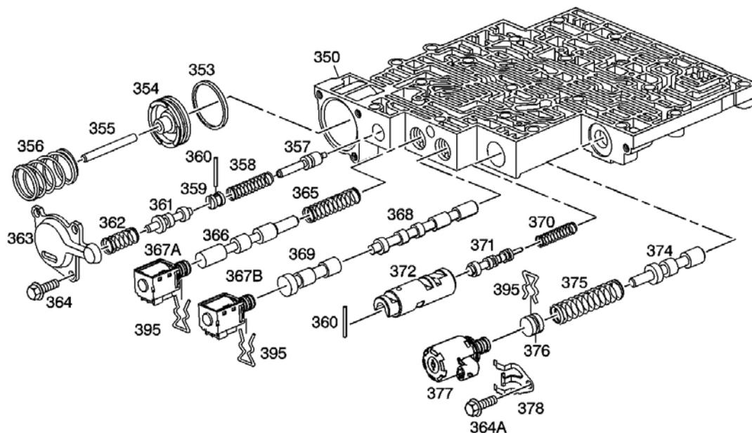
**Fig. 6: Control Valve Body Assembly Disassembled View (1 Of 2)**
