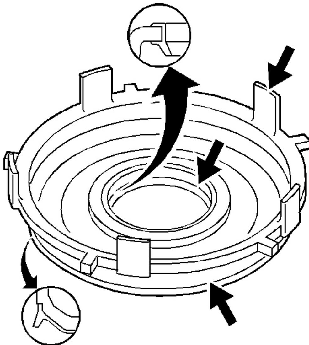
**Fig. 156: Inspecting Forward Clutch Piston For Damage Or Wear**
