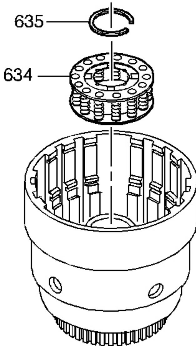
**Fig. 163: View Of Overrun Clutch Spring Assembly**
