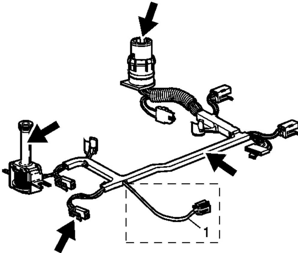
**Fig. 283: Locating Wiring Harness And Solenoid Assembly Inspection Areas**
