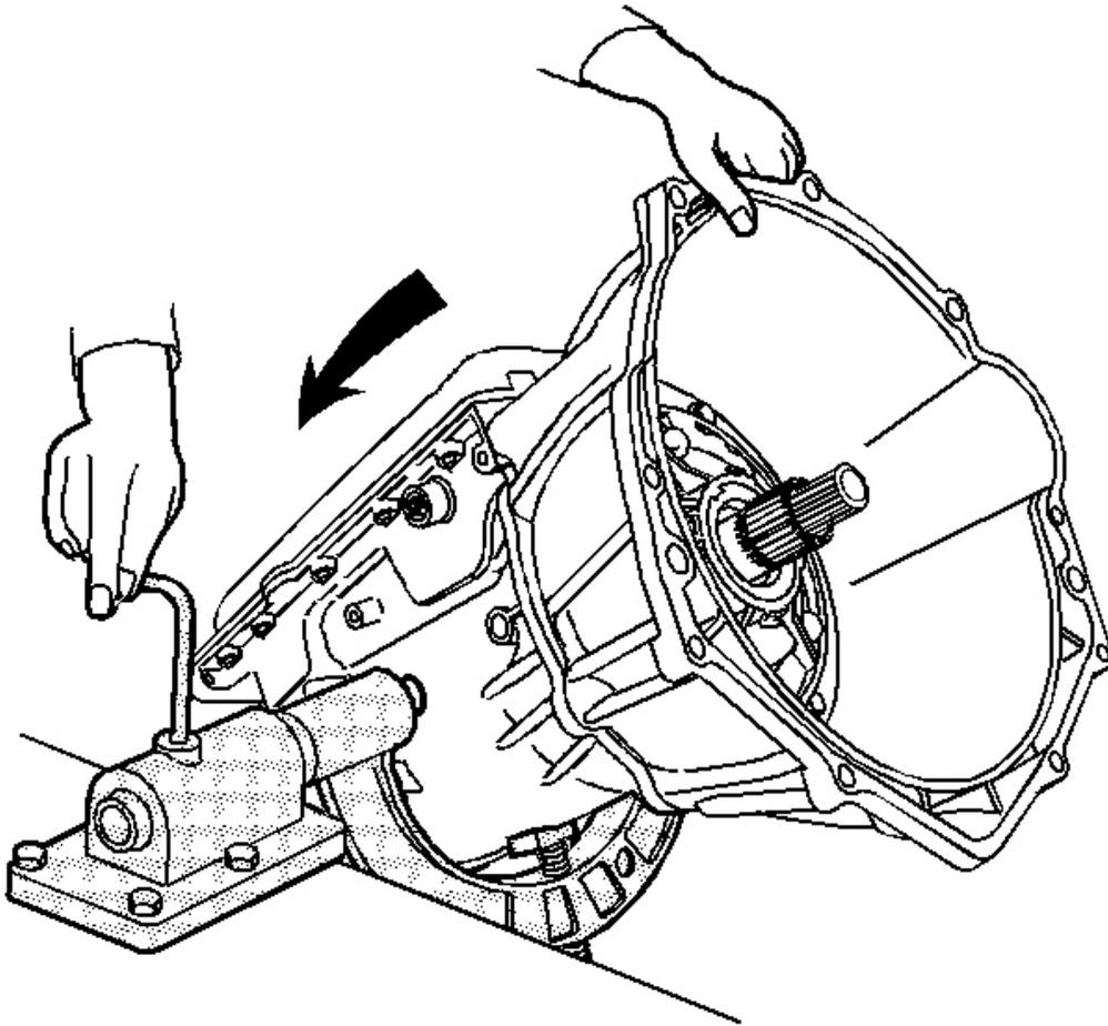
**Fig. 24: Draining Transmission Oil**
