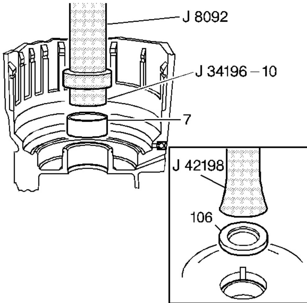
**Fig. 98: View Of Case Bushing & Case Rear Oil Seal**
