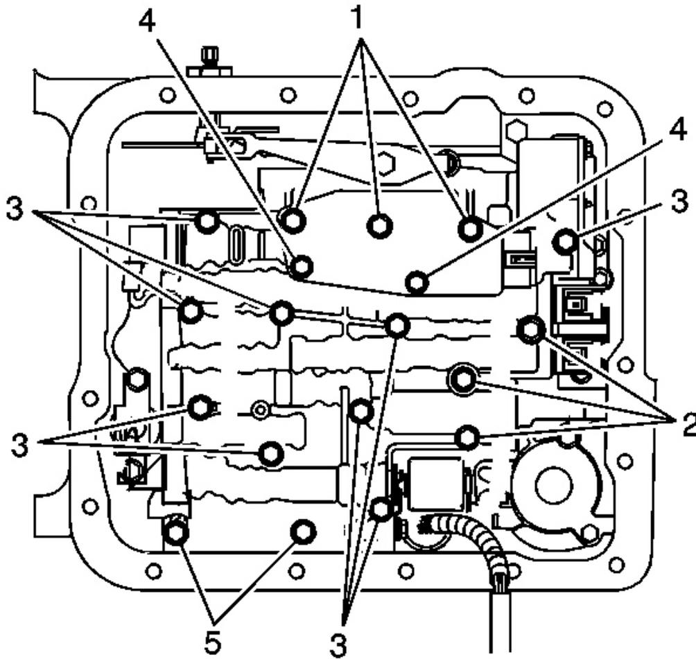
**Fig. 290: Locating Valve Body Bolts**
