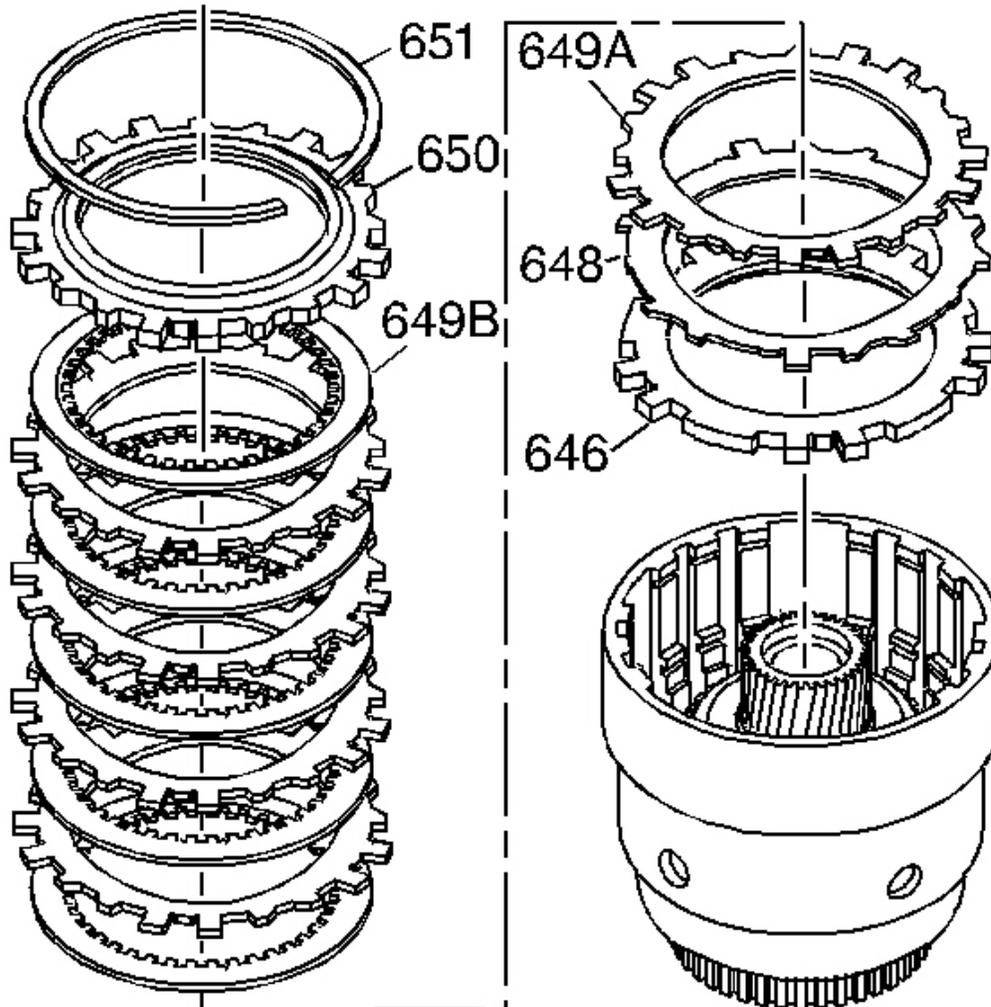
**Fig. 177: Identifying Forward Clutch Apply Plates**
