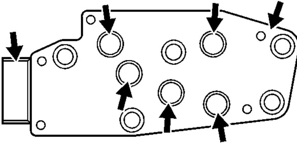
**Fig. 287: Inspection Areas On Transmission Fluid Pressure (TFP) Manual Valve Position Switch Assembly**
