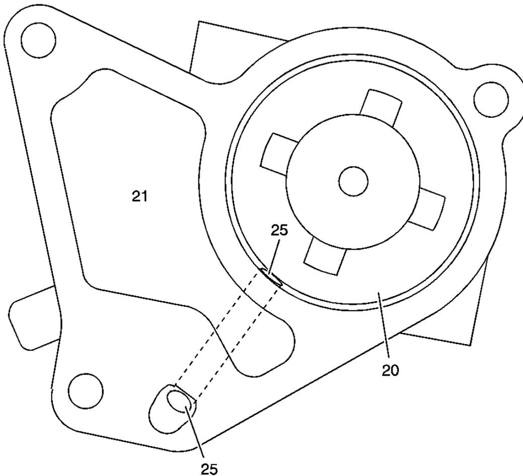
**Fig. 346: 1-2 Accumulator Cover Fluid Passages**
