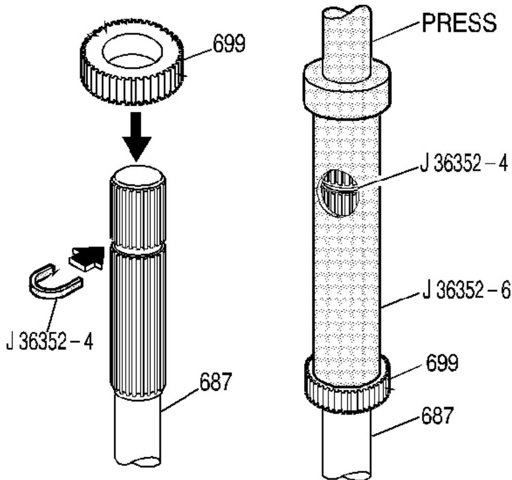
**Fig. 135: Pressing Internal Speed Sensor Rotor Onto Output Shaft**
