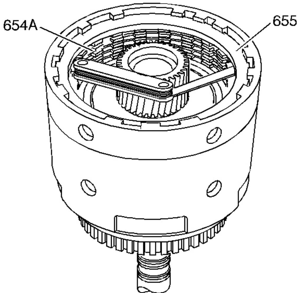
**Fig. 184: Checking 3rd & 4th Clutch Plate Travel**
