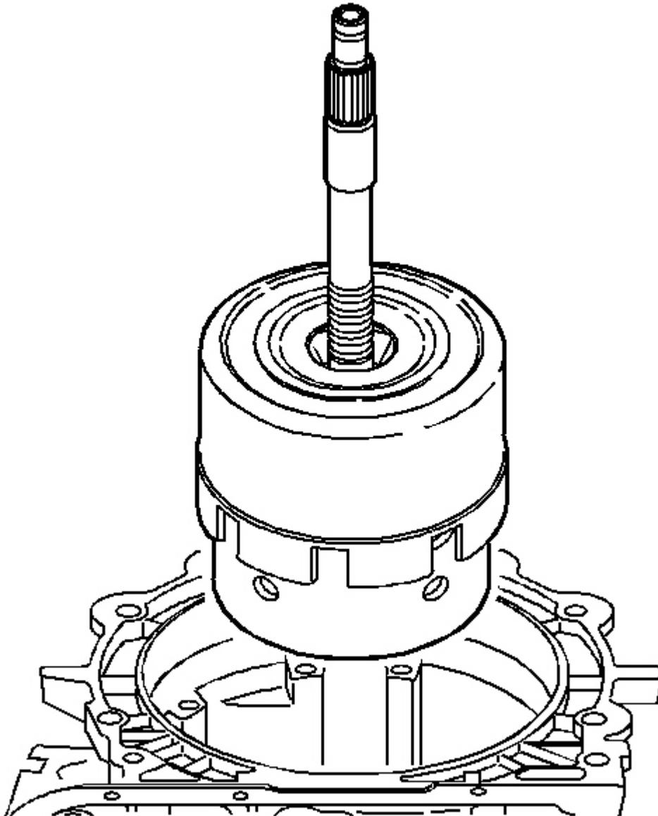
**Fig. 203: Identifying Reverse Input & Input Clutch Assembly**
