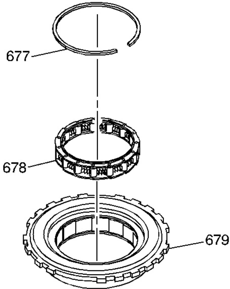
**Fig. 117: Identifying Low And Reverse Roller Clutch Assembly**
