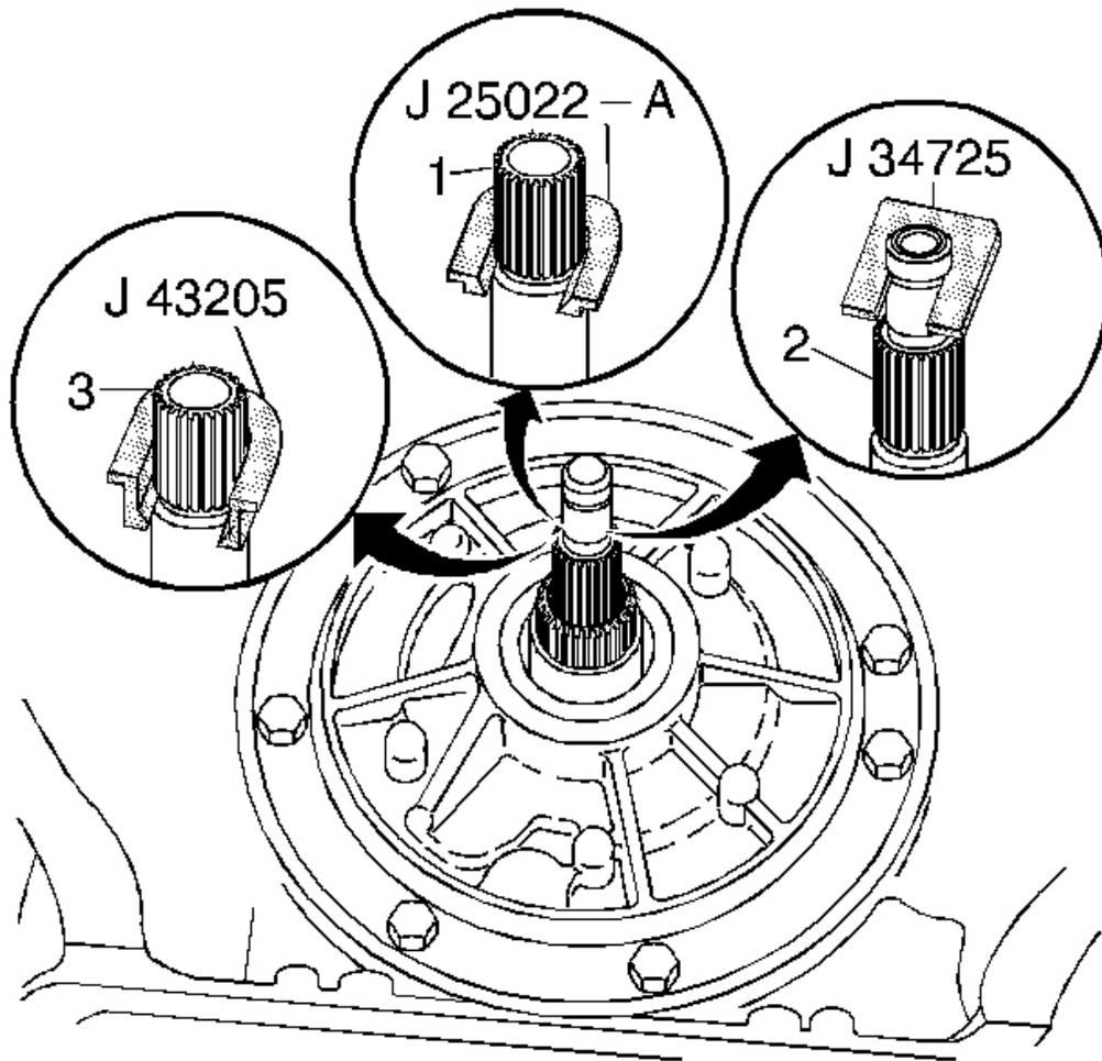
**Fig. 56: Identifying Different End Play Fixture Adapters**
