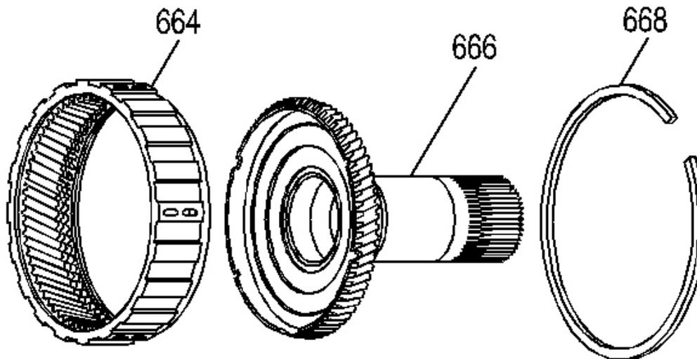
**Fig. 127: Identifying Reaction Carrier Components**
