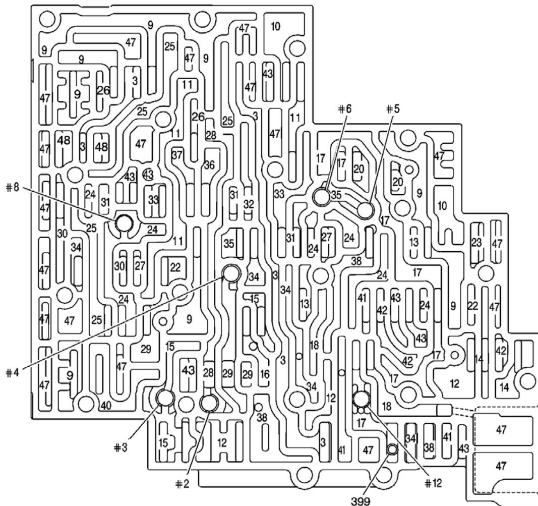
**Fig. 343: Control Valve Body Fluid Passages (Case Side)**
