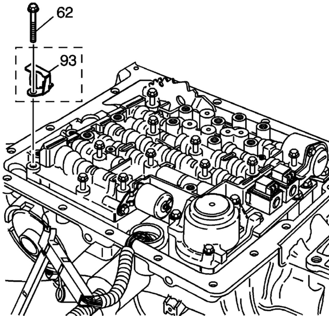
**Fig. 47: Locating Valve Body Bolts & Fluid Level Indicator Stop Bracket**
