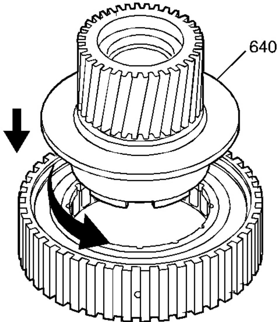
**Fig. 173: Inspection Areas On Forward Sprag Clutch Inner Race And Input Sun Gear Assembly**
