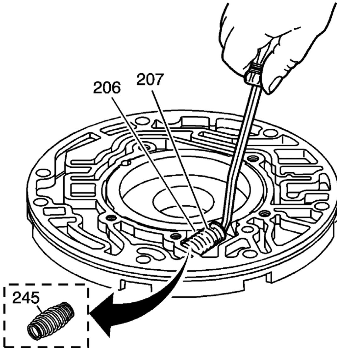
**Fig. 220: View Of Fluid Pump Slide Outer Spring**
