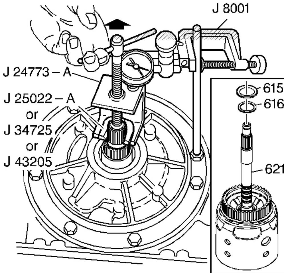
**Fig. 59: Checking End Play With J 8001**
