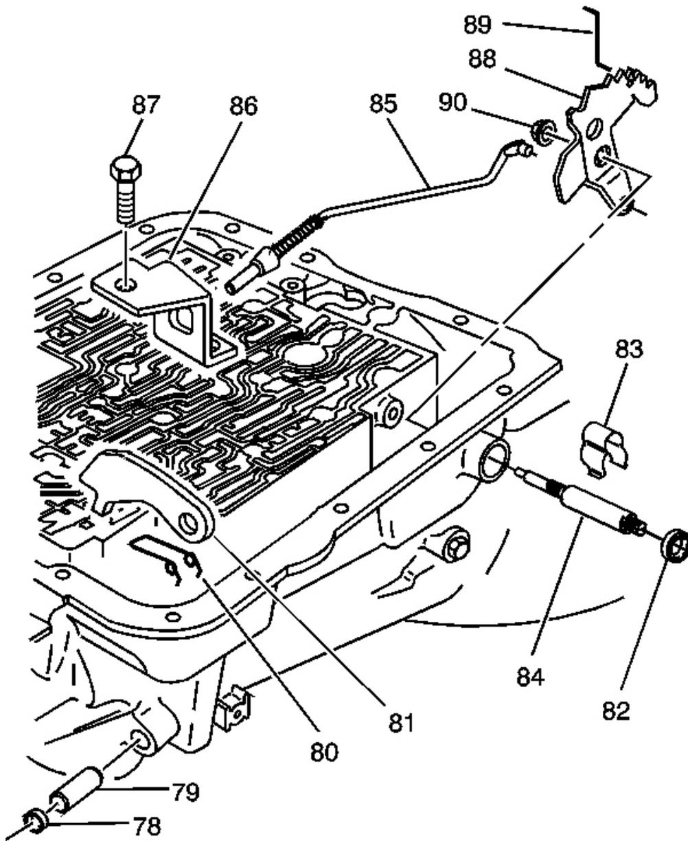
**Fig. 10: Parking Lock & Manual Shift Shaft Assembly Disassembled View**
