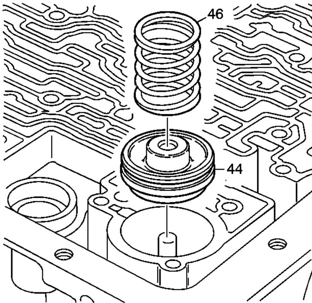
**Fig. 53: View Of 3-4 Accumulator Piston & Seal Assembly**
