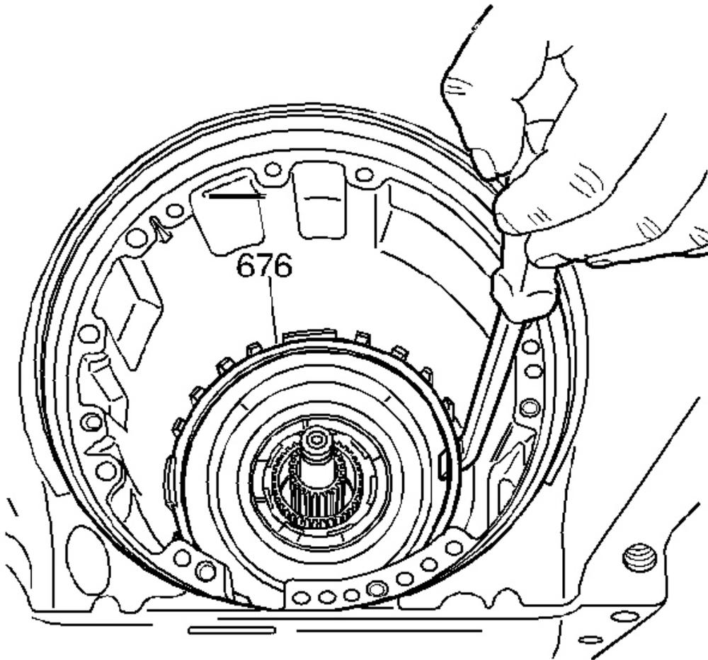
**Fig. 121: Identifying Low And Reverse Support Retainer Ring**
