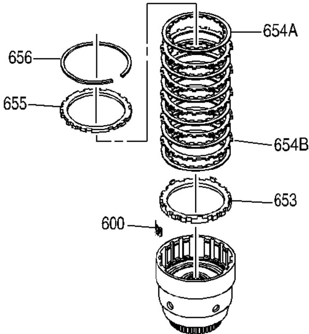
**Fig. 146: Locating 3rd & 4th Clutch Backing Plate Retainer Ring**
