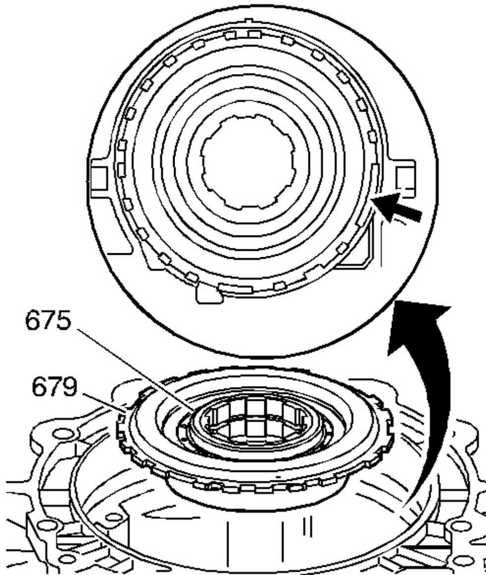
**Fig. 120: Aligning Wide Case Lug With Wide Low And Reverse Clutch Support Notch**
