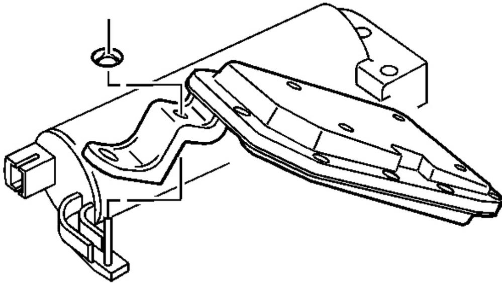
**Fig. 298: View Of Secondary Fluid Pump & Clip**
