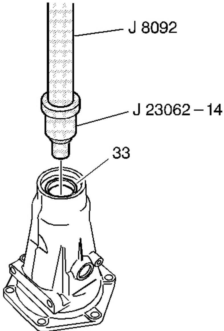
**Fig. 312: Removing Case Extension Bushing**
