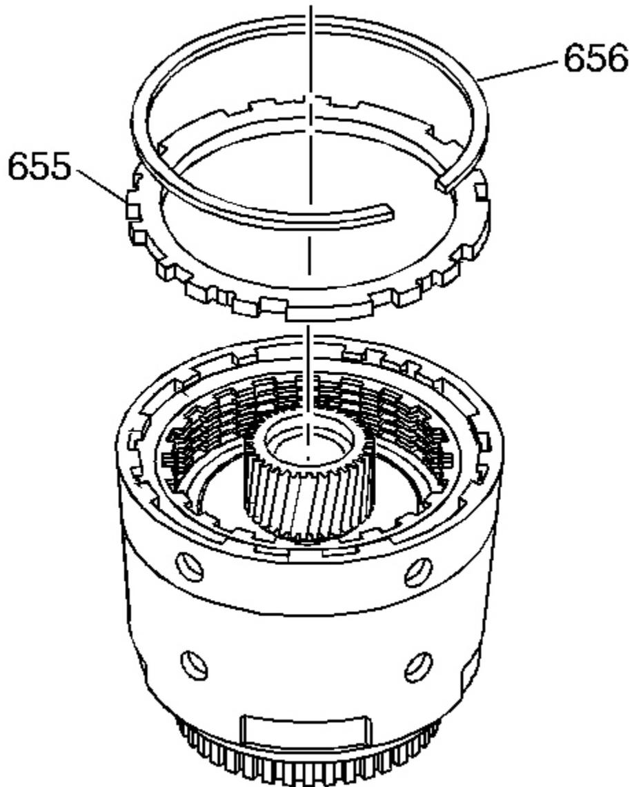
**Fig. 183: Locating 3rd & 4th Clutch Selective Backing Plate & Retainer Ring**
