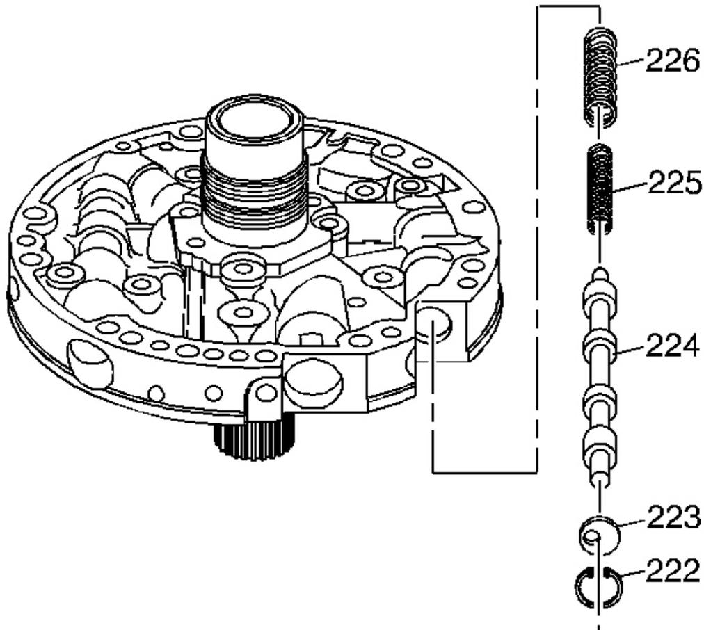
**Fig. 234: Locating Converter Clutch Valve**
