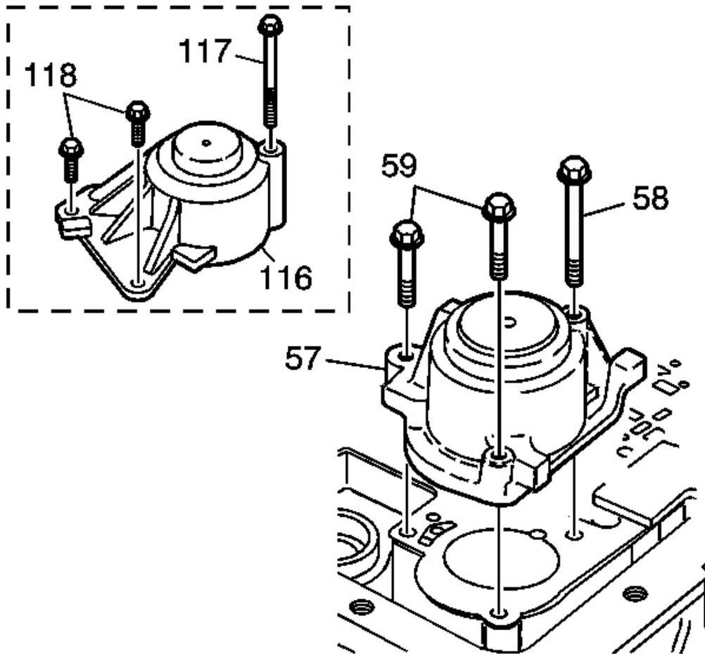
**Fig. 282: Installing 1-2 Accumulator Housing Bolts**
