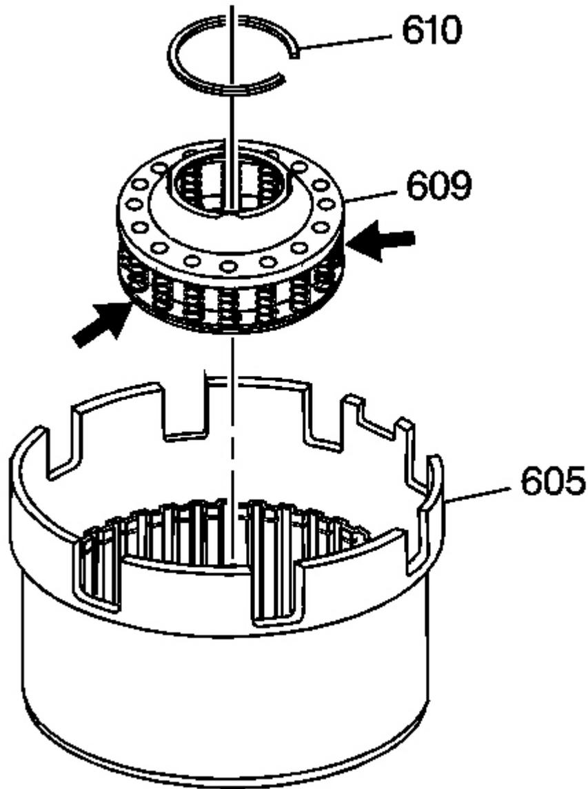
**Fig. 197: Identifying Reverse Input Clutch Spring Assembly**
