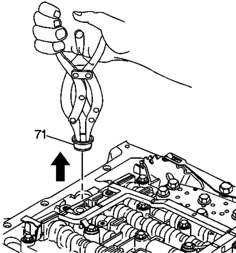
**Fig. 38: Removing Oil Filter Seal**
