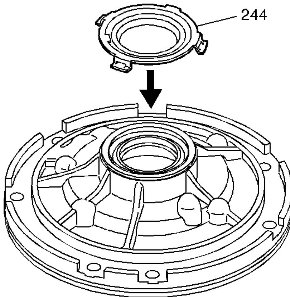
**Fig. 218: Installing Front Helix Retainer**
