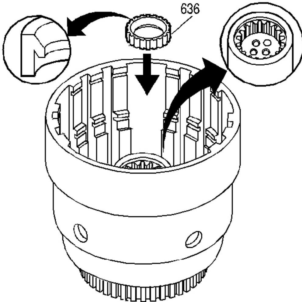
**Fig. 165: View Of Input Housing To Output Shaft Seal**
