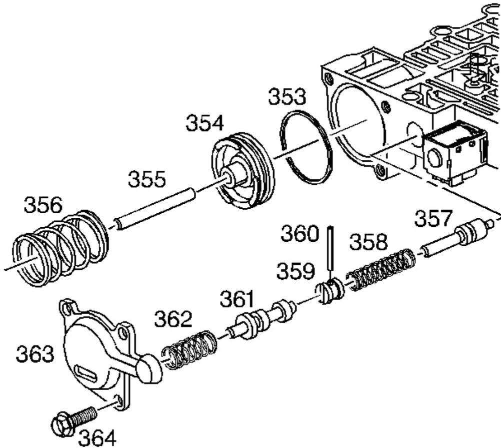
**Fig. 270: Exploded View Of Forward Abuse & Low Overrun Components**
