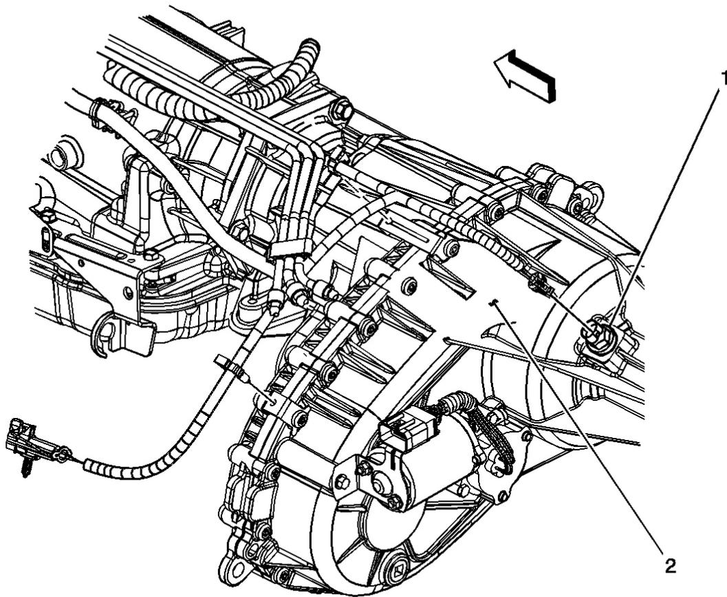
**Fig. 14: Vehicle Speed Sensor (VSS) Component View**
