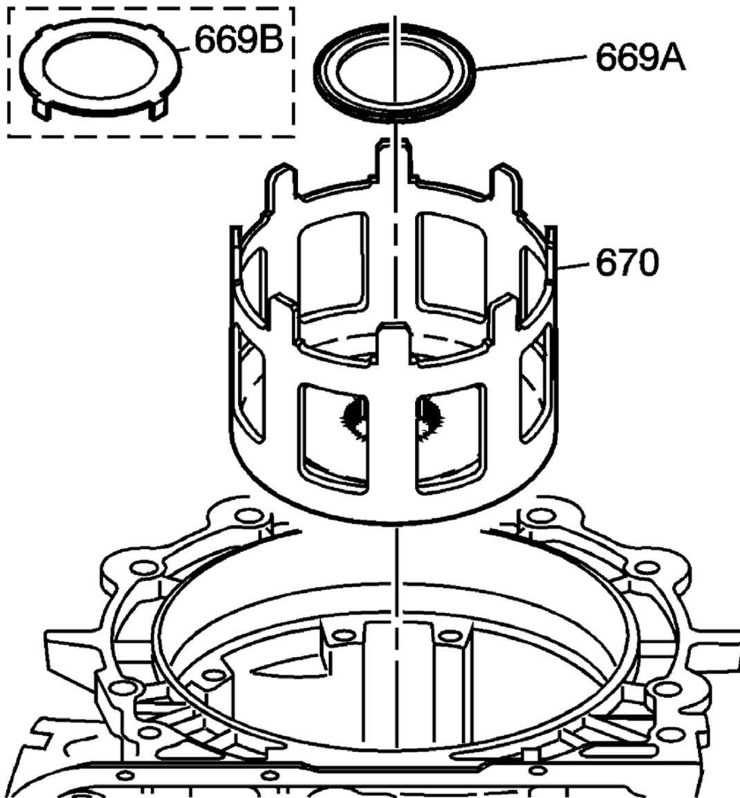
**Fig. 69: View Of Reaction Sun Shell & Thrust Washer**
