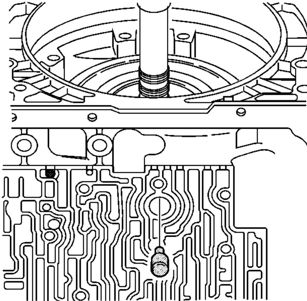
**Fig. 205: Identifying Band Anchor Pin**
