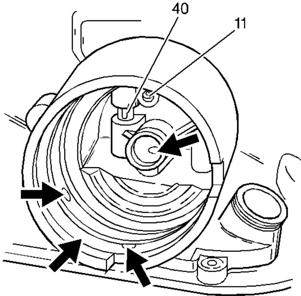
**Fig. 87: Inspecting Case Assembly Components For Damage**
