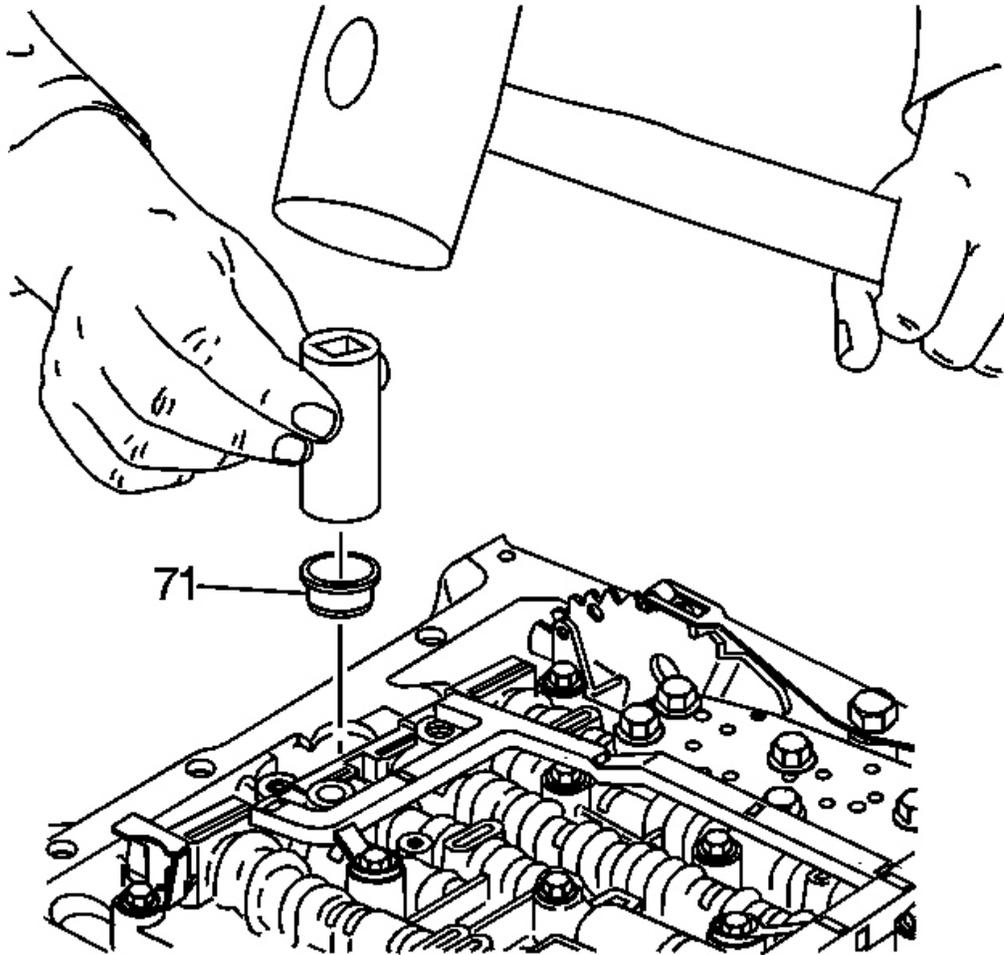
**Fig. 296: Locating Oil Filter Seal**
