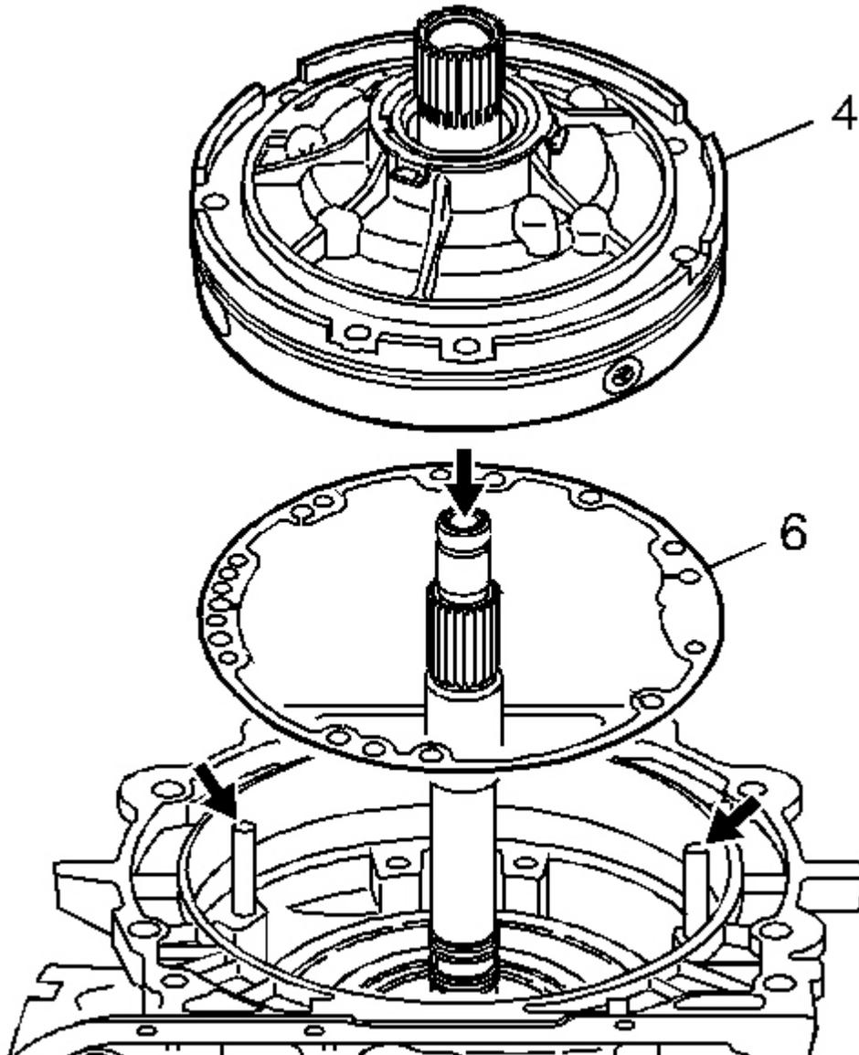
**Fig. 240: Aligning Pump Cover To Case Gasket**
