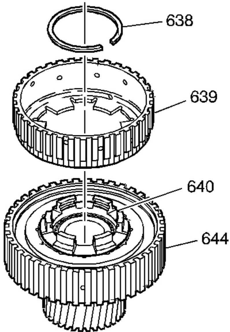
**Fig. 174: Locating Overrun Clutch Hub**
