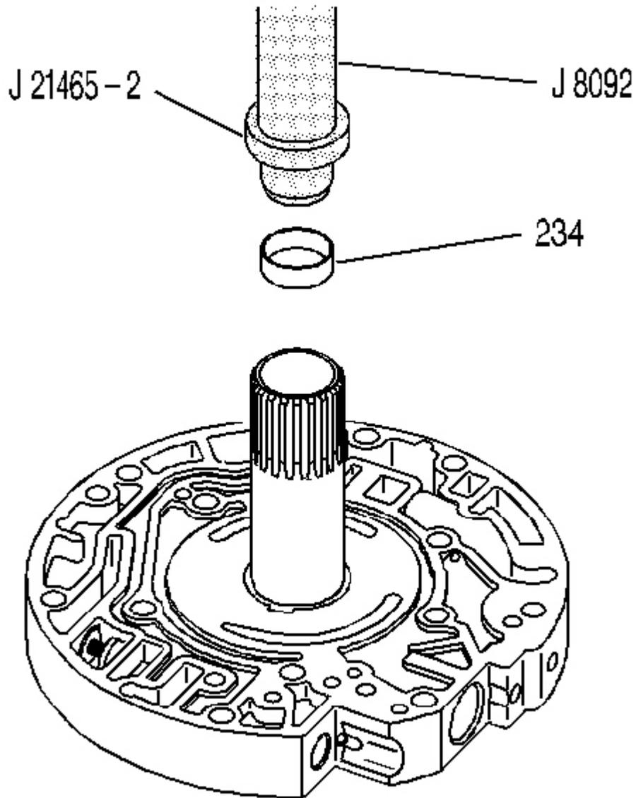
**Fig. 230: View Of Stator Shaft Front Bushing**
