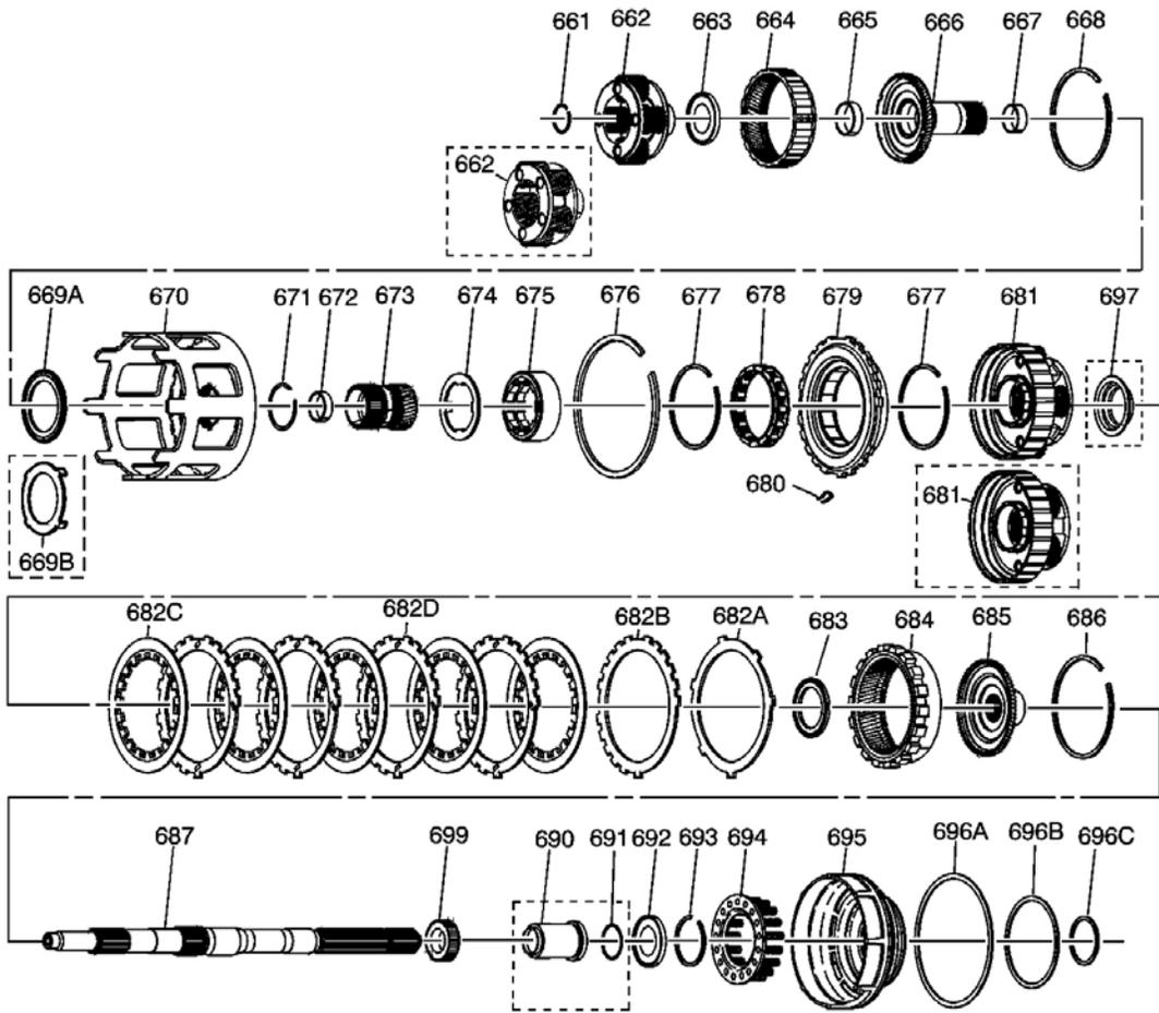
**Fig. 9: Internal Parts Disassembled View (2 Of 2)**
