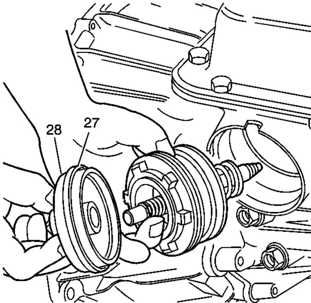
**Fig. 306: View Of 2-4 Servo Assembly**
