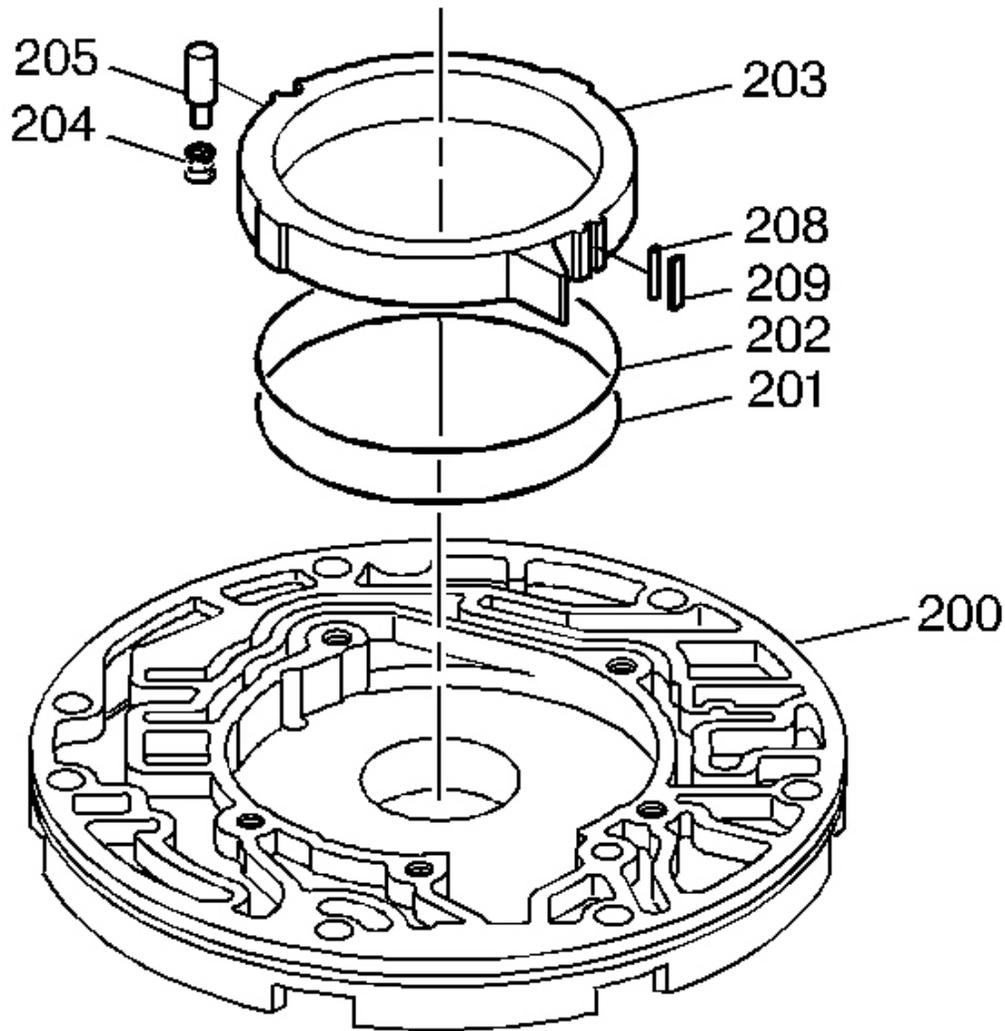
**Fig. 210: Identifying Pump Slide Components**
