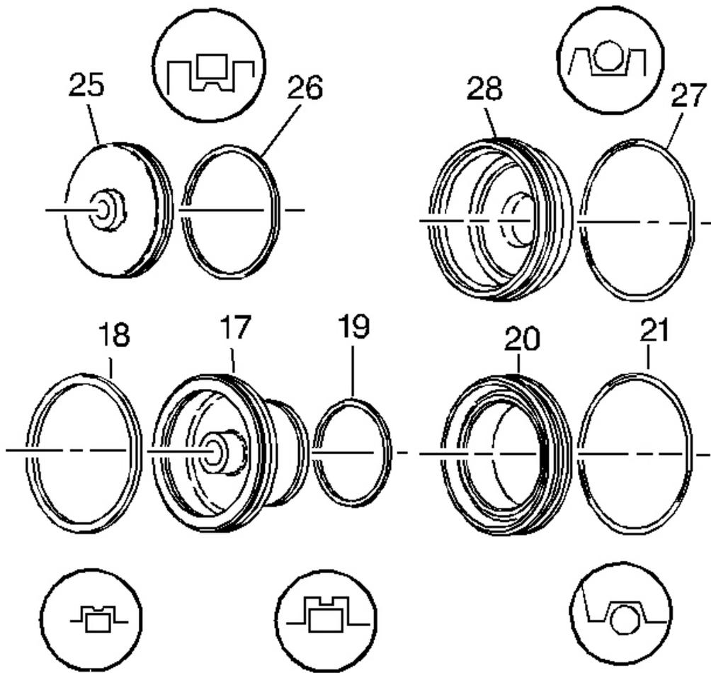
**Fig. 303: 2-4 Servo Assembly Components**
