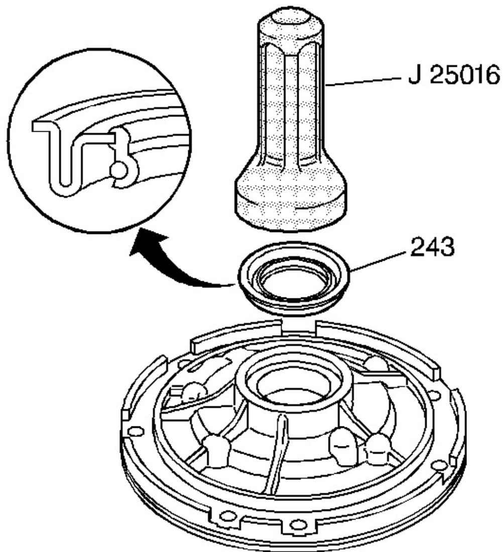
**Fig. 217: Using J 25016 To Install Oil Seal Assembly**
