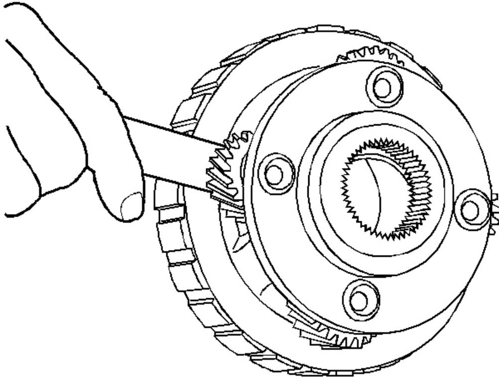
**Fig. 107: Checking Reaction Carrier Pinion End Play With Feeler Gage**
