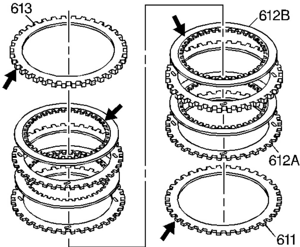
**Fig. 199: Inspecting Plates For Damage Or Wear**
