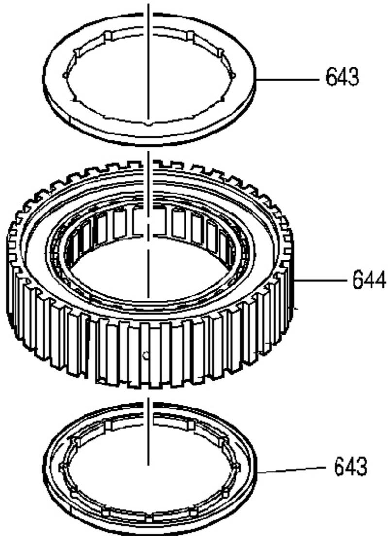
**Fig. 170: View Of Sprag Assembly Retainer Rings**
