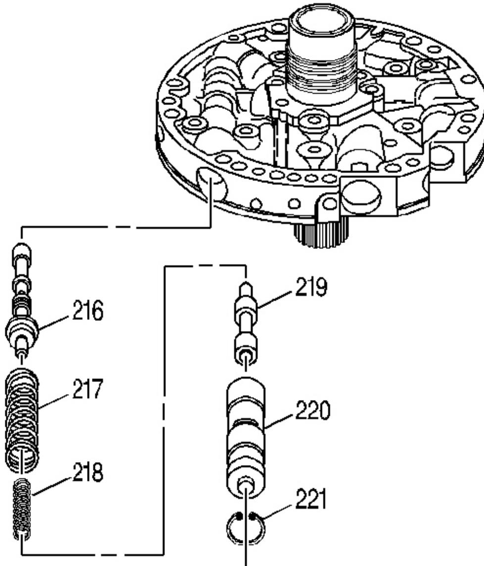
**Fig. 235: View Of Pressure Regulator Valve**
