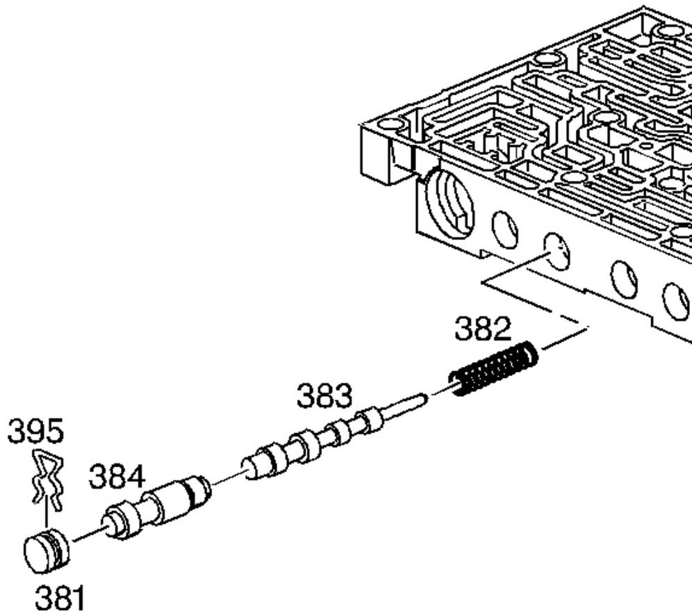
**Fig. 259: View Of 4-3 Sequence Valve & 3-4 Relay Valve**
