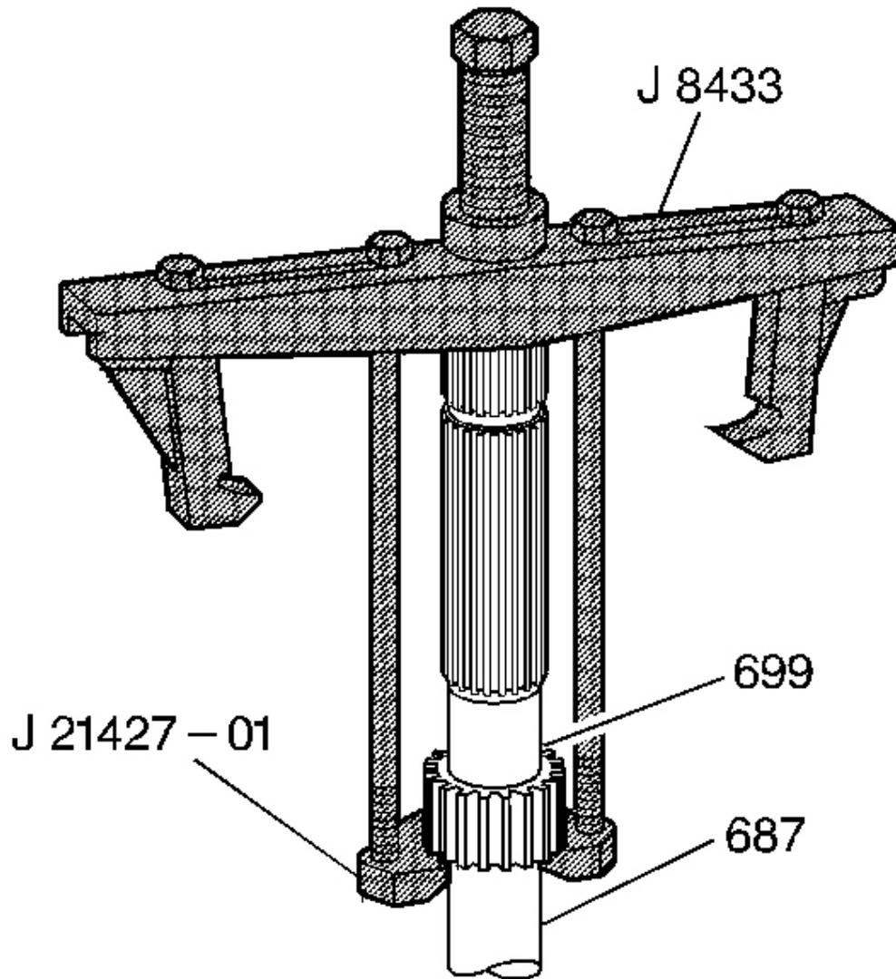
**Fig. 134: Using J 8433 & J 21427-01 To Remove Internal Speed Sensor Rotor**
