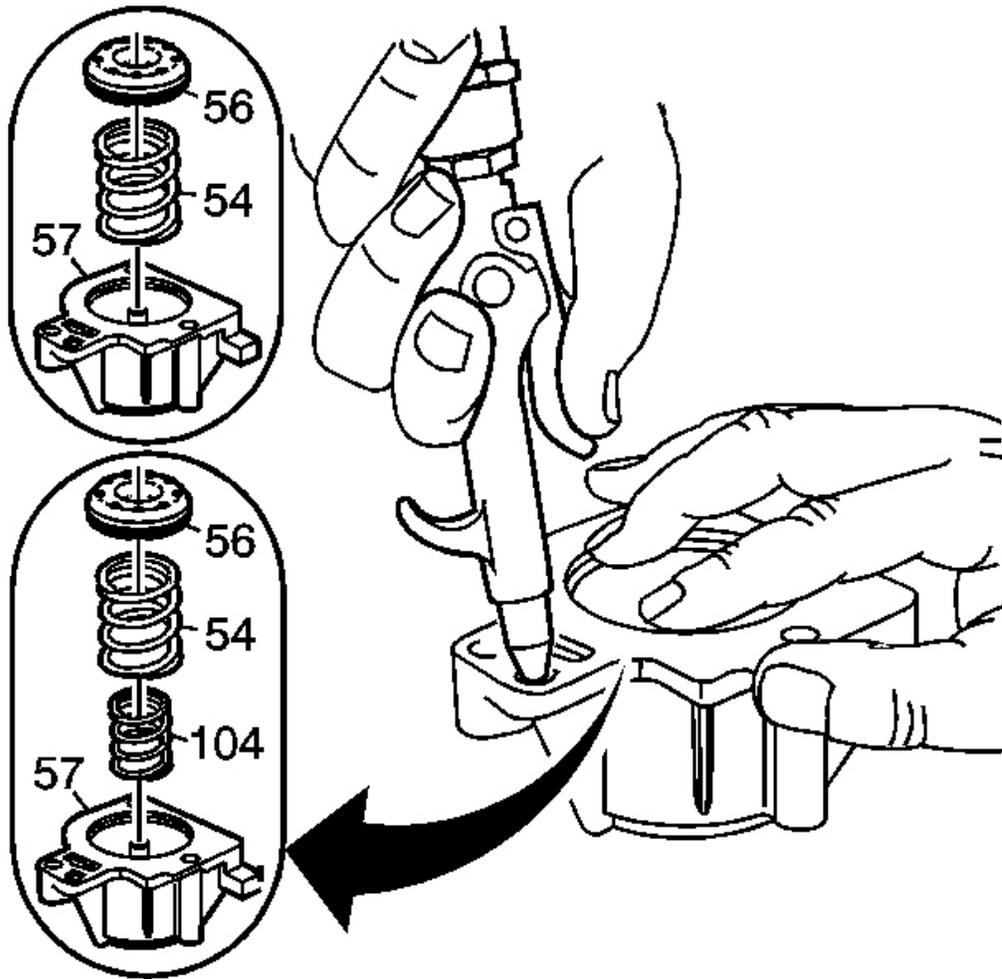
**Fig. 274: View Of 1-2 Accumulator Components**
