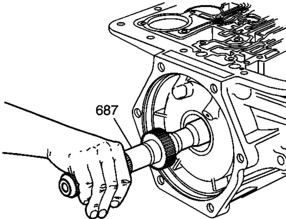
**Fig. 136: View Of Output Shaft**
