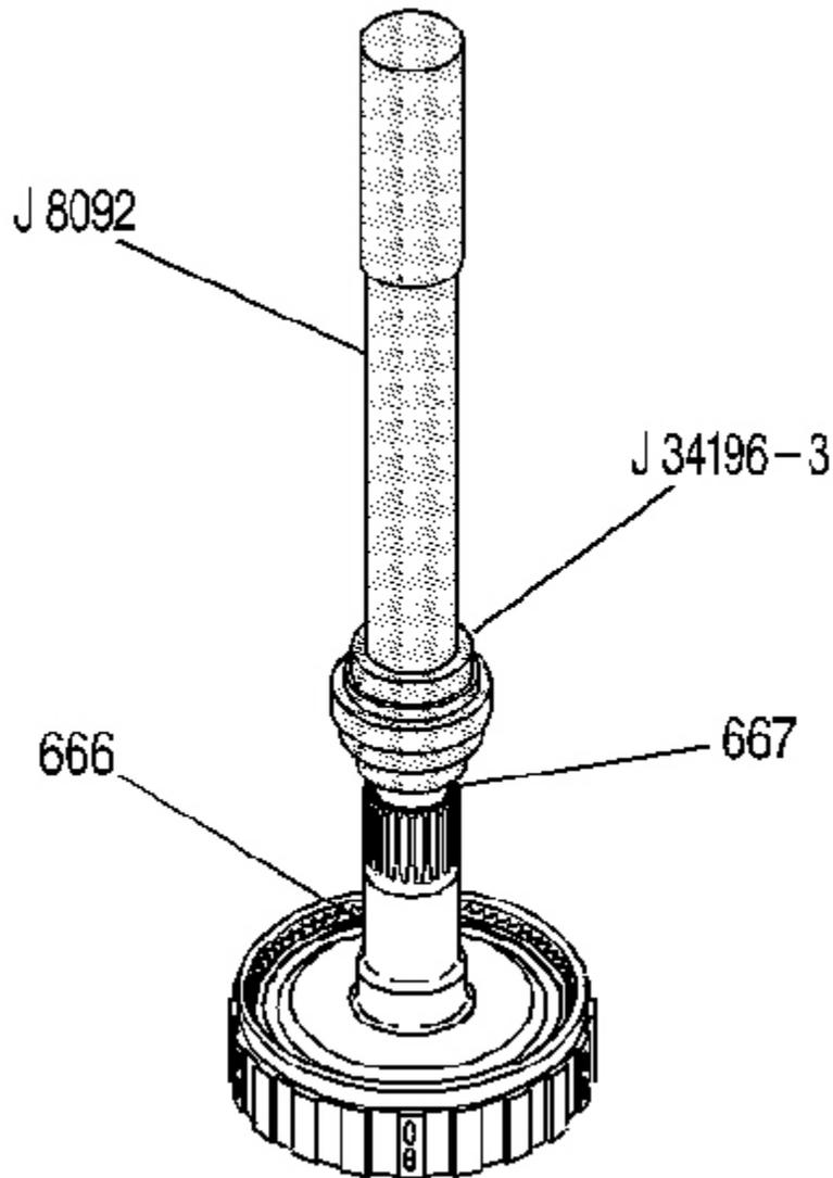
**Fig. 131: View Of Reaction Carrier Shaft Rear Bushing**
