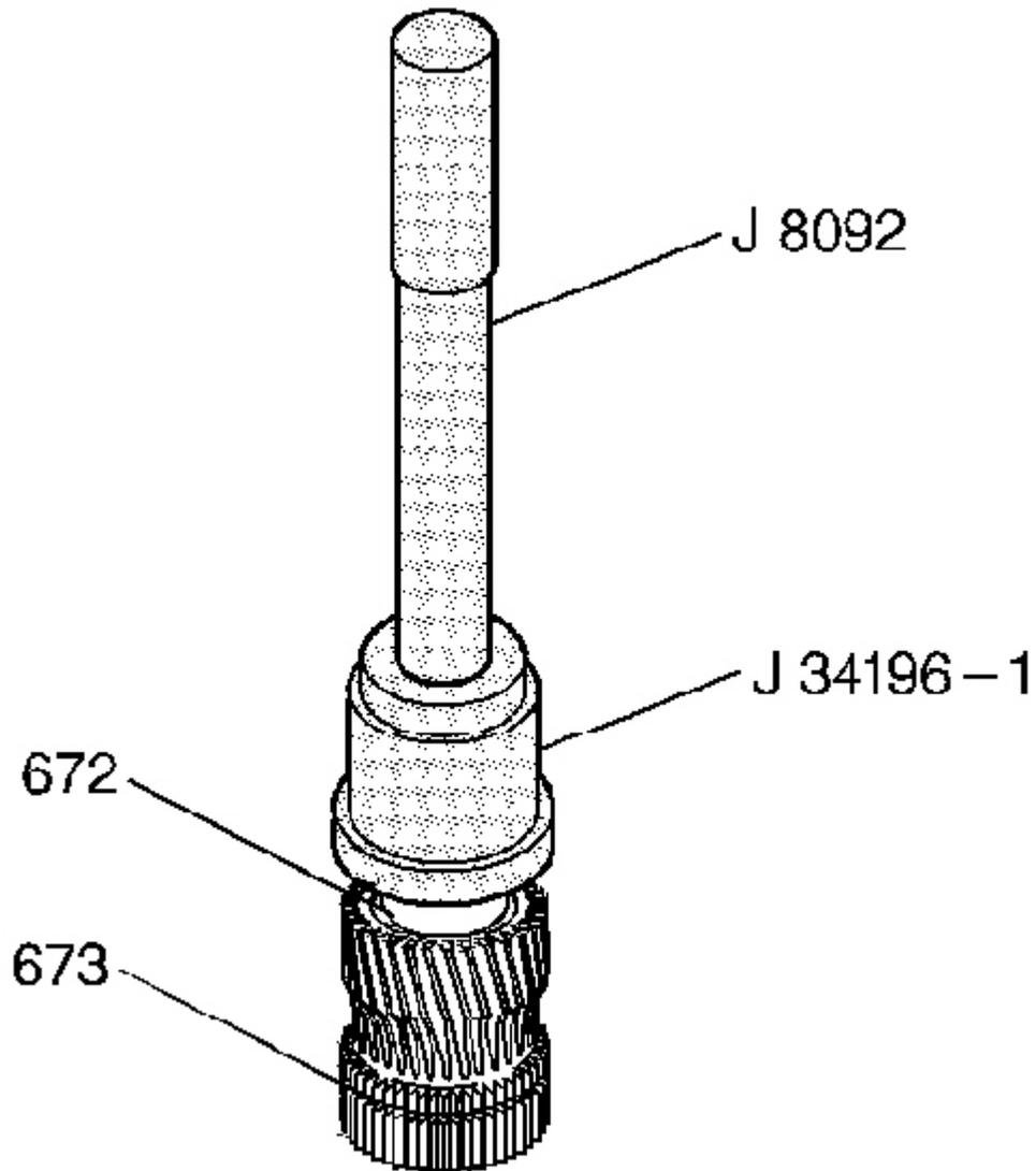
**Fig. 123: Removing Reaction Sun Bushing From Reaction Sun Gear**
