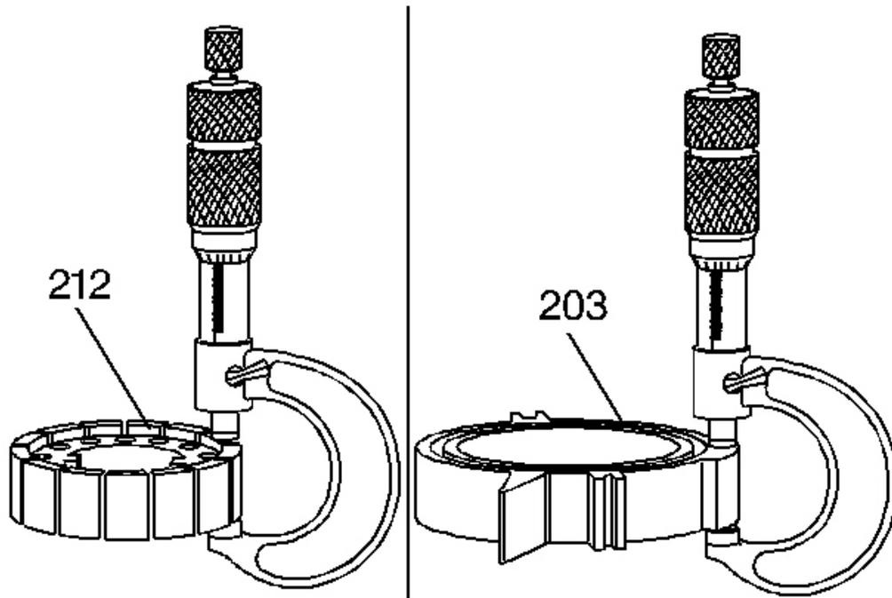
**Fig. 211: Measuring Oil Pump Rotor & Slide**
