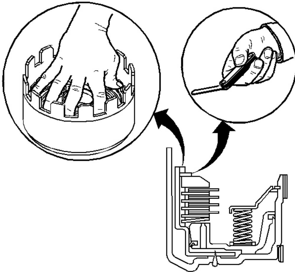
**Fig. 201: Checking Reverse Input Clutch Plate Travel**
