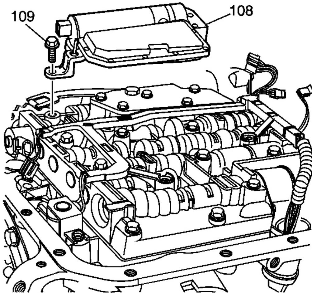
**Fig. 40: Identifying Secondary Fluid Pump**
