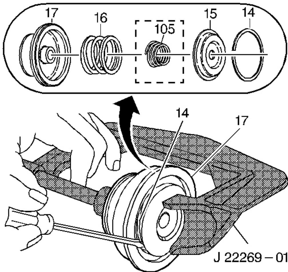
**Fig. 304: Locating Servo Cushion Outer & Inner Spring With Retainer**
