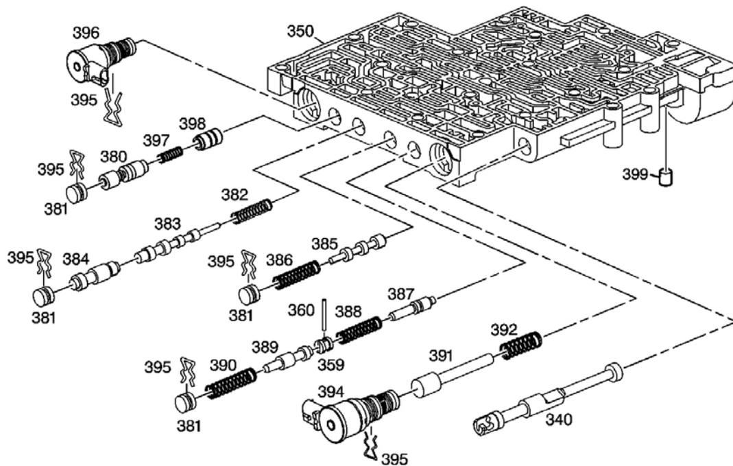
**Fig. 7: Control Valve Body Assembly Disassembled View (2 Of 2)**
