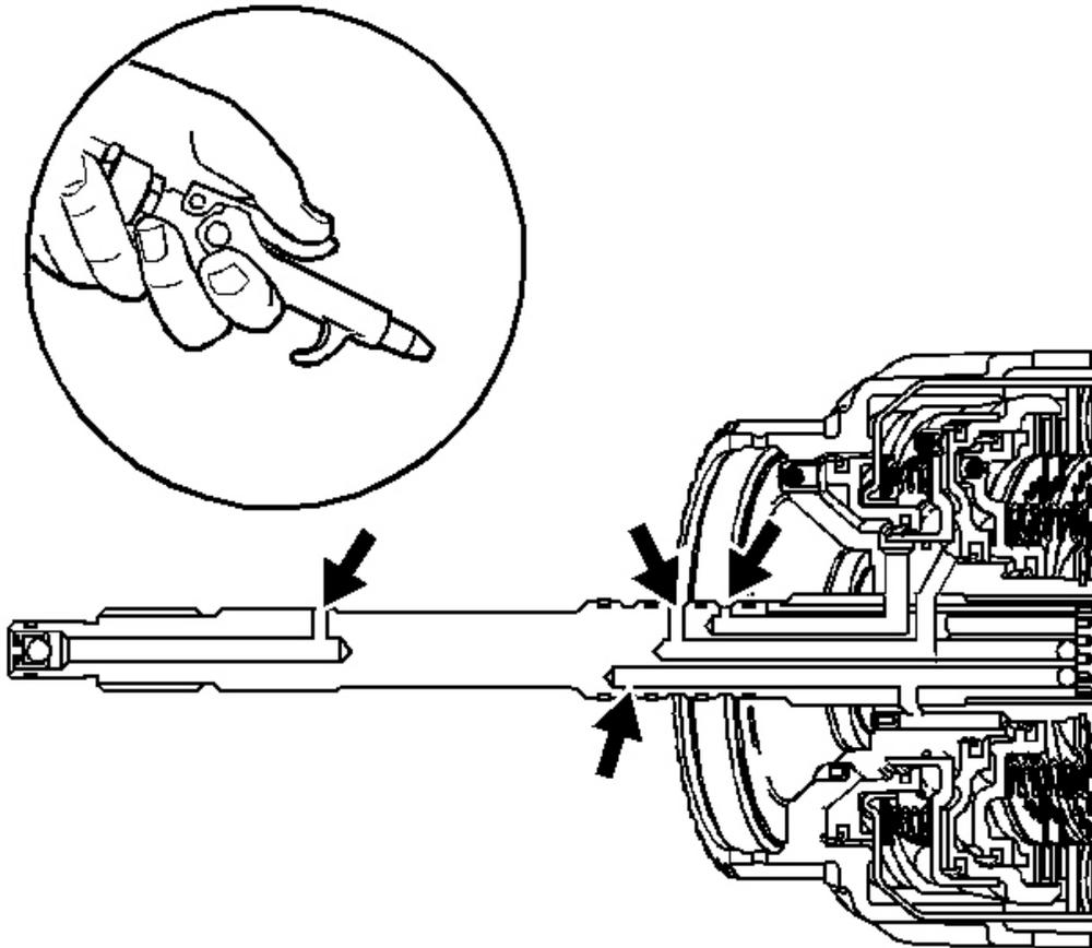
**Fig. 152: Blowing Air Into Oil Feed Passages**
