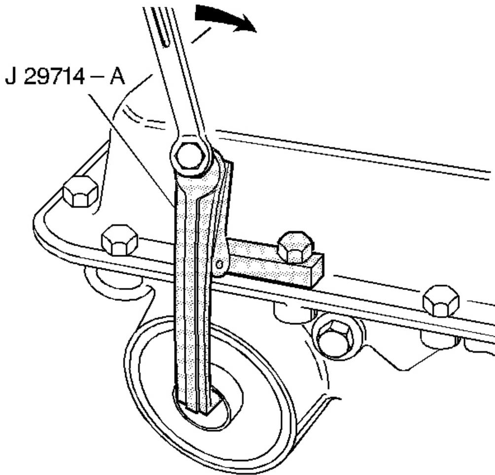
**Fig. 27: Compressing Servo Cover With J 29714-A**
