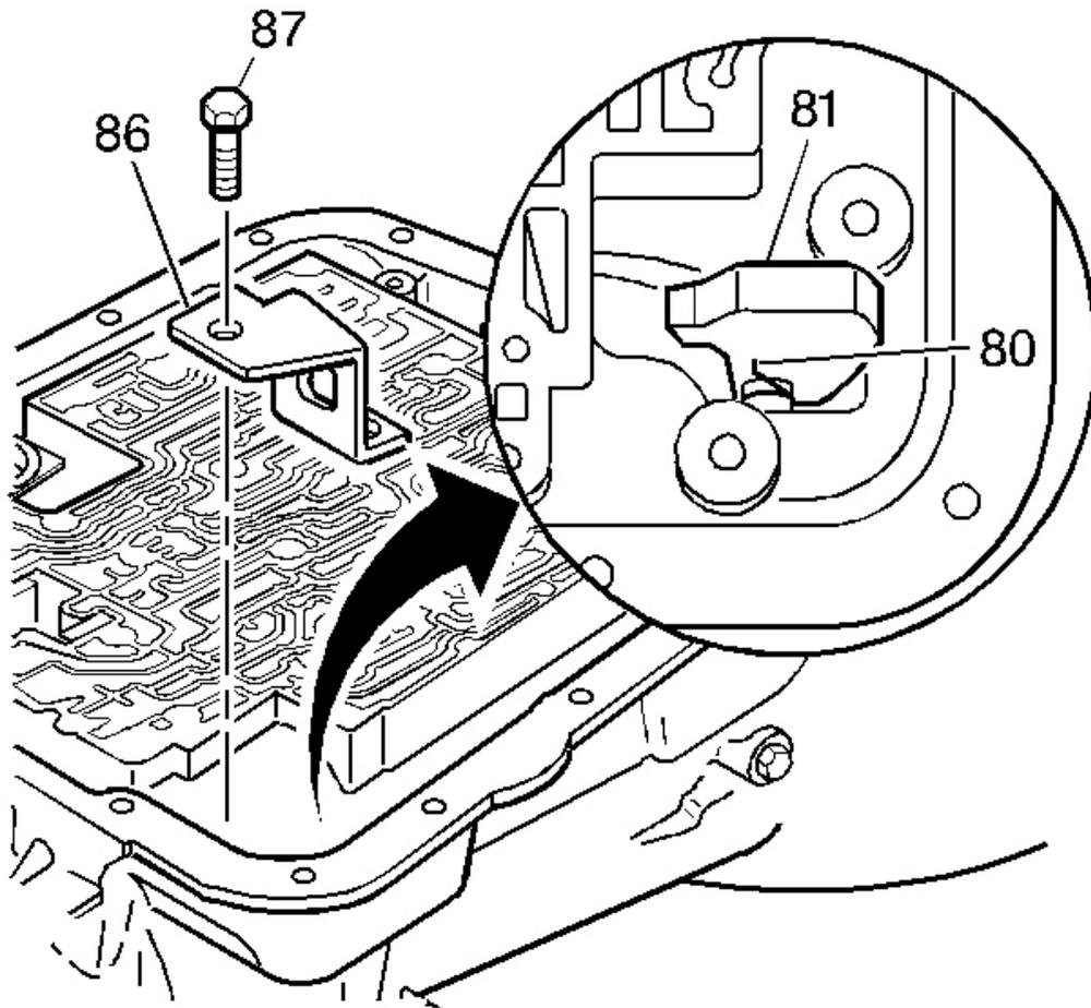
**Fig. 103: Locating Parking Brake Pawl & Return Spring**
