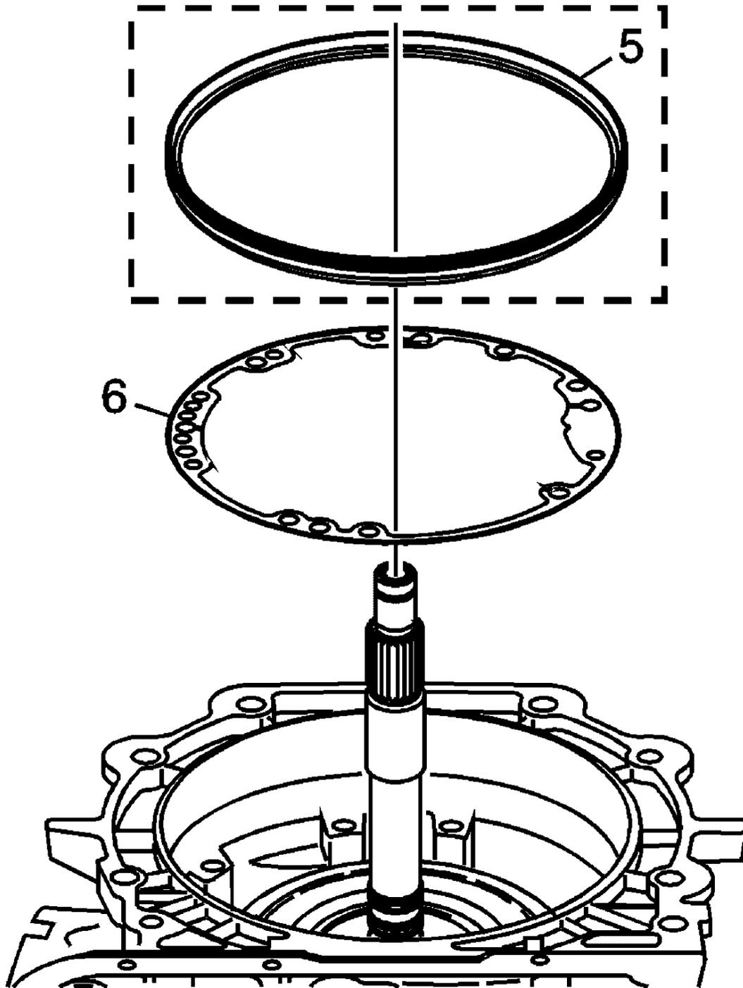
**Fig. 62: Identifying External Fluid Pump Seal**
