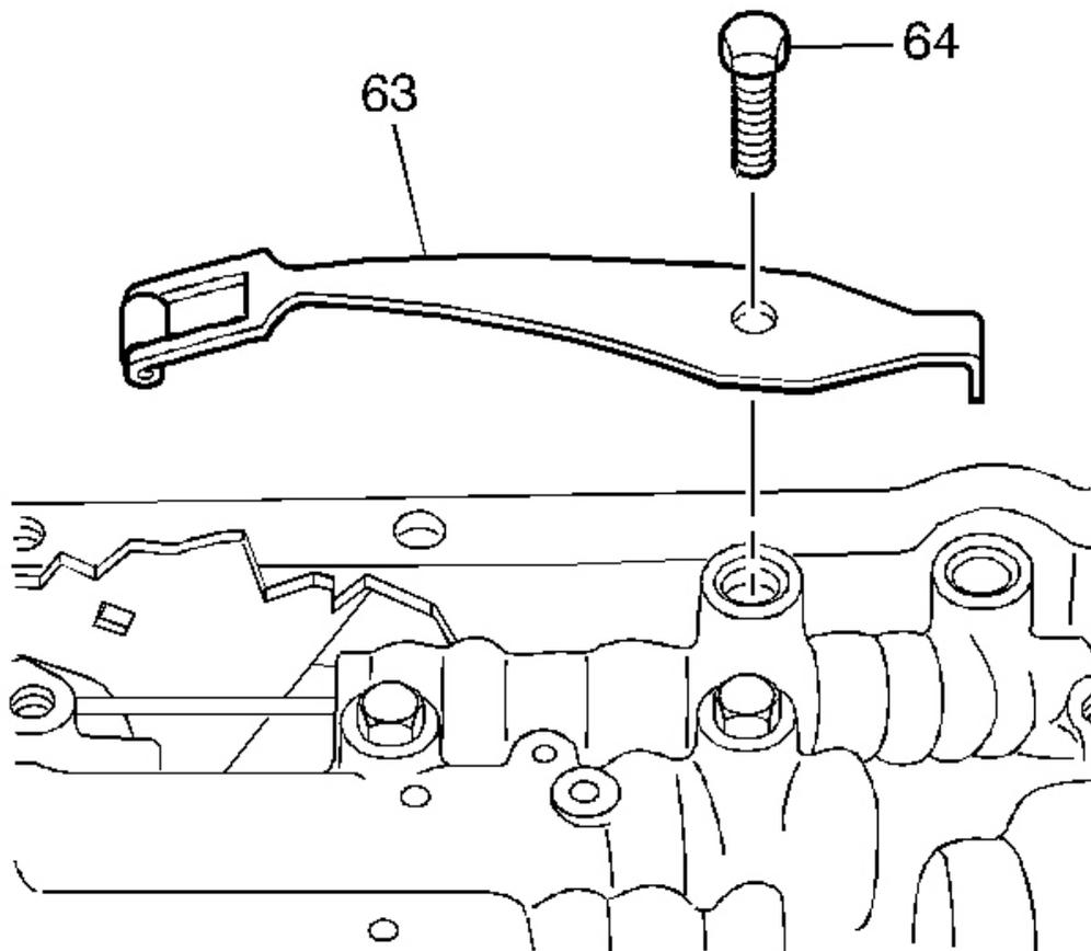
**Fig. 293: View Of Manual Detent Spring Assembly**
