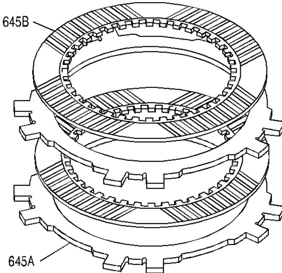
**Fig. 166: Identifying Overrun Clutch Plates**
