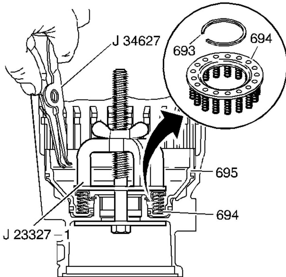
**Fig. 102: View Of Low And Reverse Clutch Spring Assembly & Retainer Ring**
