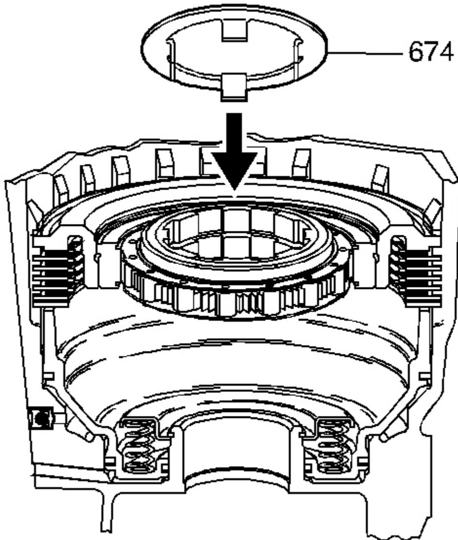
**Fig. 126: Aligning Thrust Washer Tangs With Low And Reverse Roller Clutch Race Splines**
