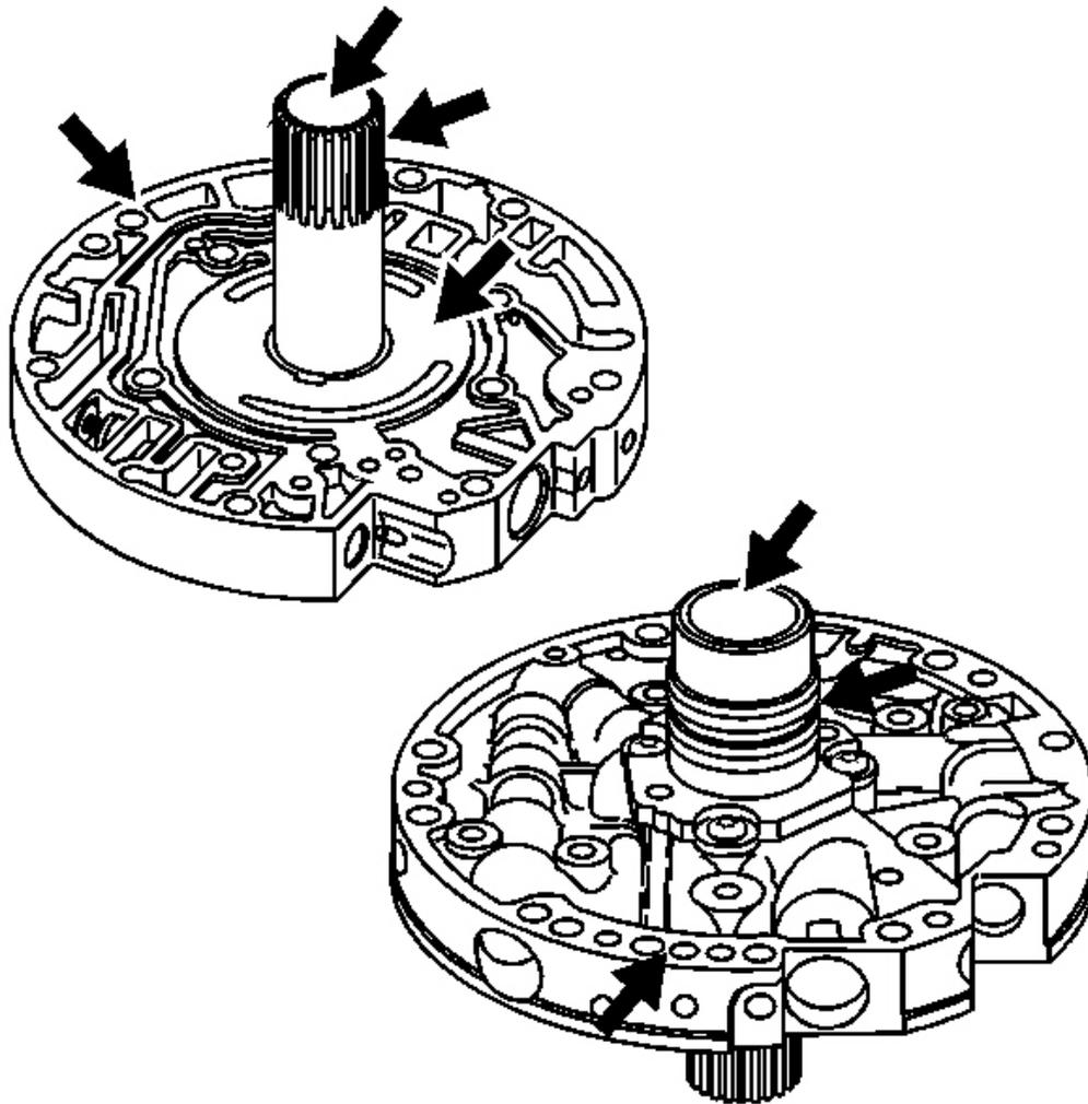
**Fig. 227: View Of Pump Cover Inspection Areas**
