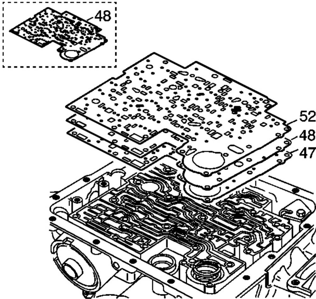
**Fig. 52: Identifying Valve Body Gasket**
