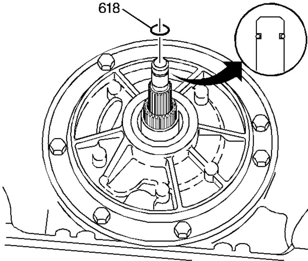
**Fig. 248: Identifying Turbine Shaft O-Ring**
