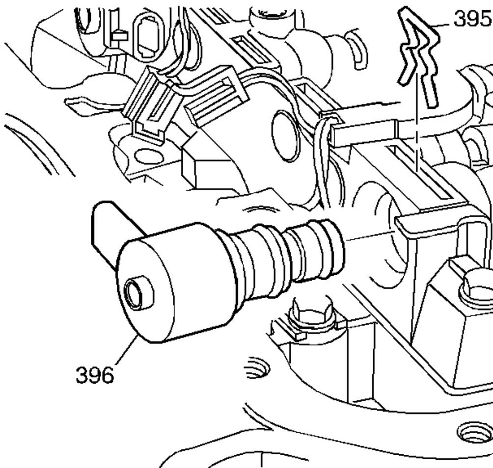
**Fig. 291: Locating TCC PWM Solenoid Valve**
