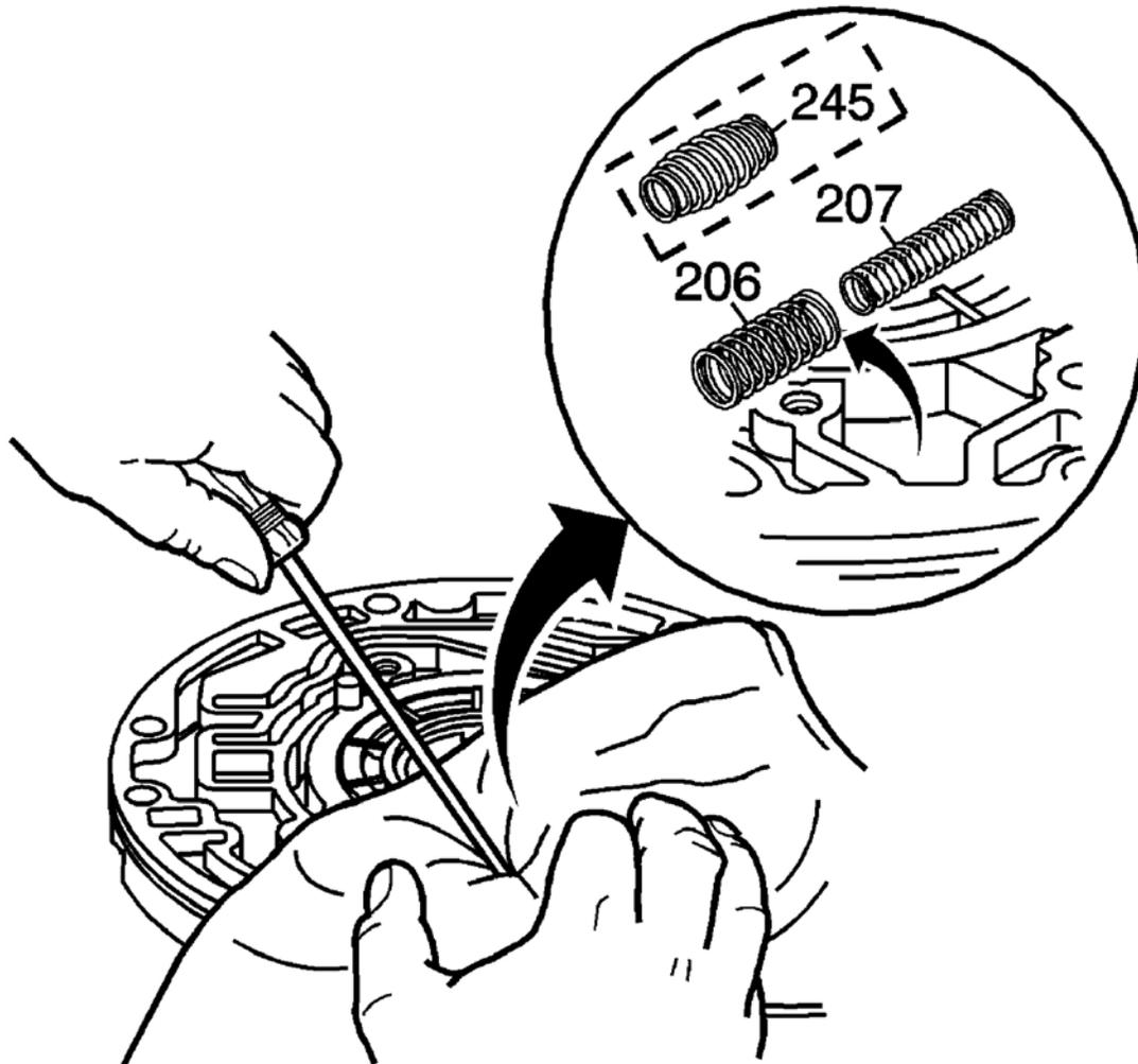
**Fig. 208: Retaining Pump Slide Springs With A Rag**
