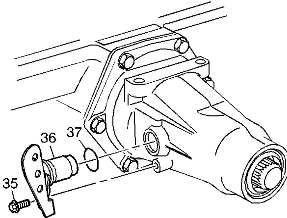
**Fig. 317: View Of Internal Transmission Speed Sensor**
