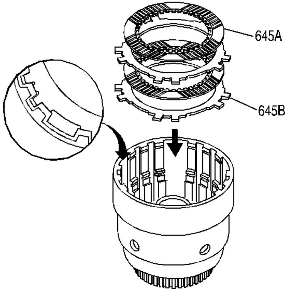
**Fig. 167: Aligning Overrun Clutch Plates**
