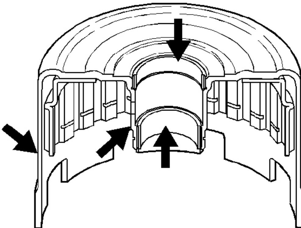
**Fig. 190: Inspection Areas On Reverse Input Clutch Housing & Drum Assembly**
