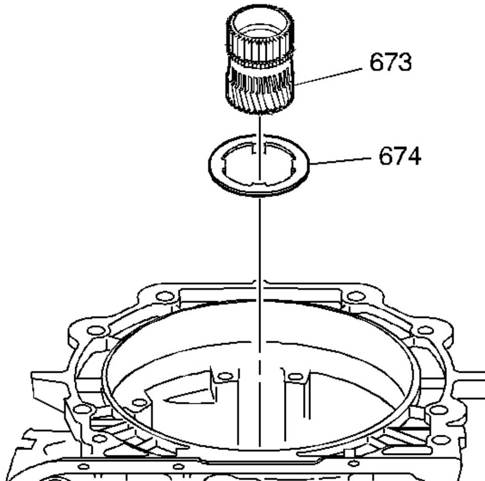
**Fig. 70: Identifying Reaction Sun Gear & Thrust Washer**
