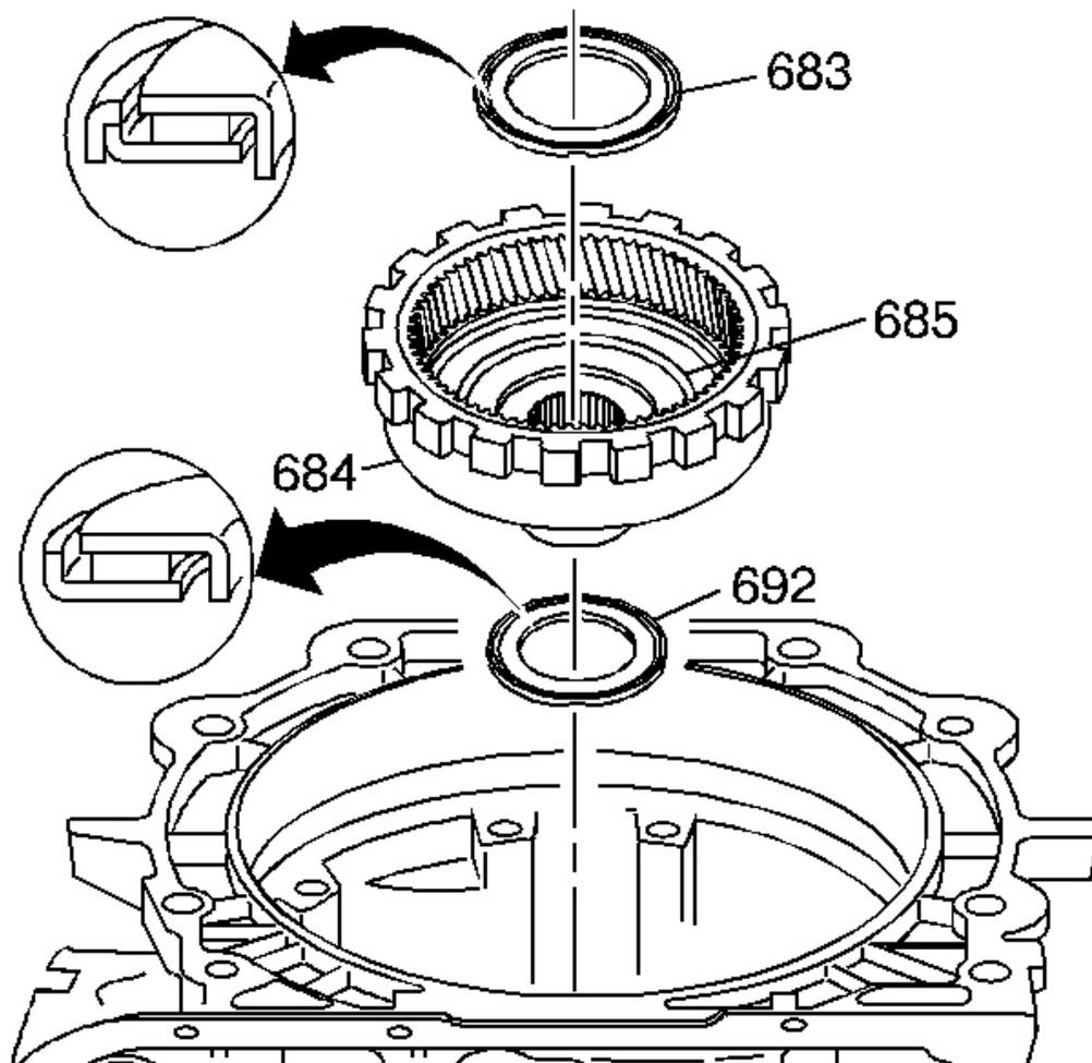
**Fig. 109: View Of Reaction Carrier/Support Thrust Bearing Assembly**
