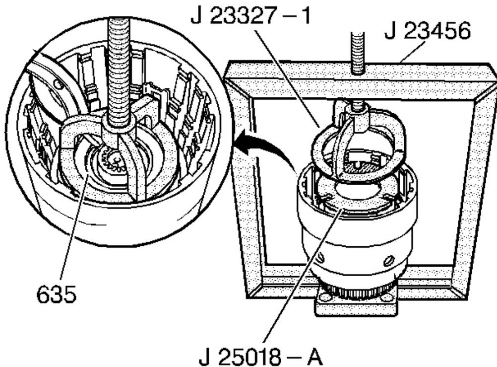
**Fig. 164: Locating Overrun Clutch Spring Retainer Snap Ring**
