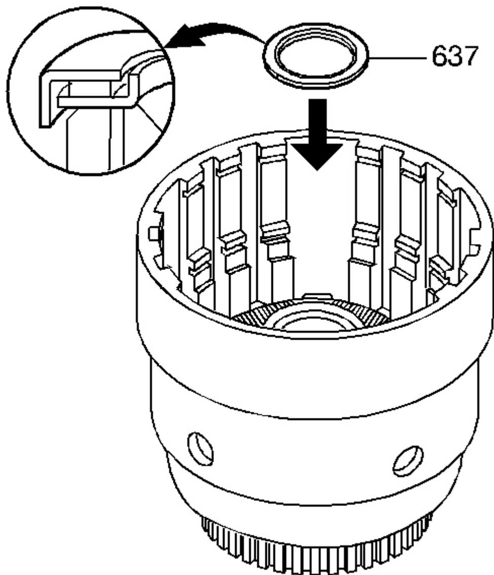
**Fig. 168: Input Sun Gear Bearing Assembly**
