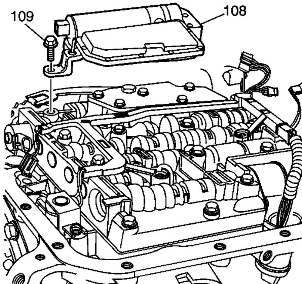
**Fig. 294: Identifying Secondary Fluid Pump**
