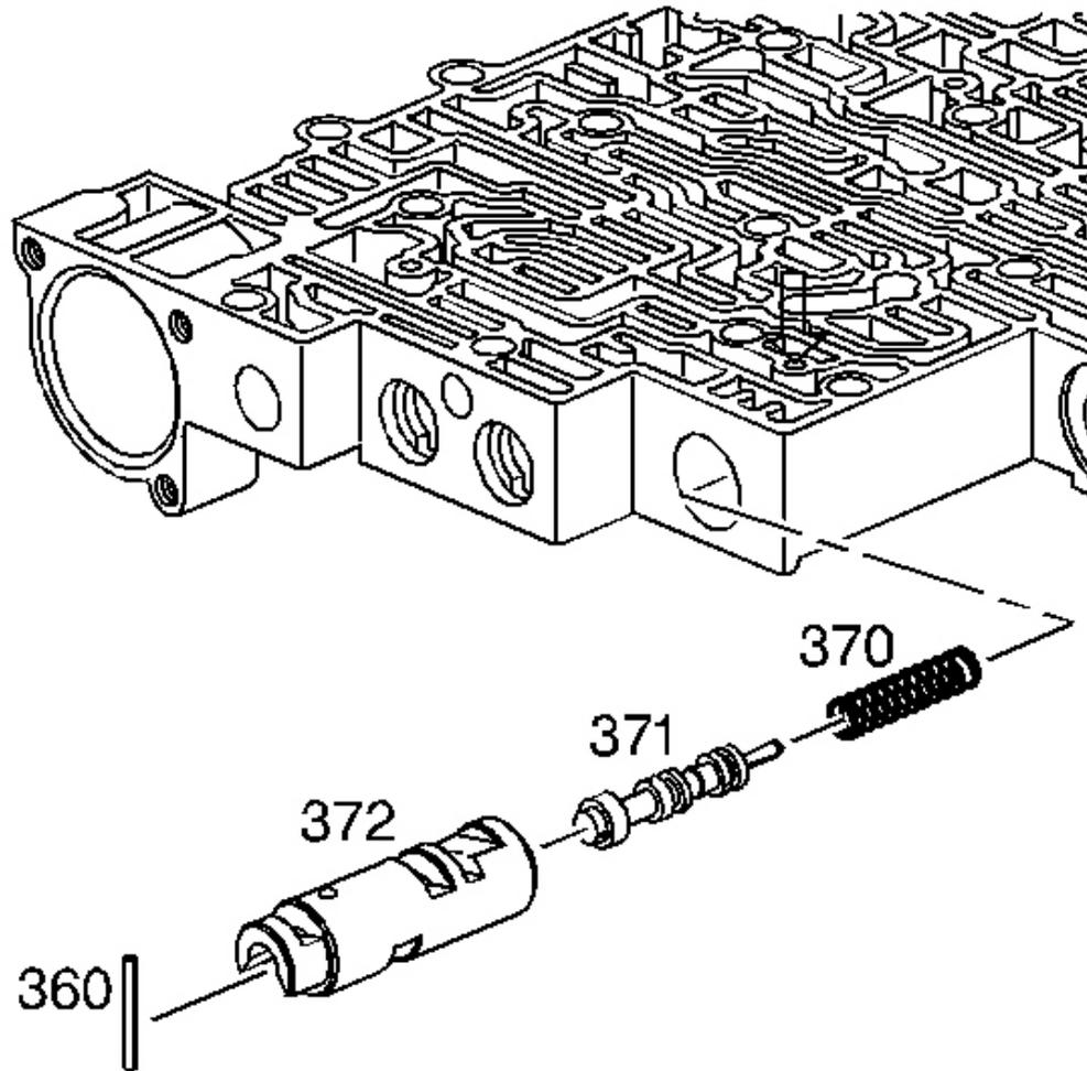
**Fig. 253: View Of 1-2 Accumulator Valve & 1-2 Accumulator Valve Sleeve**
