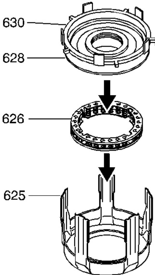
**Fig. 158: Locating 3rd & 4th Spring Assembly**
