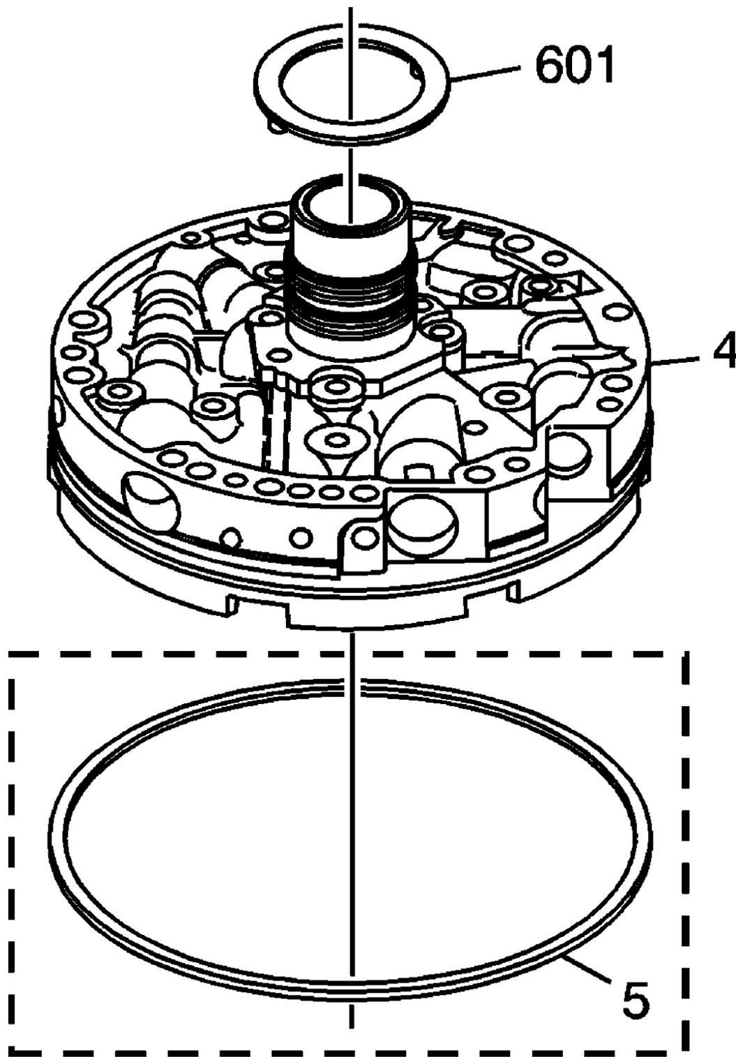
**Fig. 239: View Of Pump To Drum Thrust Washer**
