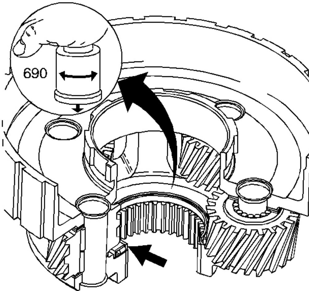
**Fig. 108: Illustrating Proper Inspection Of Reaction Carrier Captive Thrust Bearing**
