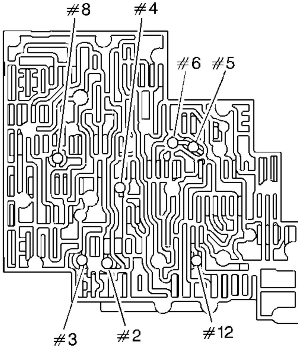
**Fig. 284: Identifying Checkball Installation Positions**
