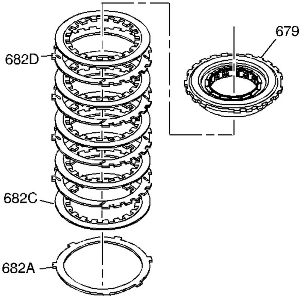
**Fig. 112: View Of Low And Reverse Clutch Plate Assembly**
