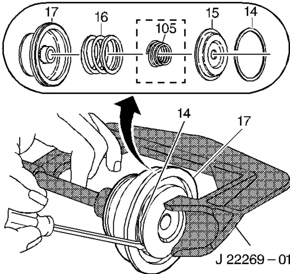
**Fig. 300: Locating Servo Cushion Outer & Inner Spring With Retainer**
