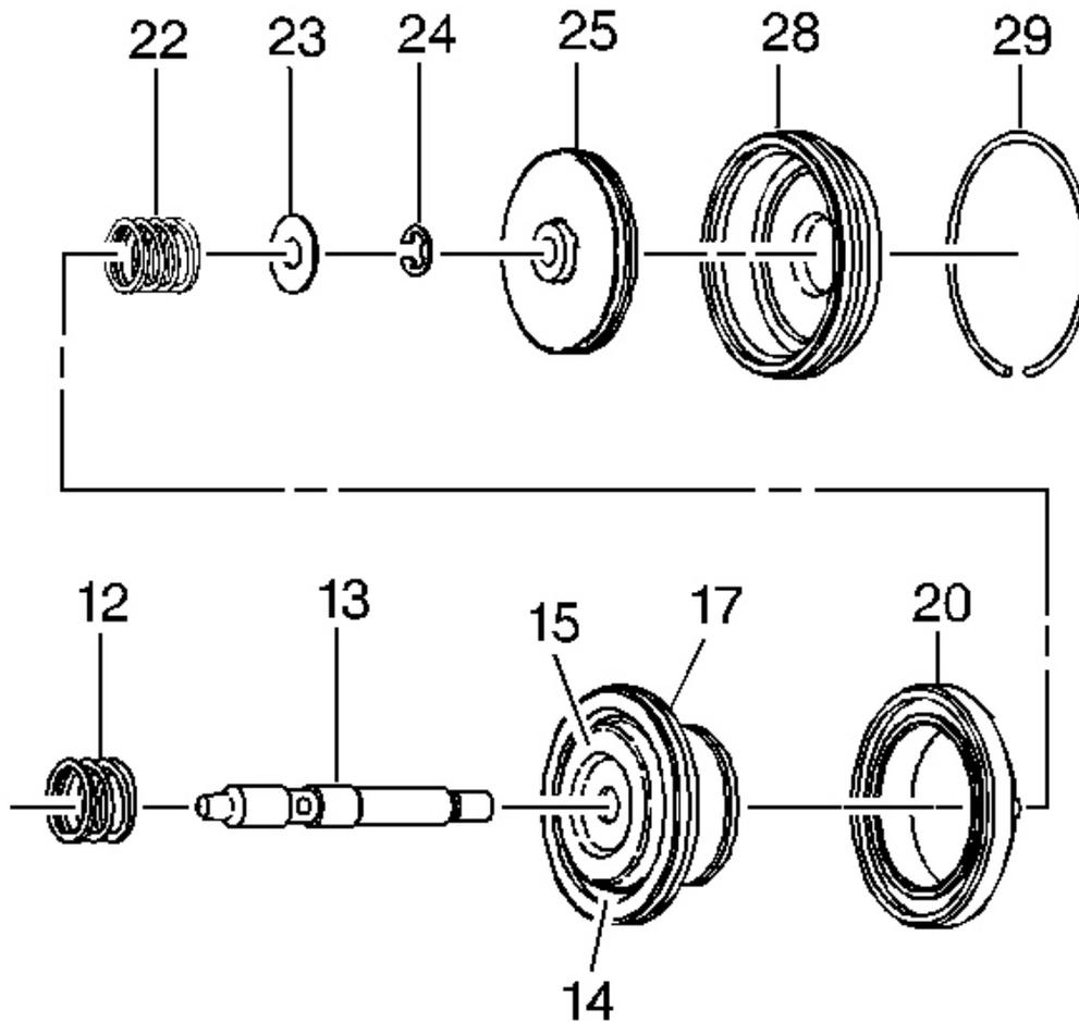
**Fig. 305: Illustrating Assembly Order Of 2-4 servo components**
