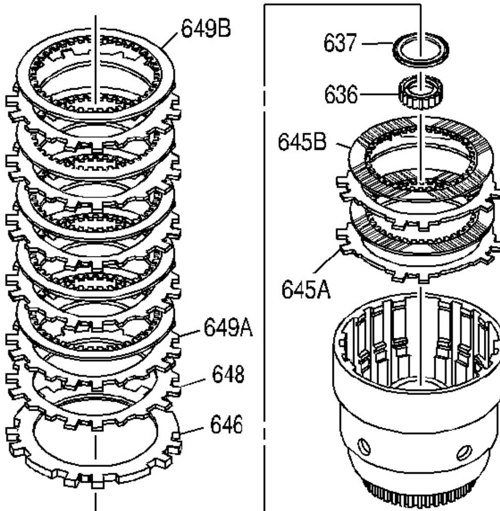
**Fig. 148: View Of Forward Clutch Plates**
