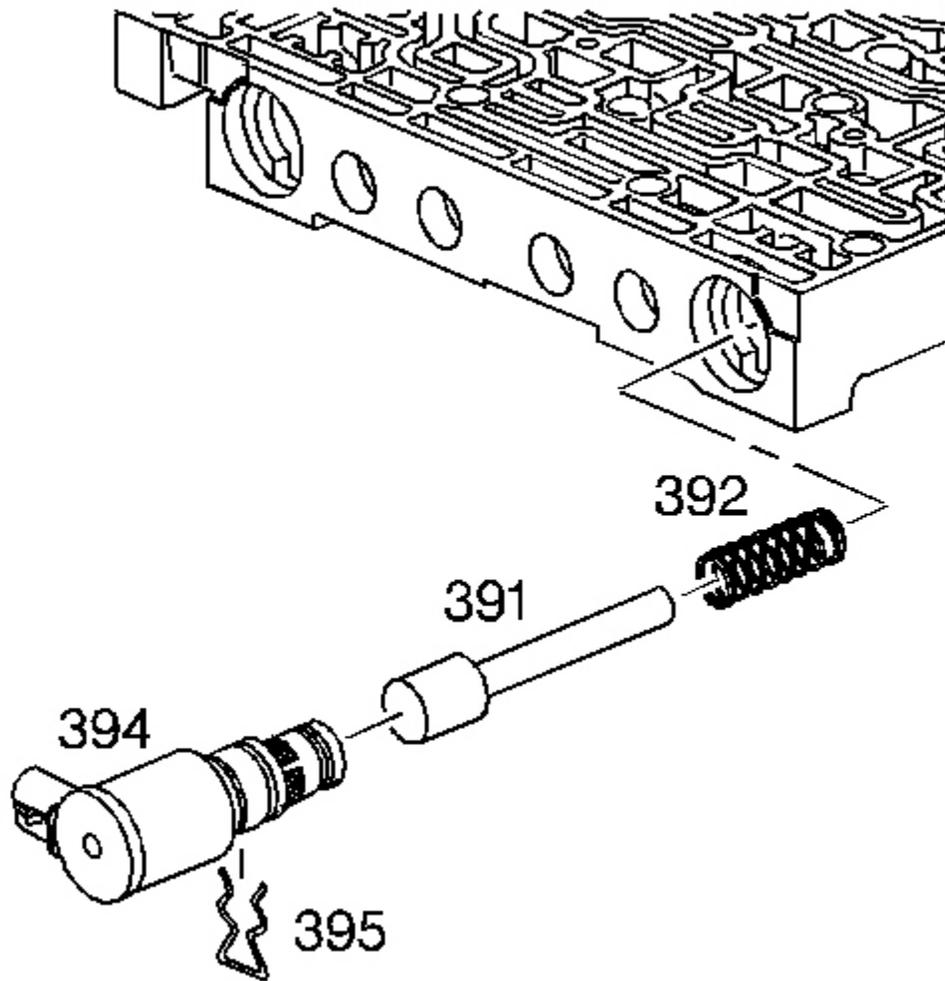
**Fig. 265: Identifying 3-2 Control Valve & 3-2 Control Solenoid**
