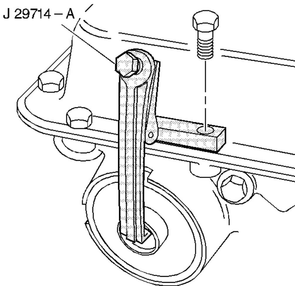
**Fig. 26: Installing J 29714-A**
