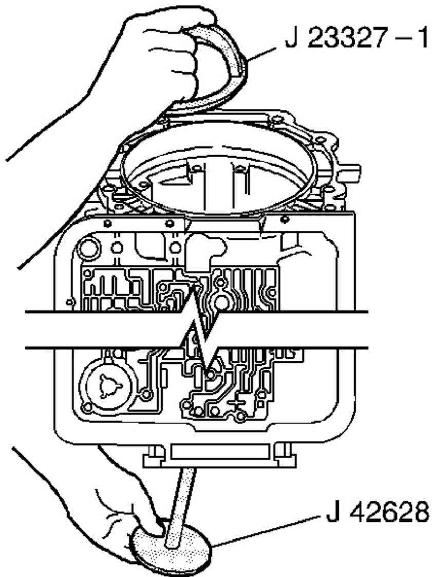
**Fig. 82: Installing J 23327-1 & J 42628**
