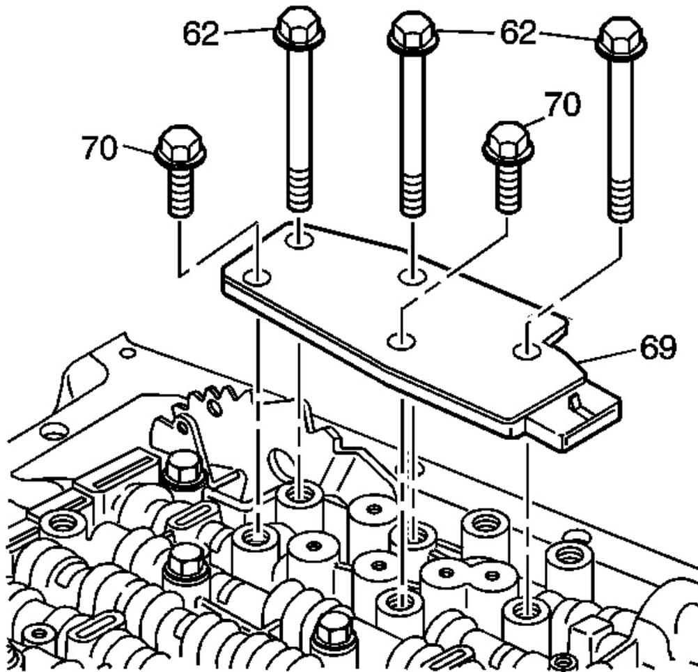
**Fig. 45: TFP Manual Valve Position Switch Retaining Bolts**
