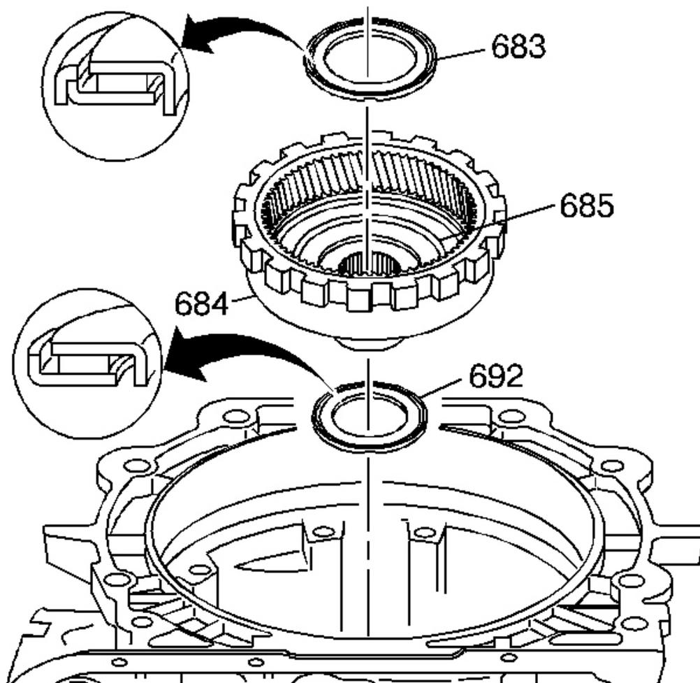
**Fig. 78: View Of Reaction Carrier/Support Thrust Bearing Assembly
