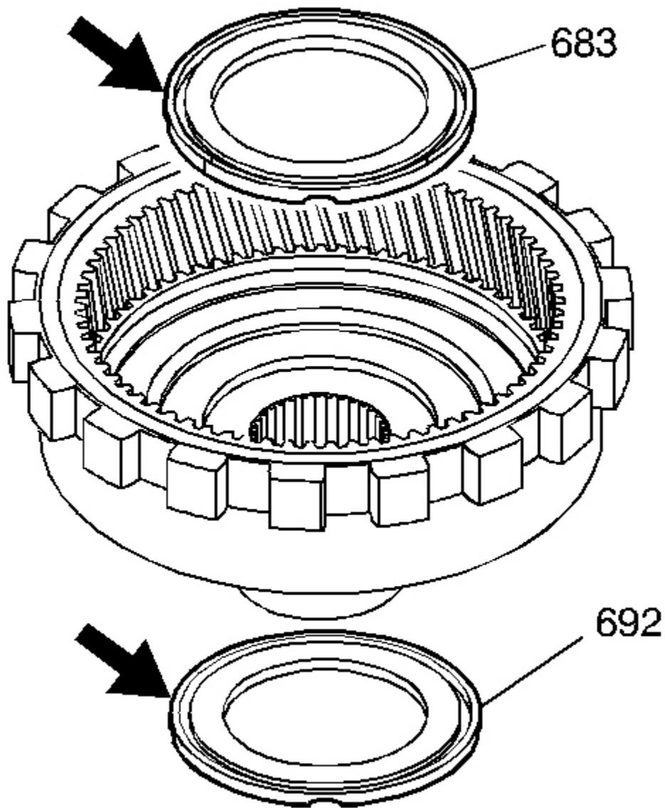
**Fig. 105: Inspecting Areas Of Reaction Carrier/Support Thrust Bearing Assembly**
