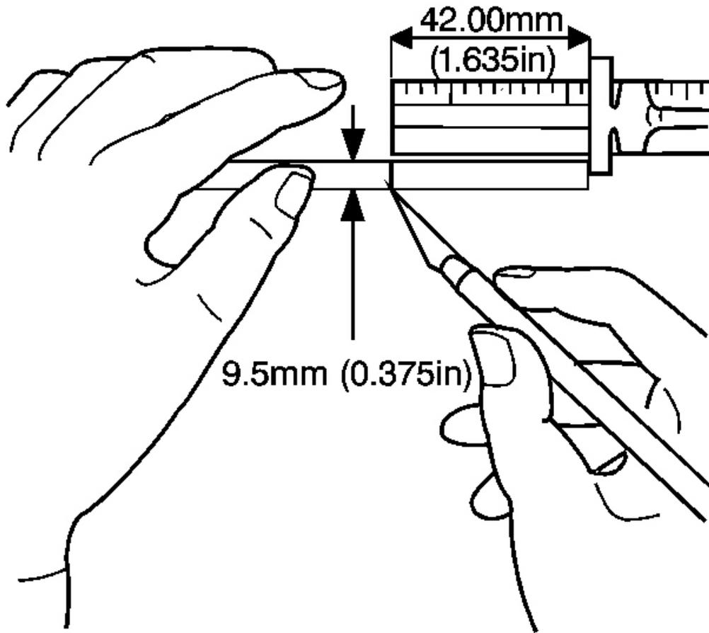
**Fig. 93: Scribing Mark On Rod For Gaging Proper Depth Of Third Accumulator Retainer And Ball Assembly**
