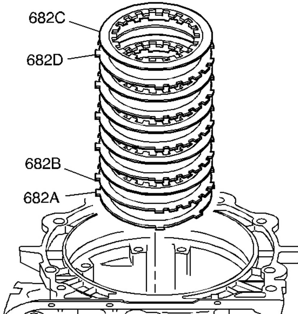
**Fig. 77: Locating Low And Reverse Clutch Components**
