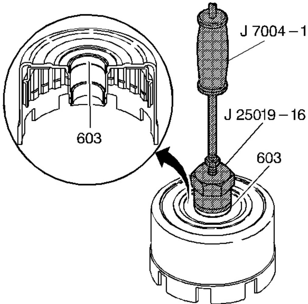
**Fig. 191: Identifying Reverse Input Clutch Front Bushing**
