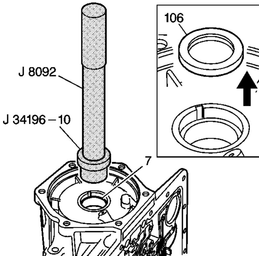
**Fig. 97: Identifying Case Rear Oil Seal & Case Bushing**
