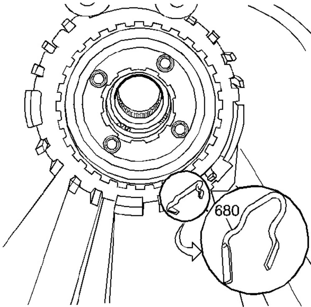
**Fig. 75: View Of Low And Reverse Clutch Support Retainer Spring**
