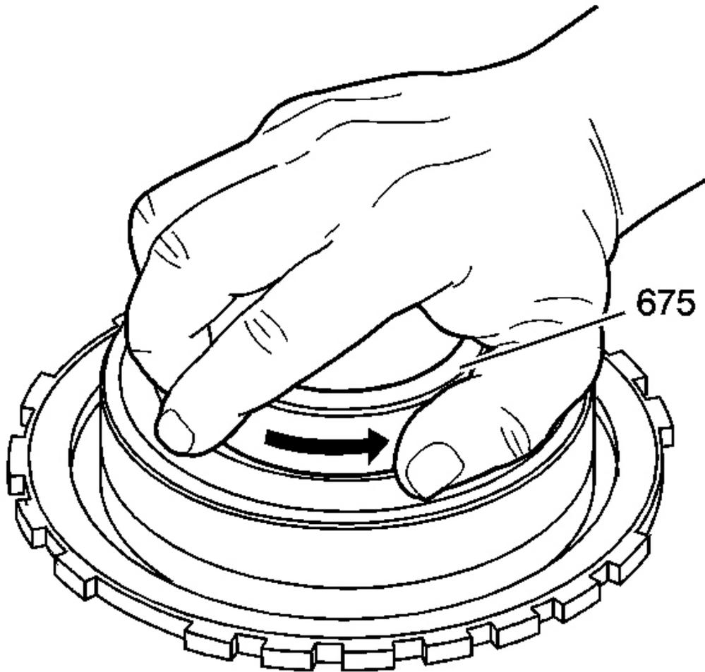
**Fig. 118: Checking Low And Reverse Roller Clutch Race Rotation**
