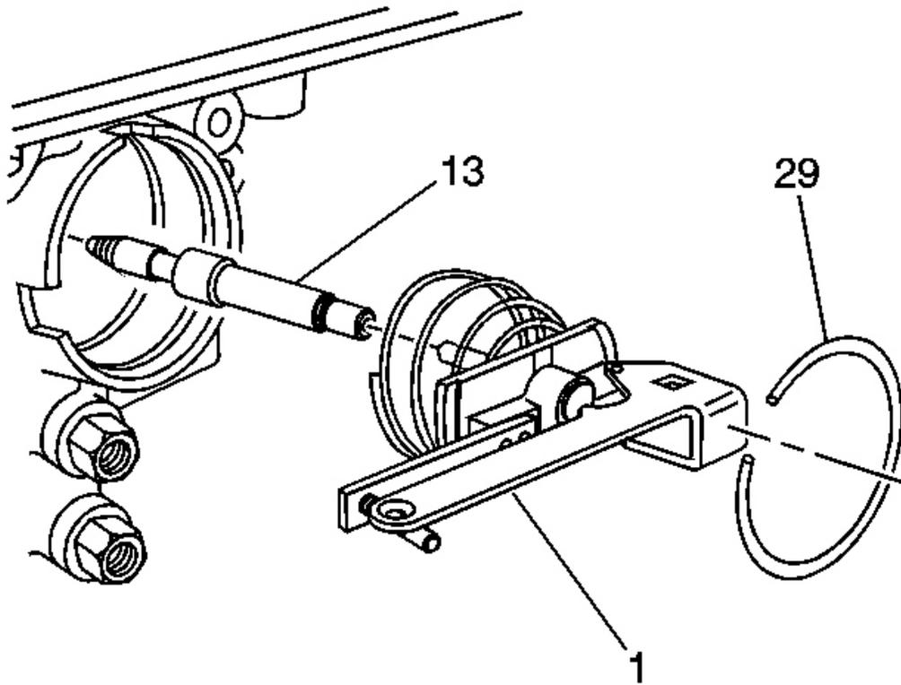
**Fig. 31: Locating Servo Cover Retaining Ring**
