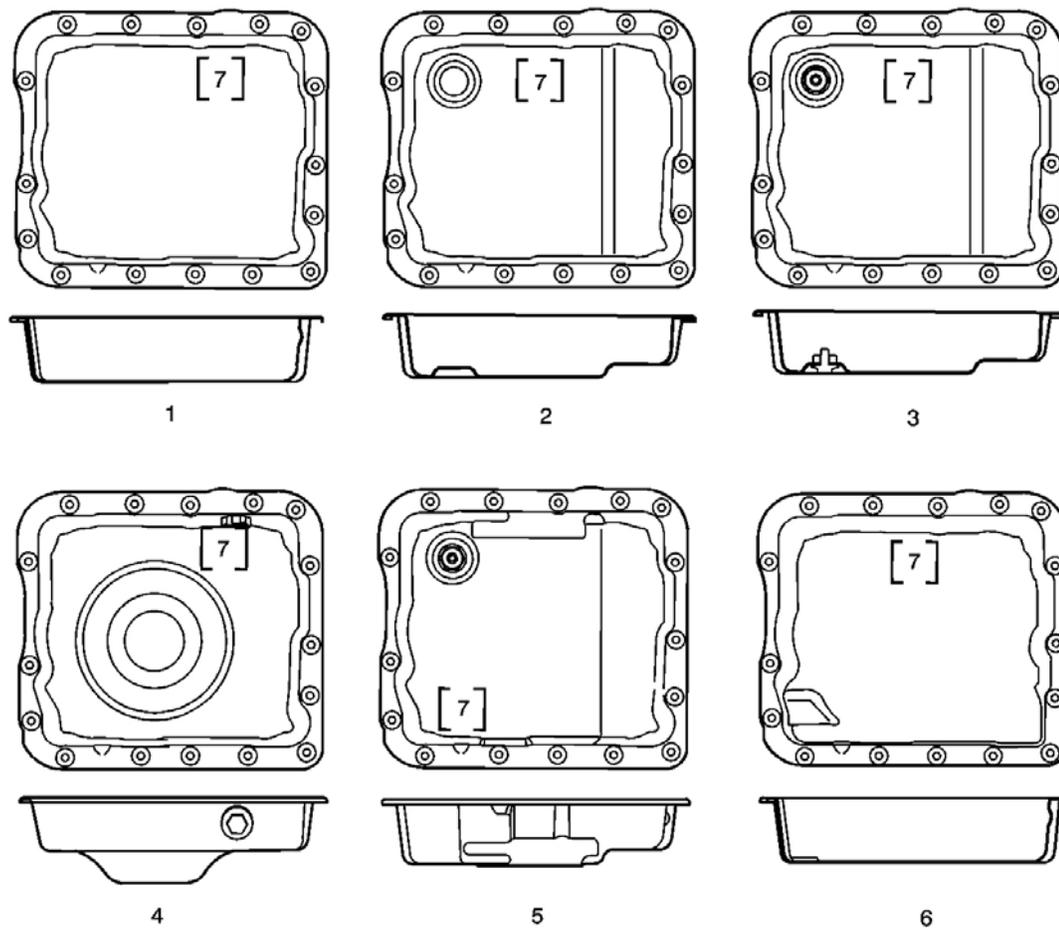
**Fig. 20: Fluid Pan Identification**
