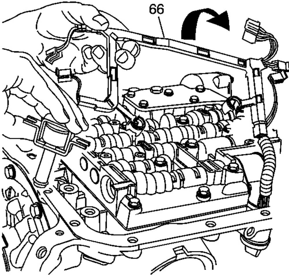
**Fig. 44: Removing TCC Solenoid And Wiring Harness**
