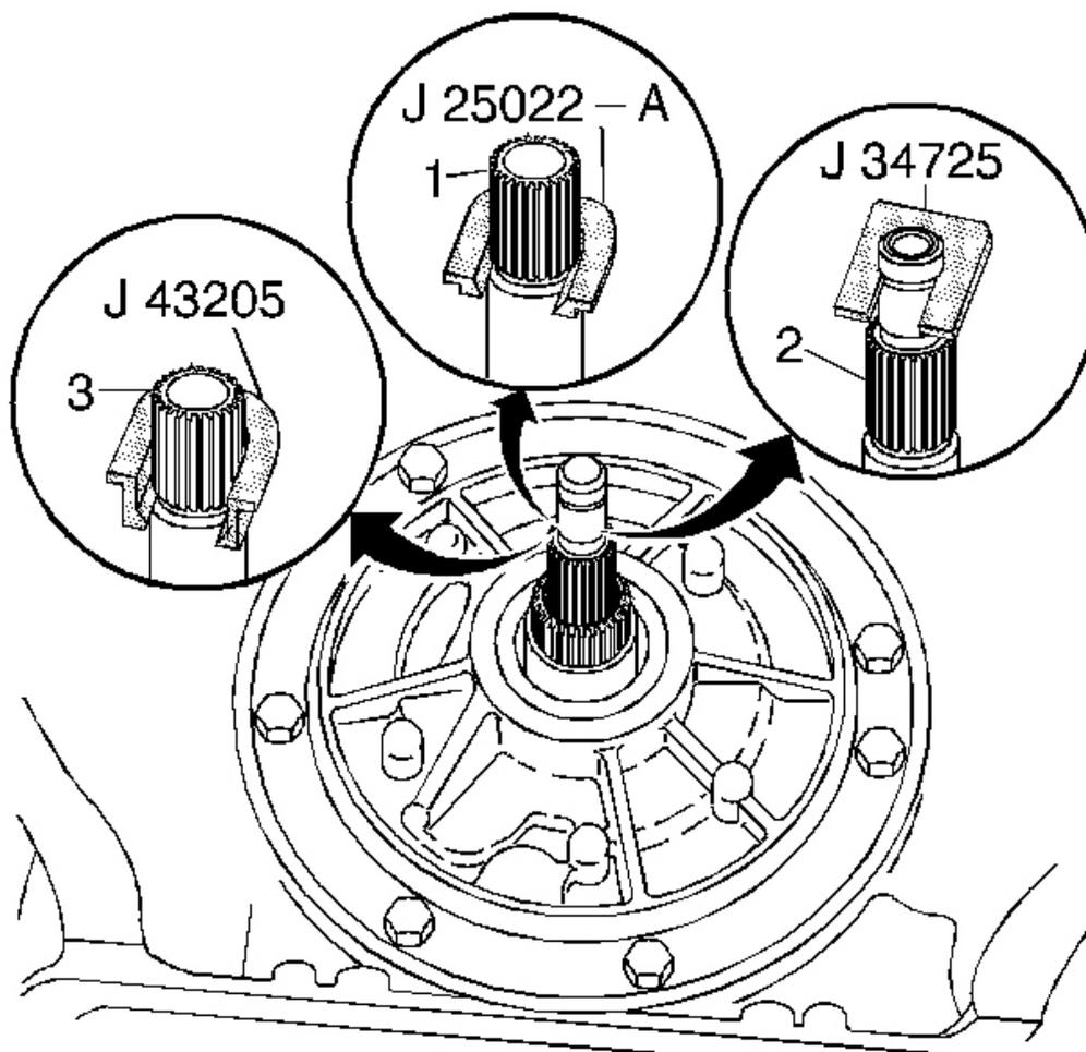
**Fig. 243: Identifying Different End Play Fixture Adapters**
