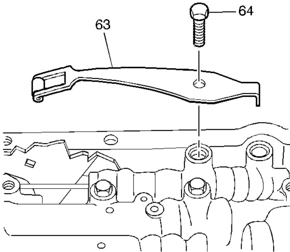
**Fig. 46: View Of Manual Detent Spring Assembly**
