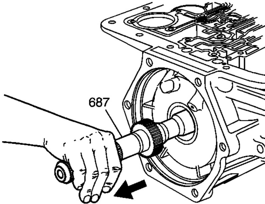
**Fig. 74: Locating Output Shaft**
