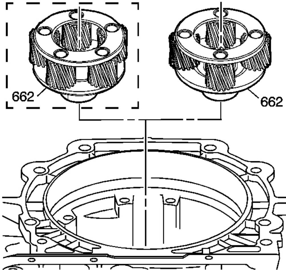
**Fig. 142: Locating Input Carrier Assembly**
