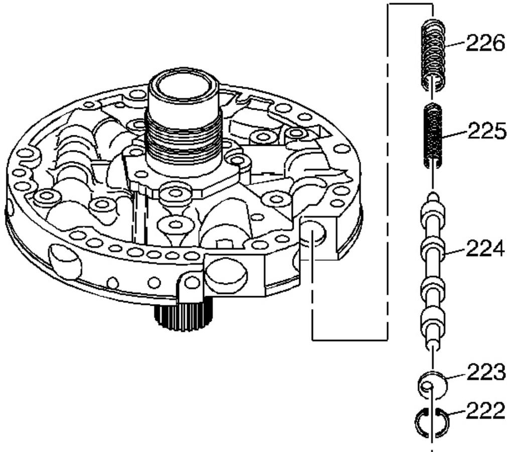
**Fig. 223: Locating Converter Clutch Valve**
