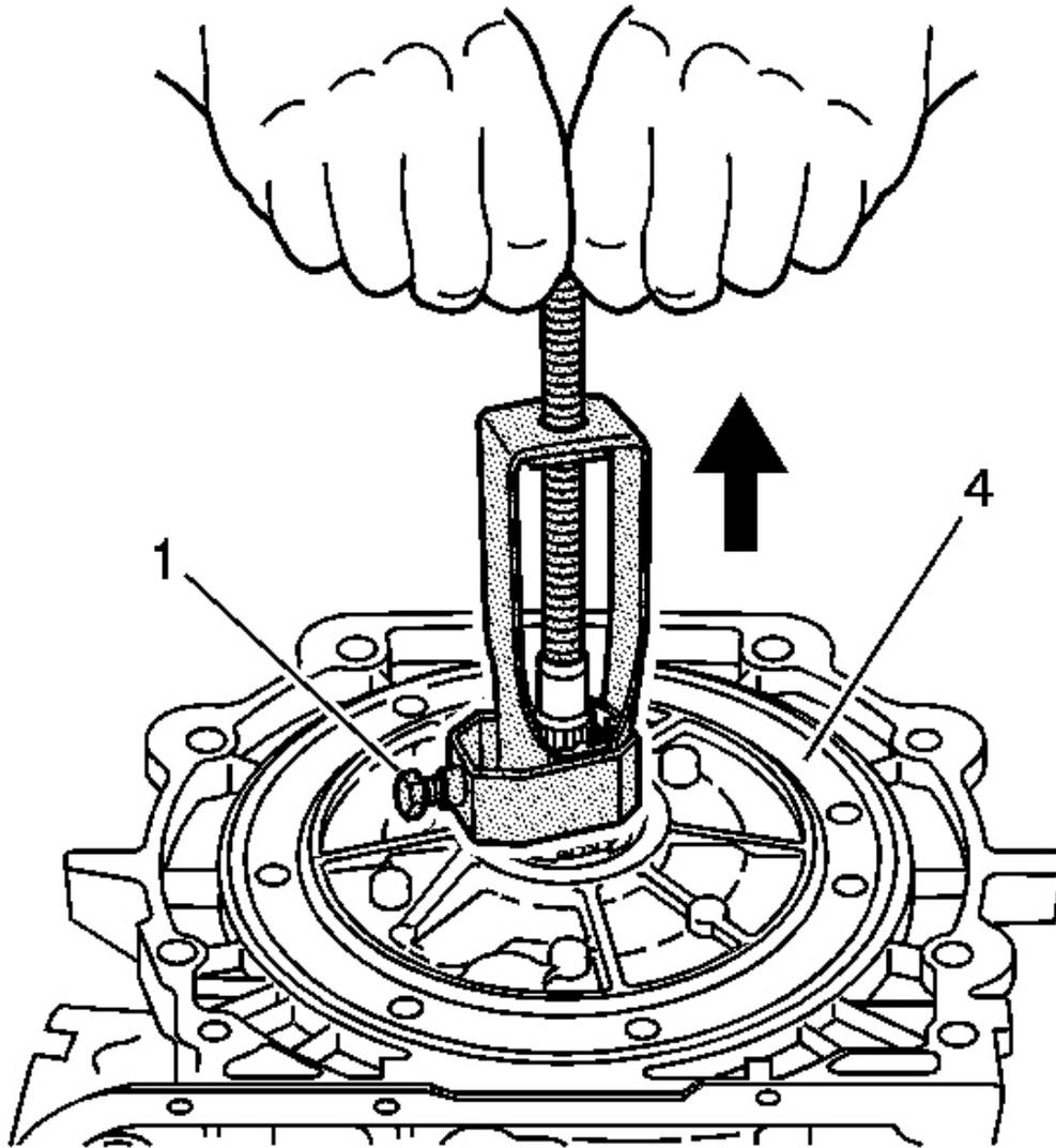
**Fig. 61: Installing J 37789-A & J 39119**
