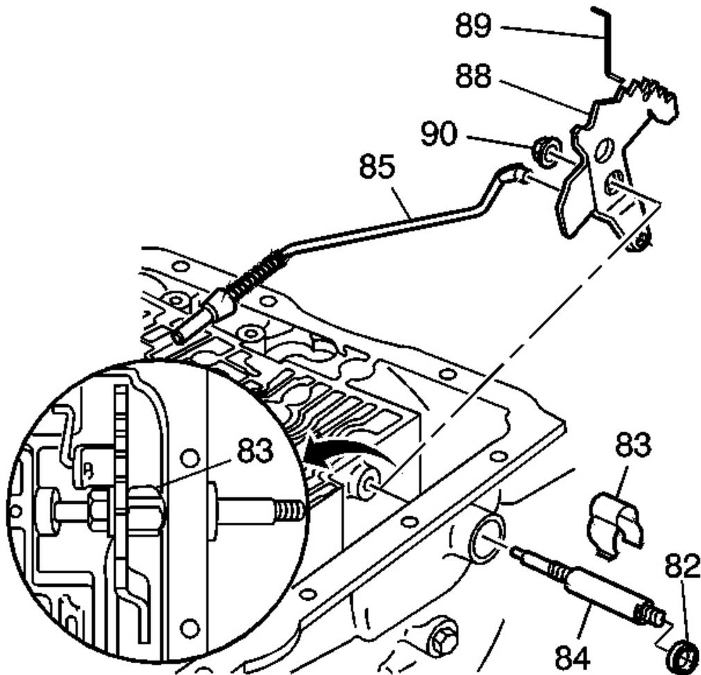
**Fig. 79: Inspecting Inner Manual Linkage**
