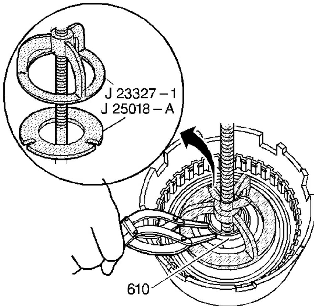
**Fig. 188: View Of Reverse Input Clutch Spring Retainer Ring**
