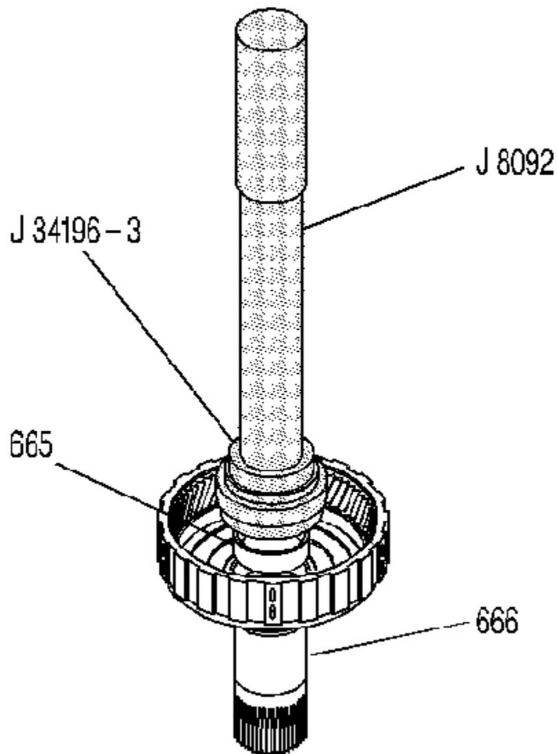
**Fig. 130: Installing Reaction Carrier Shaft Front Bushing**
