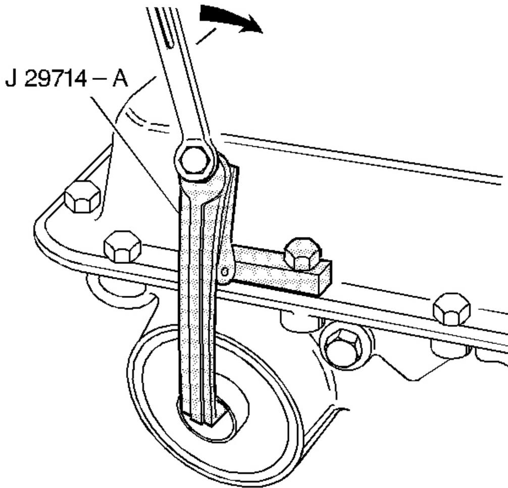
**Fig. 308: Compressing Servo Cover With J 29714-A**
