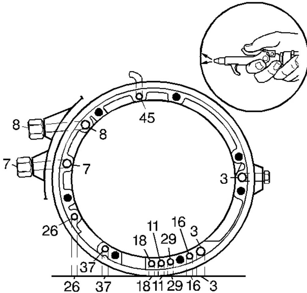
**Fig. 86: Identifying Case Fluid Passages**
