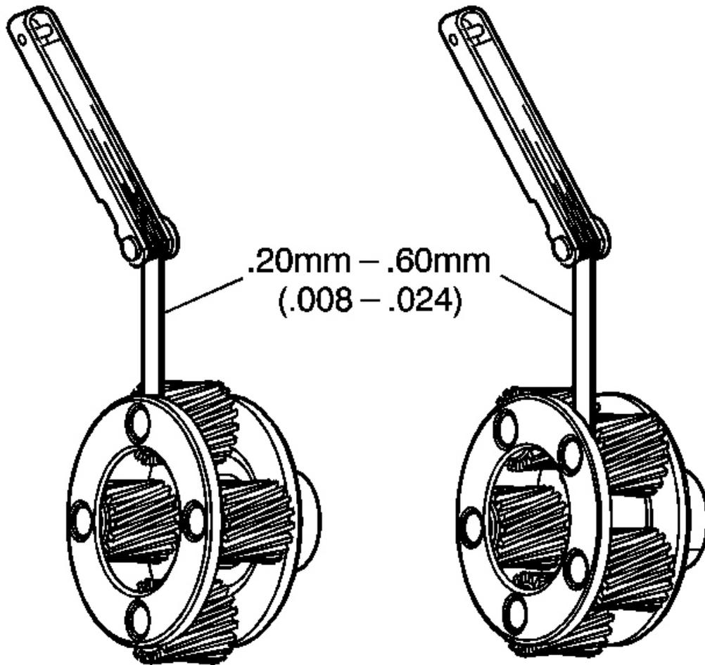
**Fig. 138: Identifying Input Carrier Pinion End Play Measurements**
