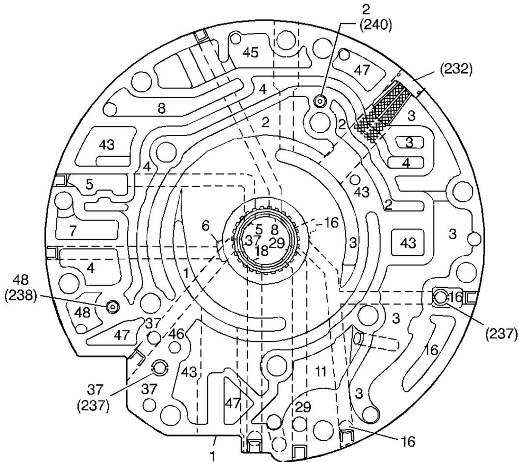
**Fig. 336: Pump Cover Fluid Passages (Pump Body Side)**
