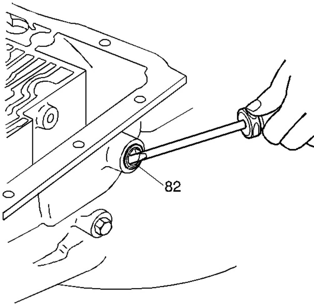
**Fig. 80: Removing Manual Shaft Seal**
