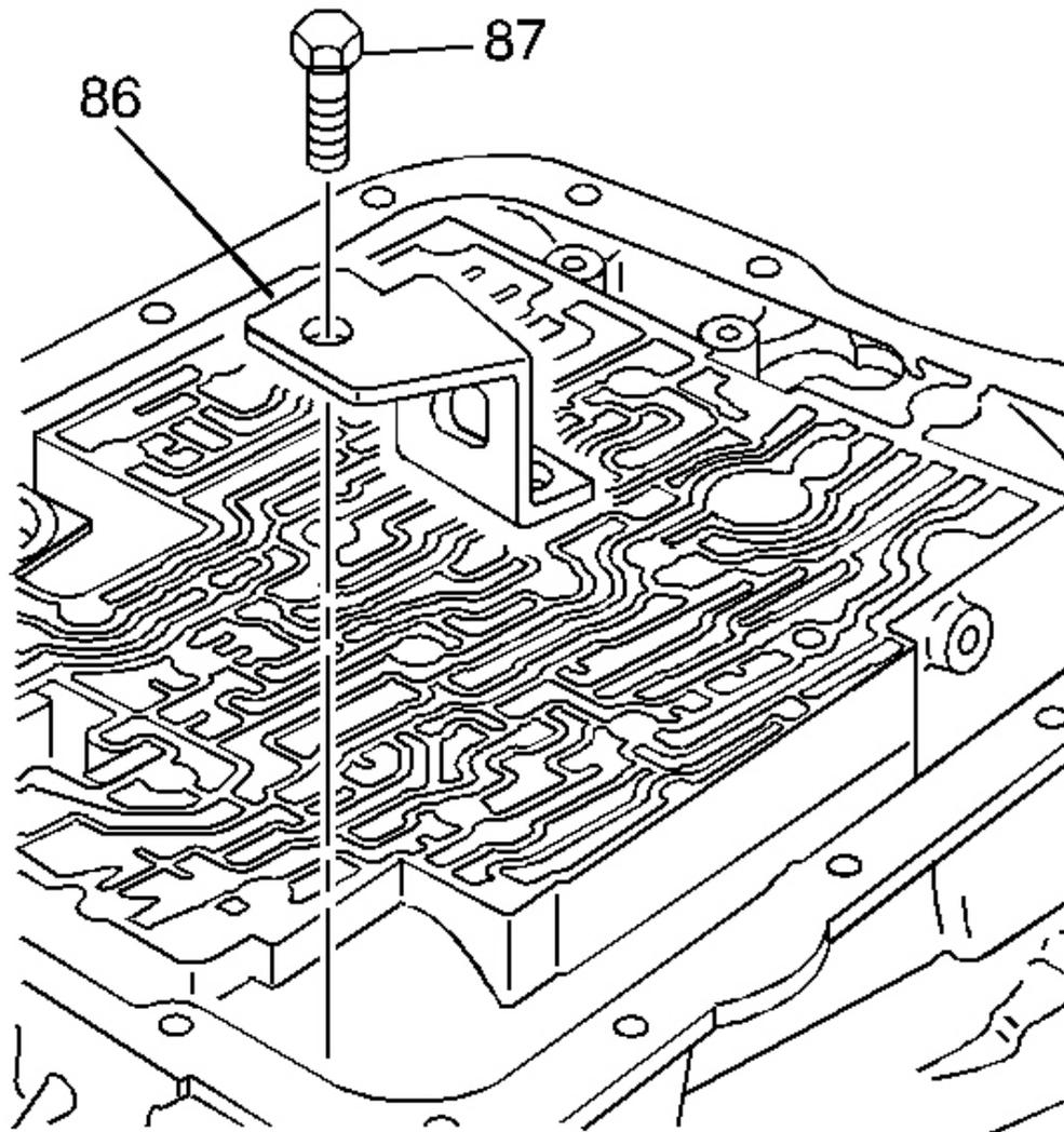
**Fig. 81: View Of Parking Lock Bracket & Bolt**
