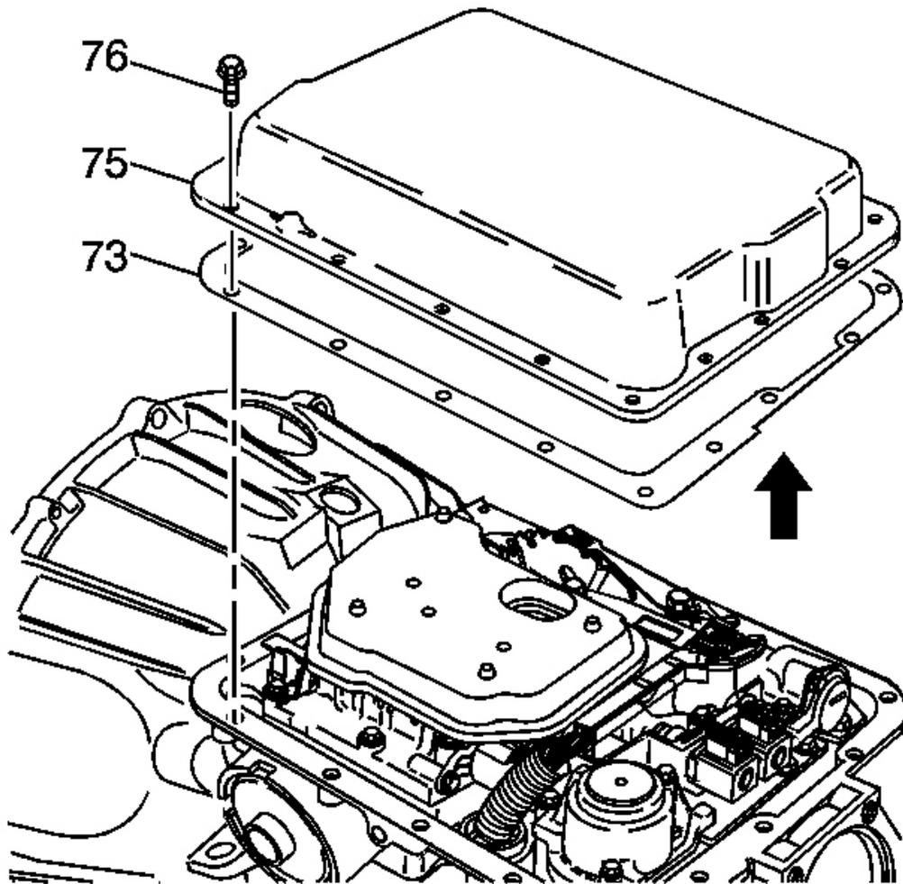
**Fig. 36: View Of Transmission Oil Pan & Gasket**
