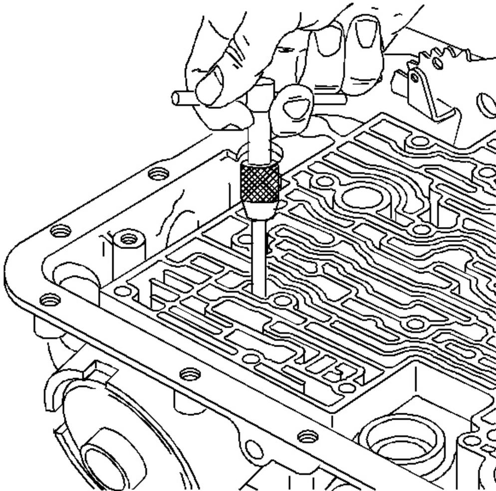
**Fig. 92: Extracting Third Accumulator Retainer And Ball Assembly**
