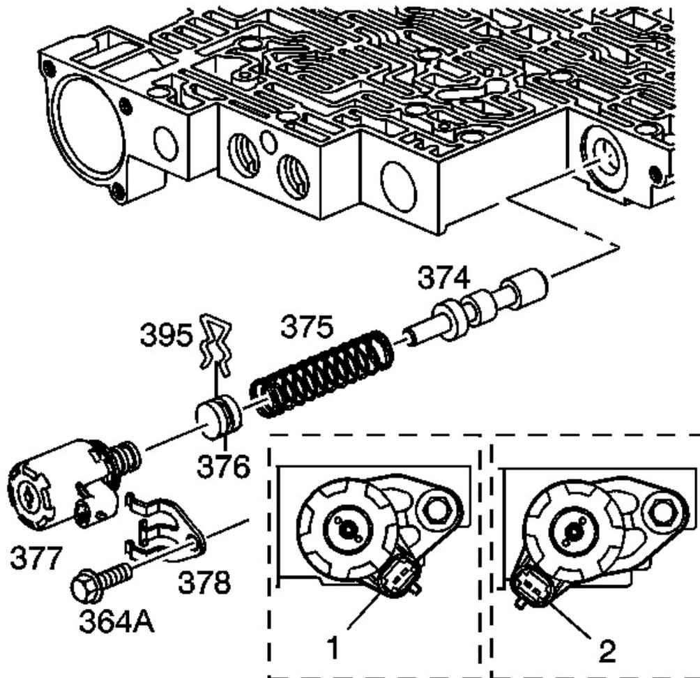
**Fig. 266: Locating Actuator Feed Limit Valve & Pressure Control Solenoid**
