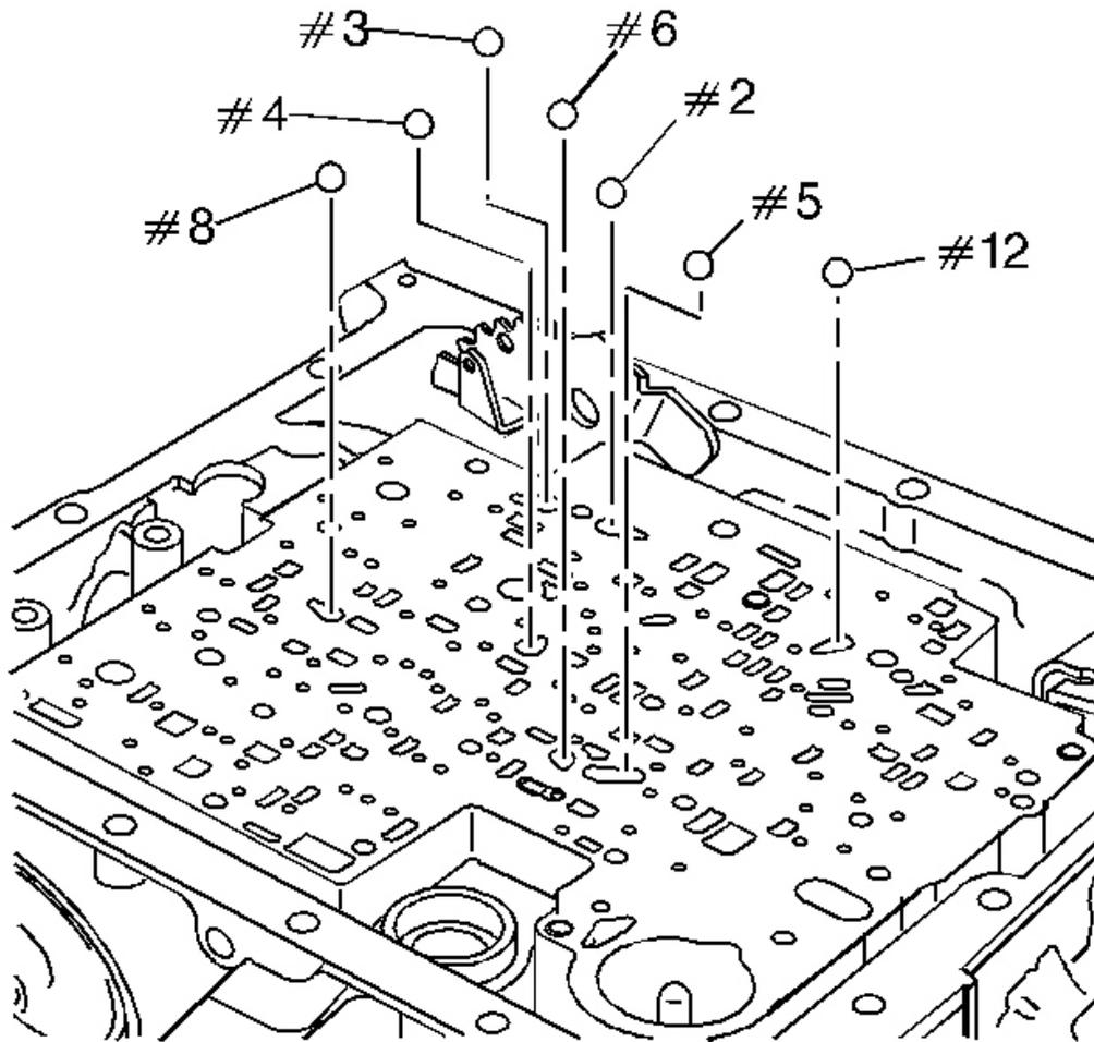
**Fig. 49: Identifying Valve Body Checkballs**
