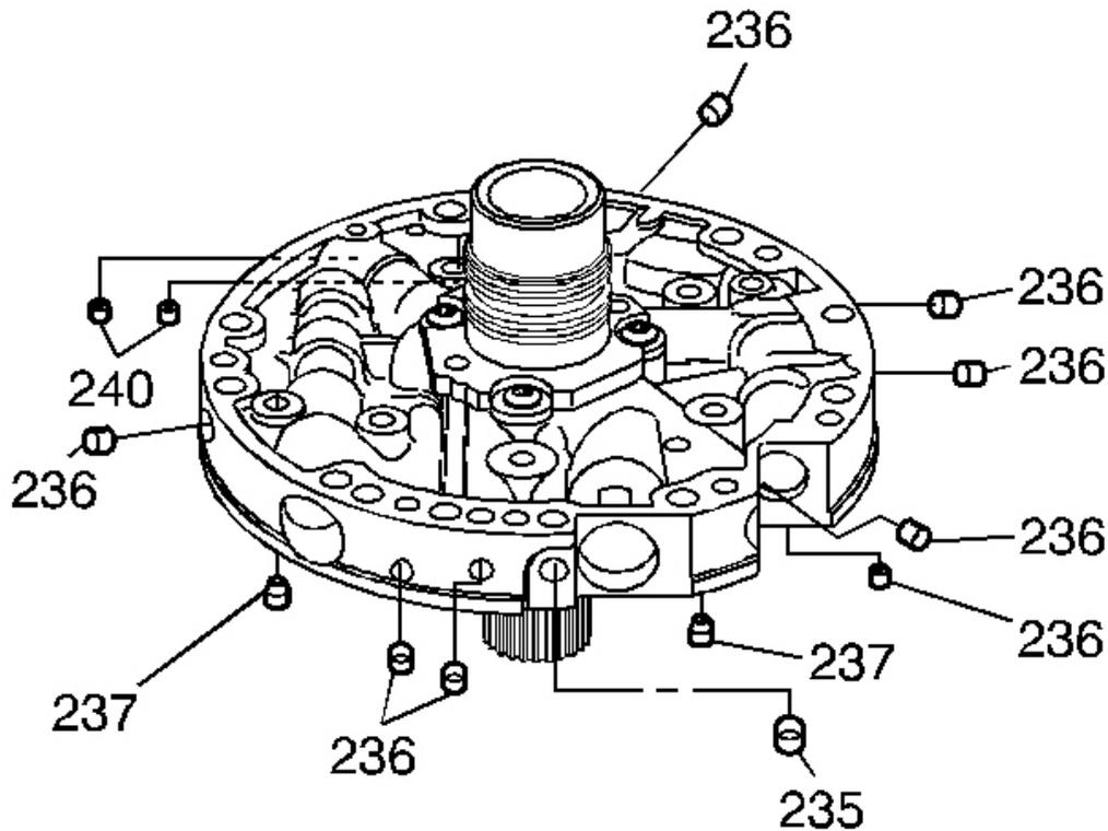
**Fig. 226: Identifying Pump Cover Components**
