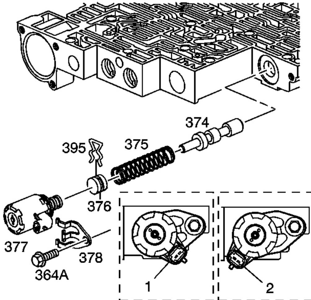
**Fig. 254: Locating Actuator Feed Limit Valve & Pressure Control Solenoid**
