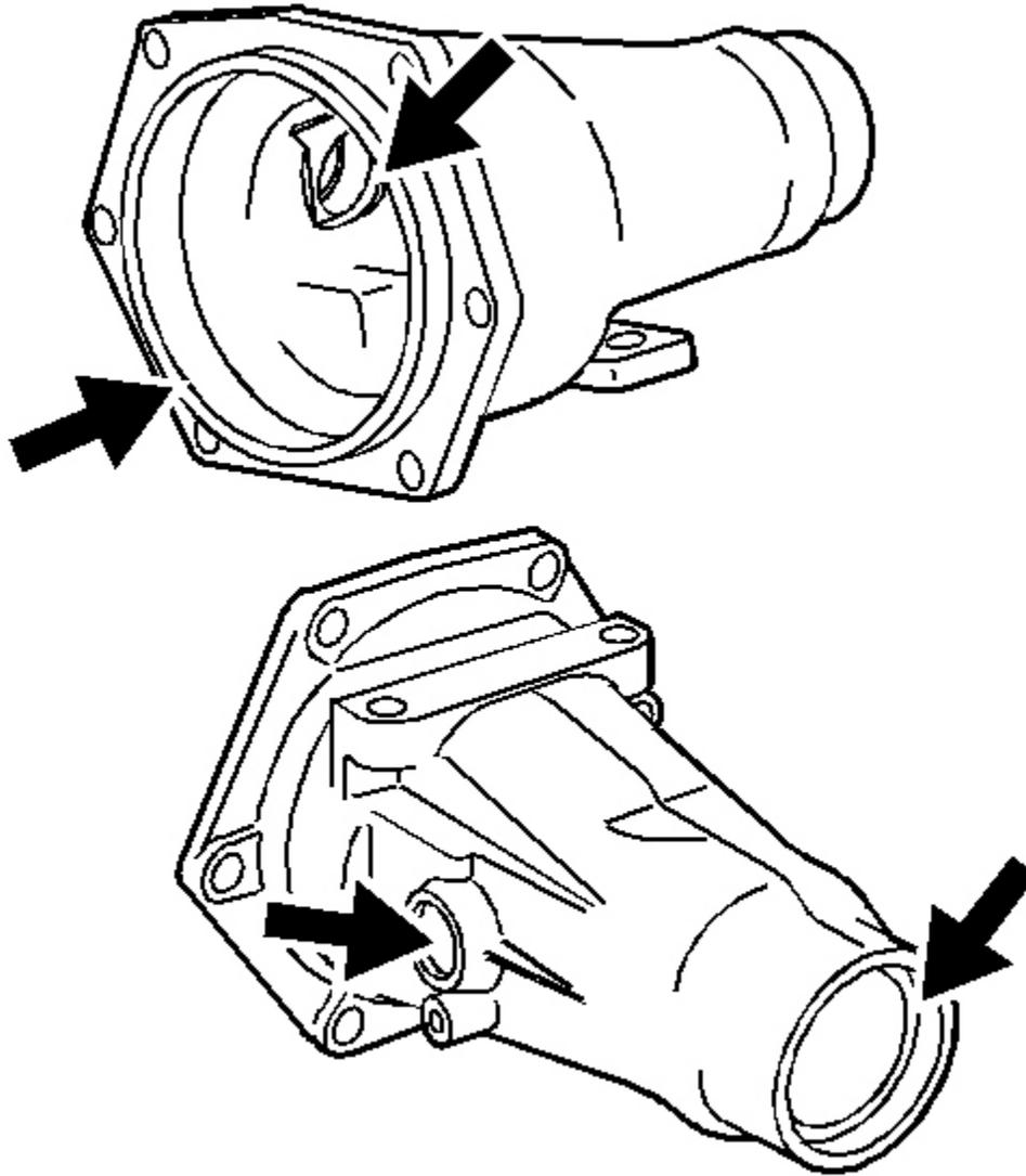
**Fig. 310: Identifying Inspection Areas On Case Extension**
