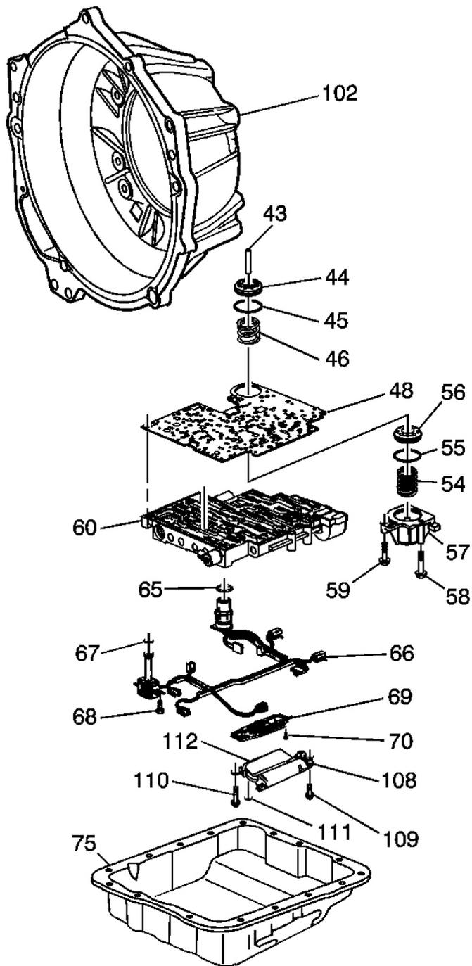
**Fig. 4: Case & Associated Parts Disassembled View (2 Of 2) - M33 Only**
