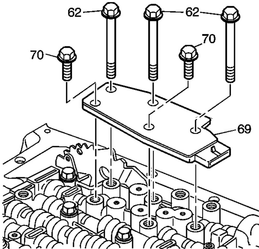
**Fig. 288: TFP Manual Valve Position Switch Retaining Bolts**
