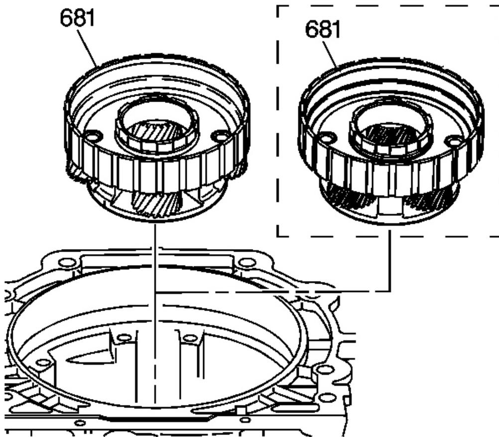
**Fig. 76: Identifying Reaction Carrier Assembly**
