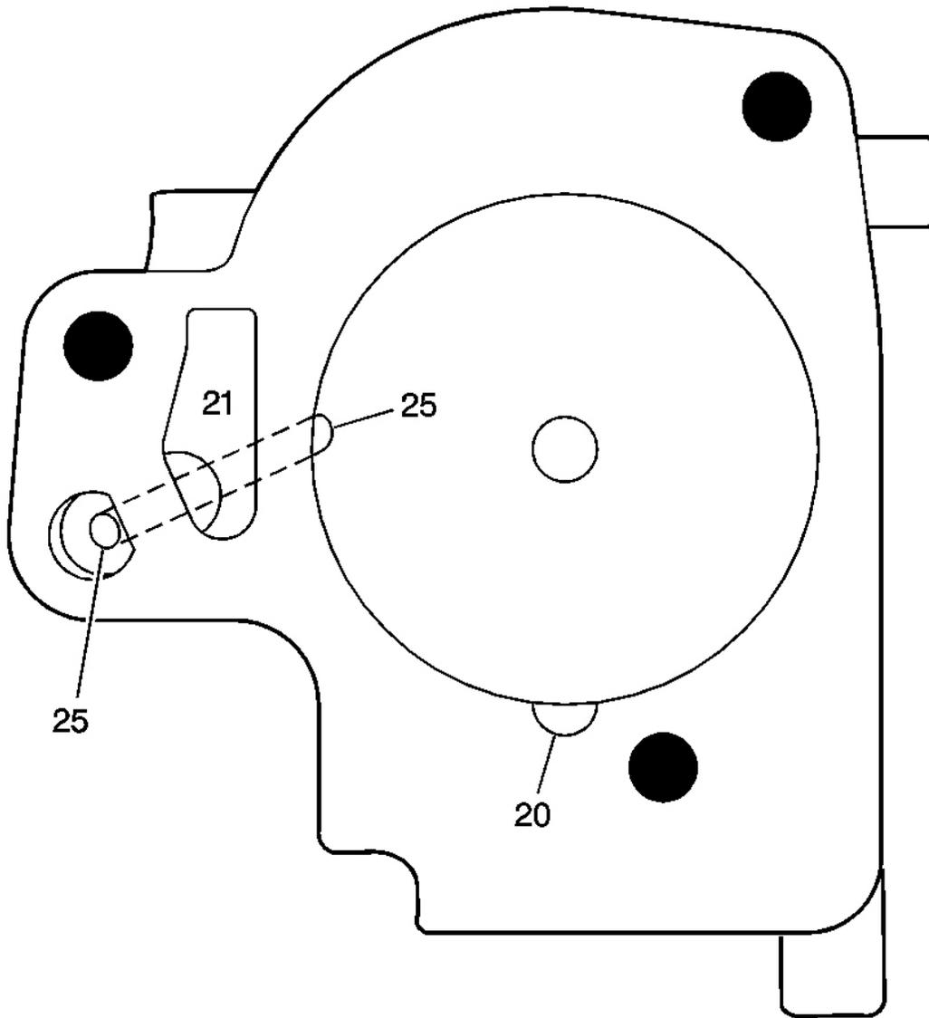
**Fig. 345: 1-2 Accumulator Cover Fluid Passages**
