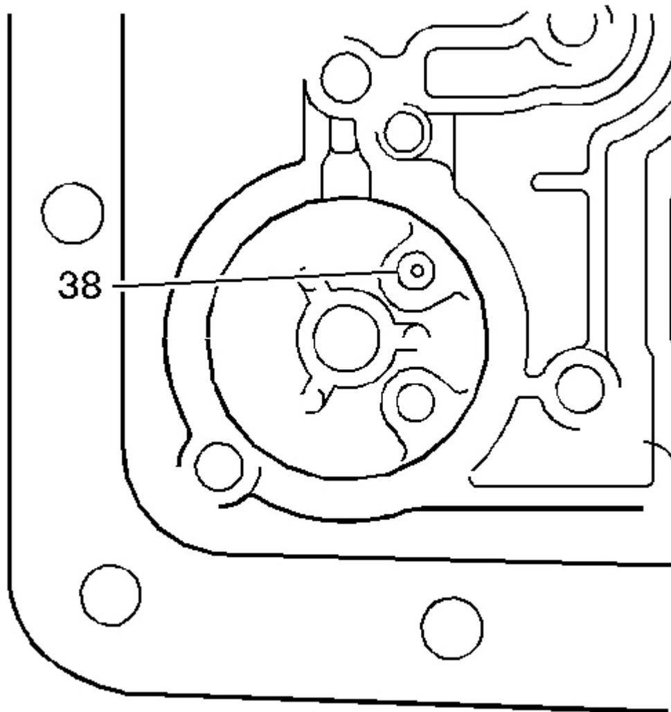
**Fig. 88: Locating Orifice Cup Plug**
