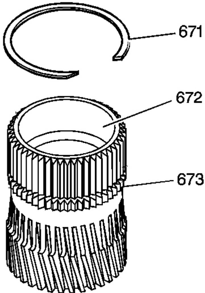
**Fig. 122: Inspection Areas On Reaction Sun Gear**
