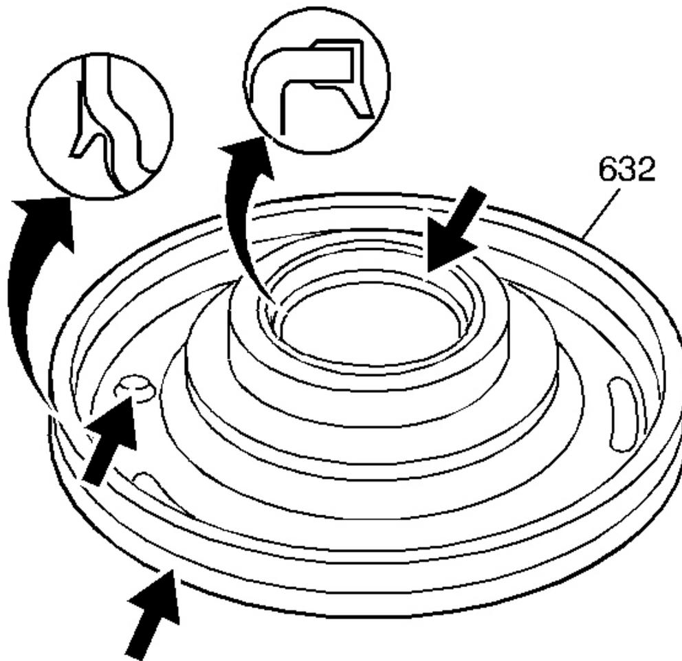
**Fig. 160: Inspection Areas On Overrun Clutch Piston**
