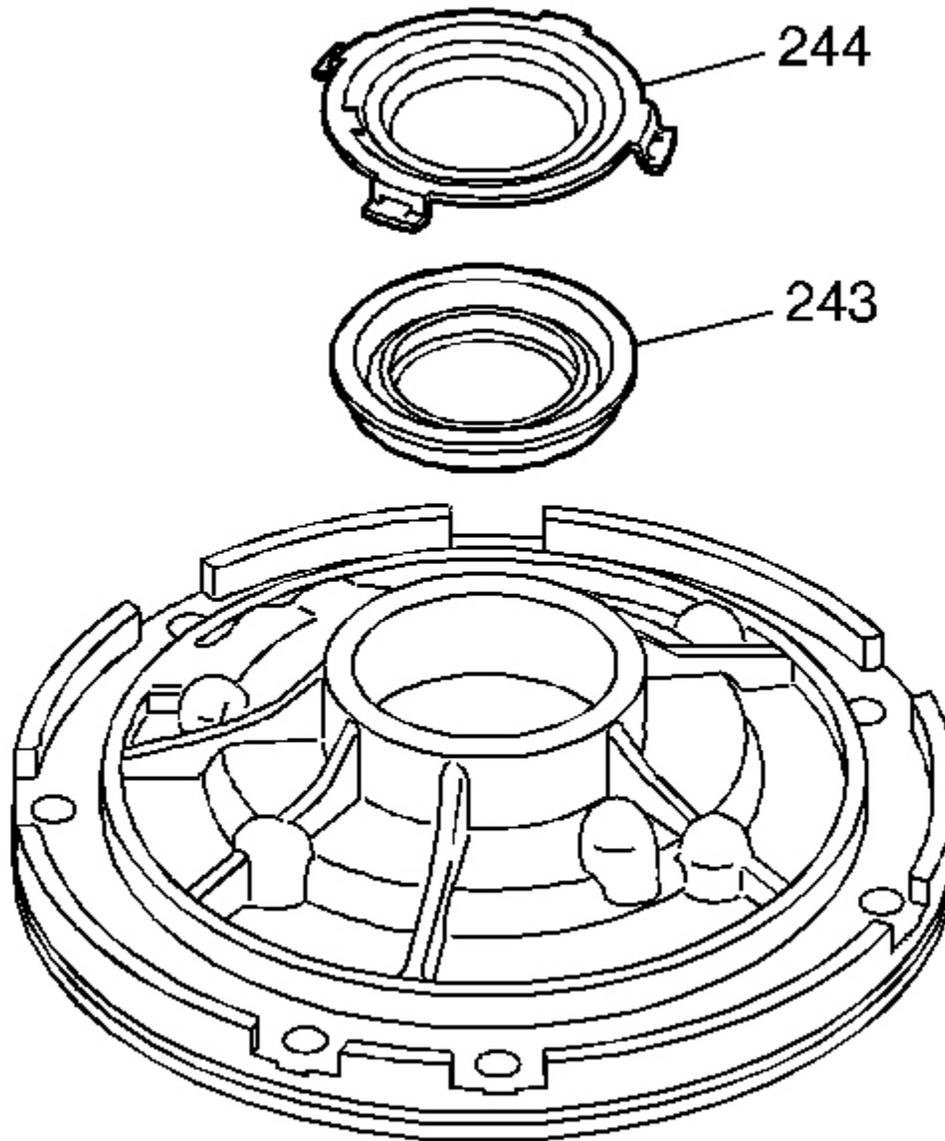
**Fig. 213: Locating Front Helix Retainer & Oil Seal Assembly**
