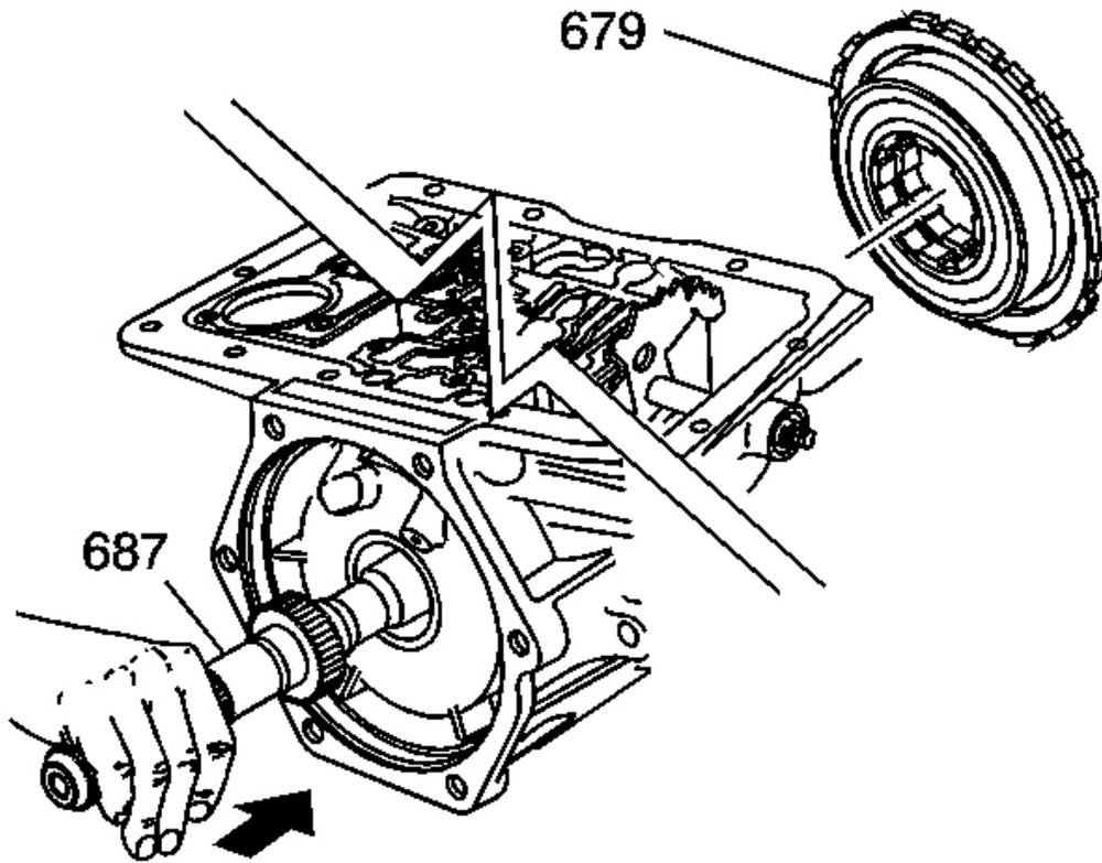
**Fig. 73: View Of Low And Reverse Clutch Support**
