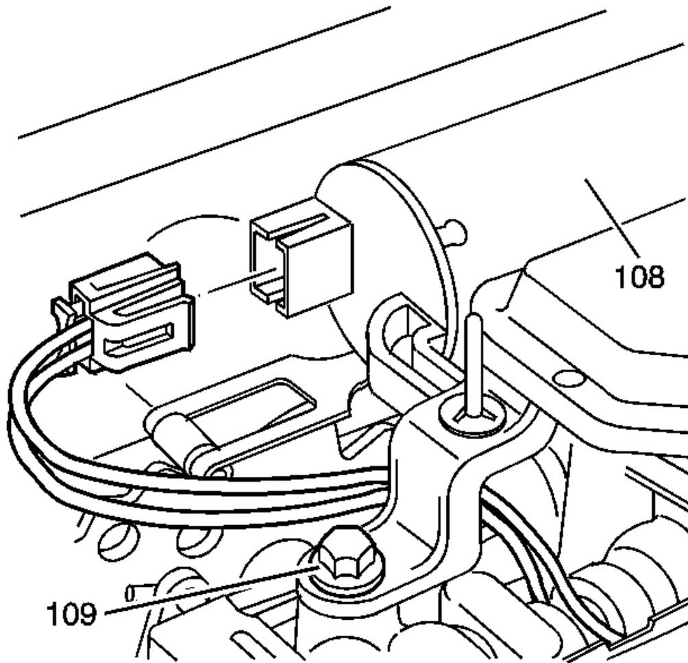
**Fig. 39: Locating Secondary Fluid Pump Electrical Connector & Retaining Bolts**
