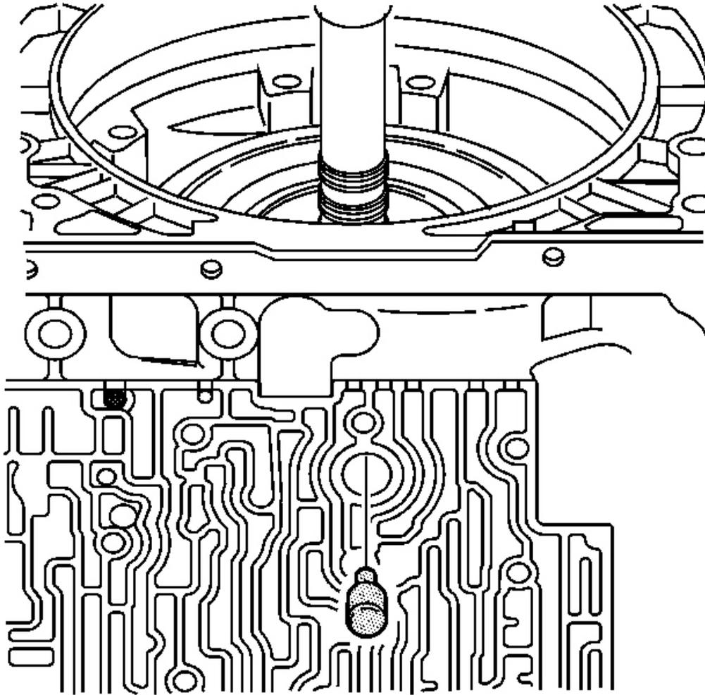
**Fig. 63: Identifying Band Anchor Pin**
