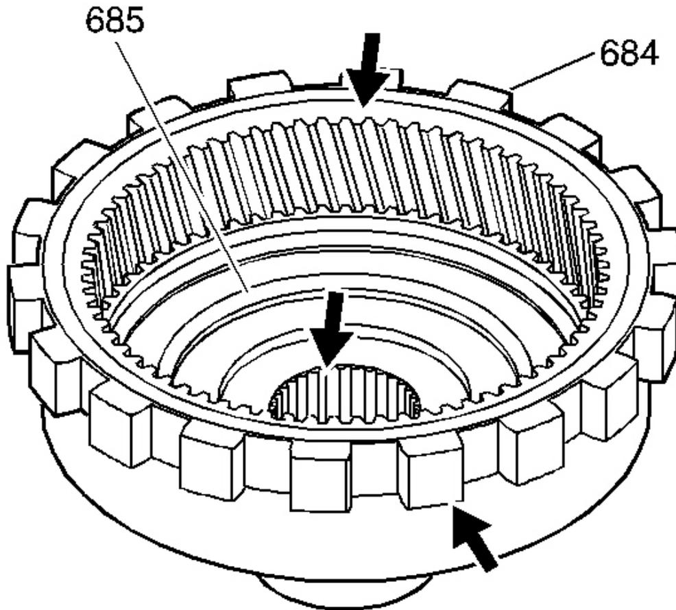
**Fig. 106: View Of Reaction Gear And Carrier Inspection Areas**
