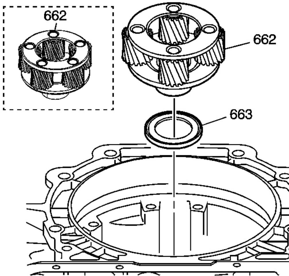
**Fig. 67: Identifying Input Carrier Assembly**
