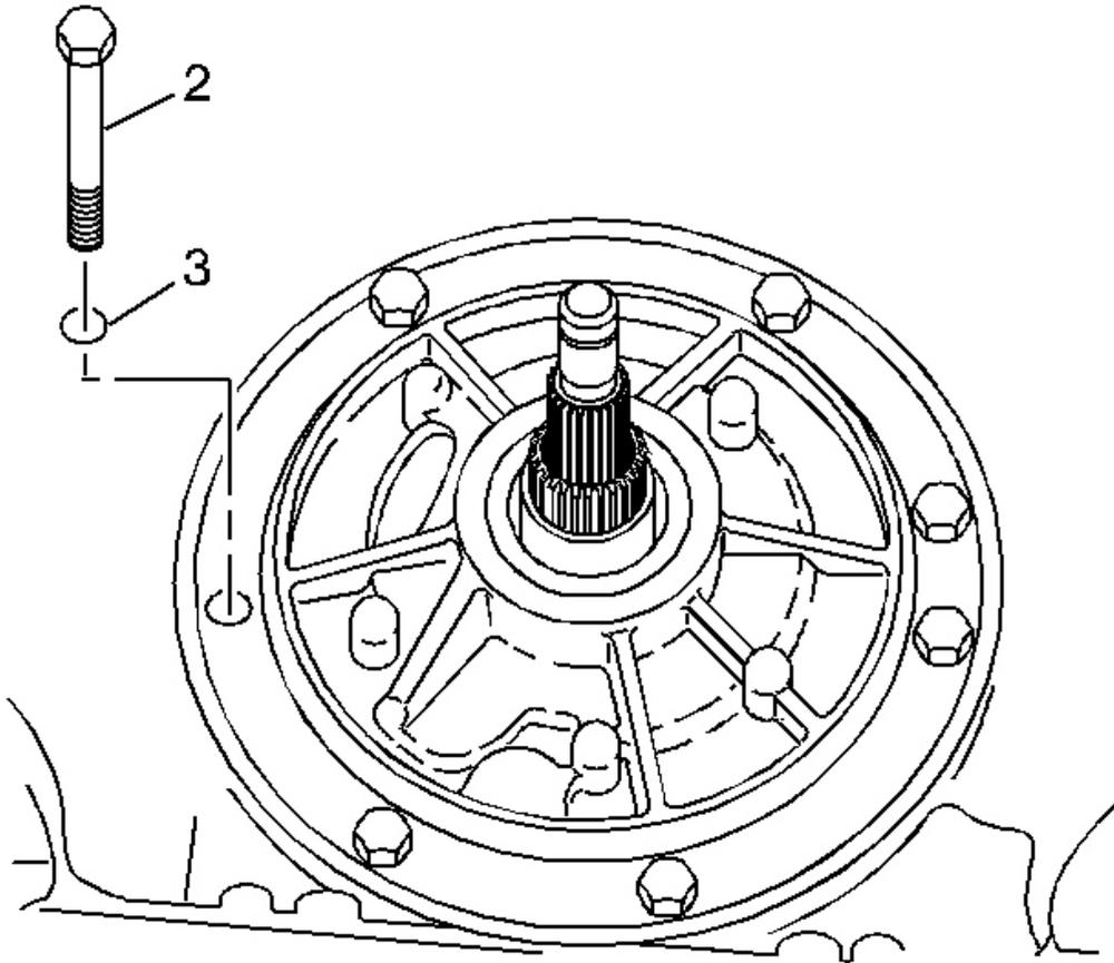
**Fig. 242: Locating Pump To Case Bolts & O-Ring Seals**
