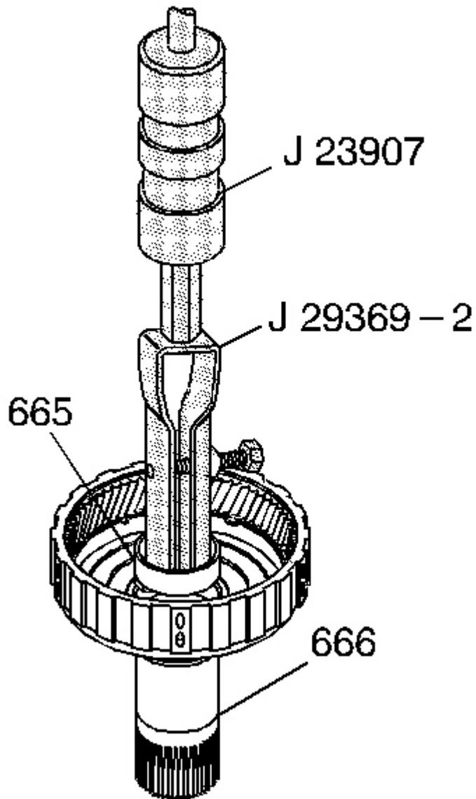
**Fig. 128: Removing Reaction Carrier Shaft Front Bushing**
