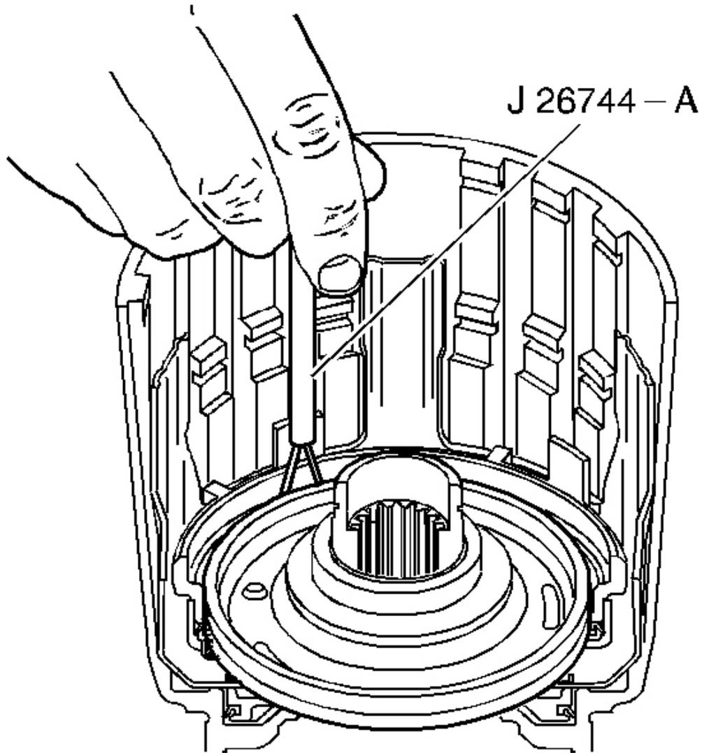
**Fig. 162: Installing Overrun Clutch Piston Outer Seal With J 26744-A**
