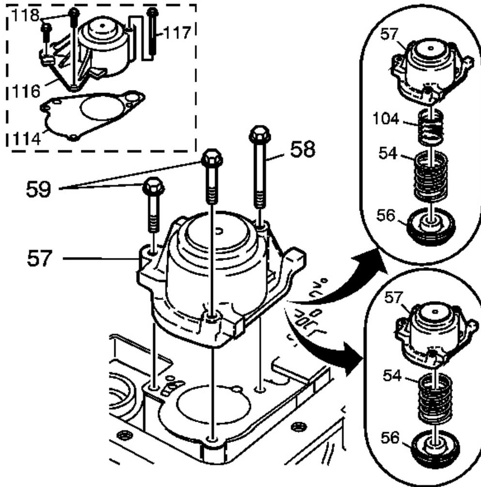
**Fig. 50: Views Of 1-2 Accumulator Assemblies**
