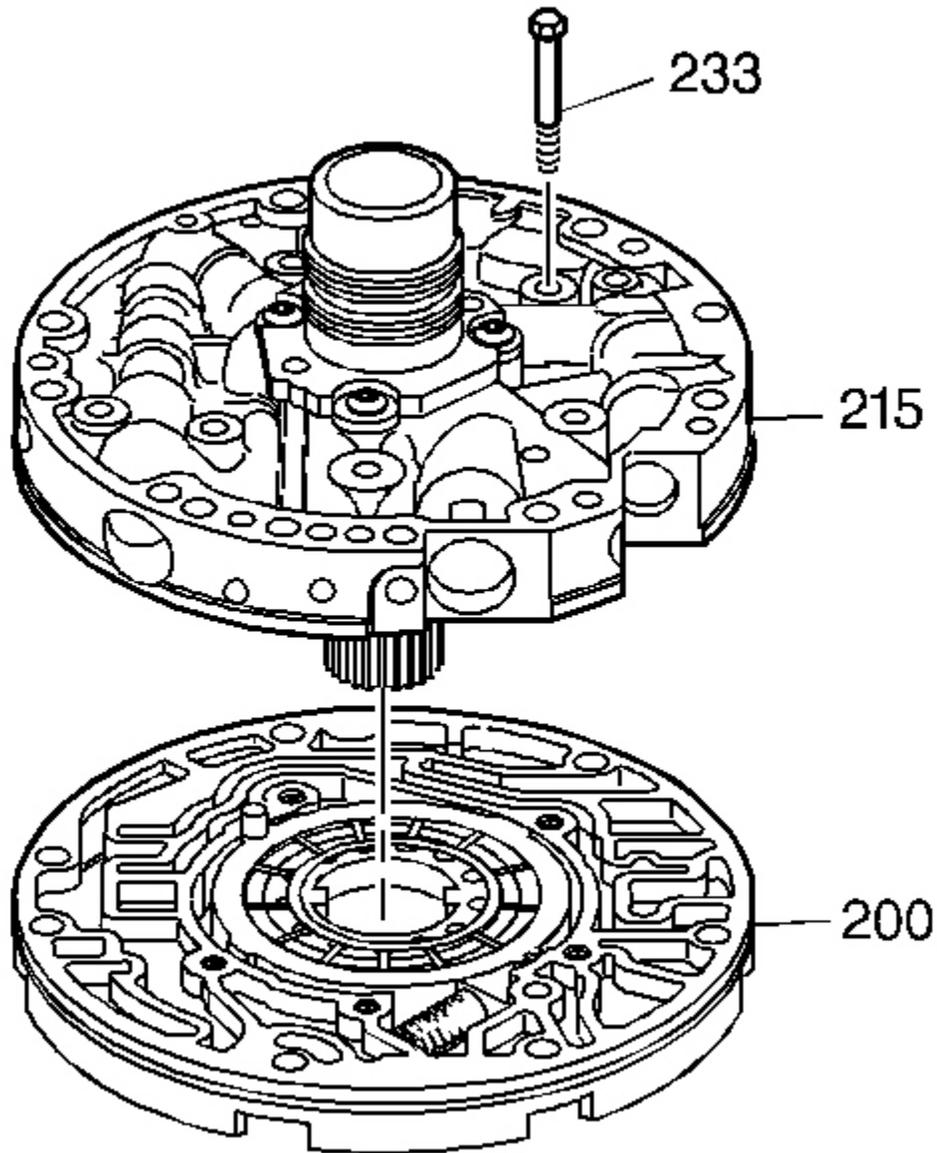
**Fig. 207: Locating Pump Cover Bolts**
