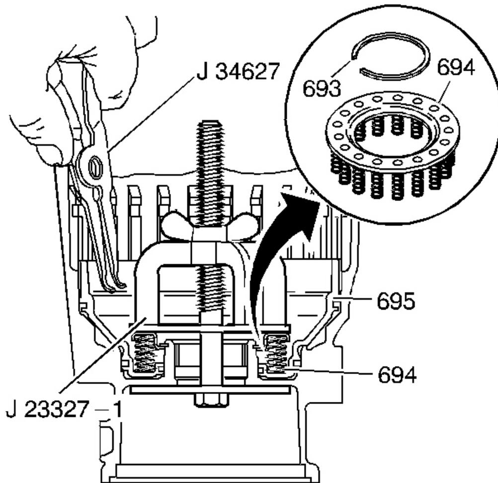
**Fig. 83: View Of Low And Reverse Clutch Spring Assembly & Retainer Ring**
