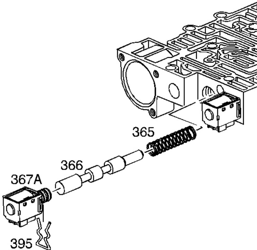
**Fig. 251: Locating 1-2 Shift Valve & Solenoid Components**
