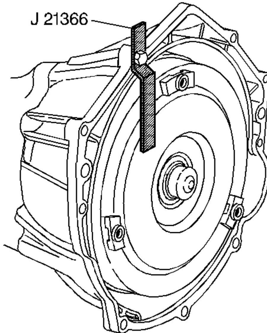
**Fig. 320: View Of J 21366 Installed On Torque Converter**
