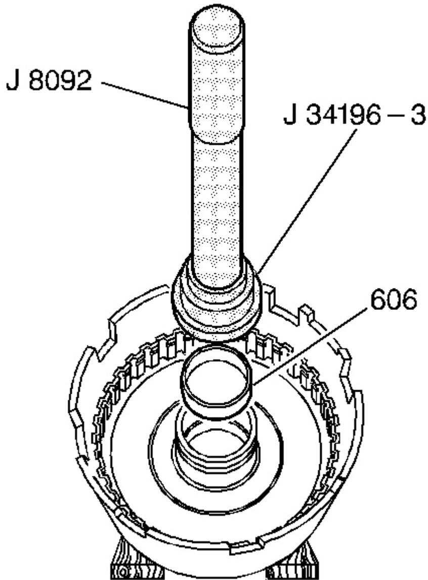
**Fig. 194: Installing Reverse Input Clutch Rear Bushing**
