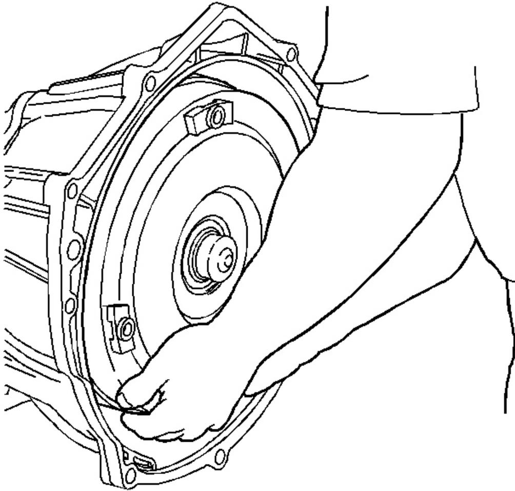
**Fig. 23: Removing Torque Converter**
