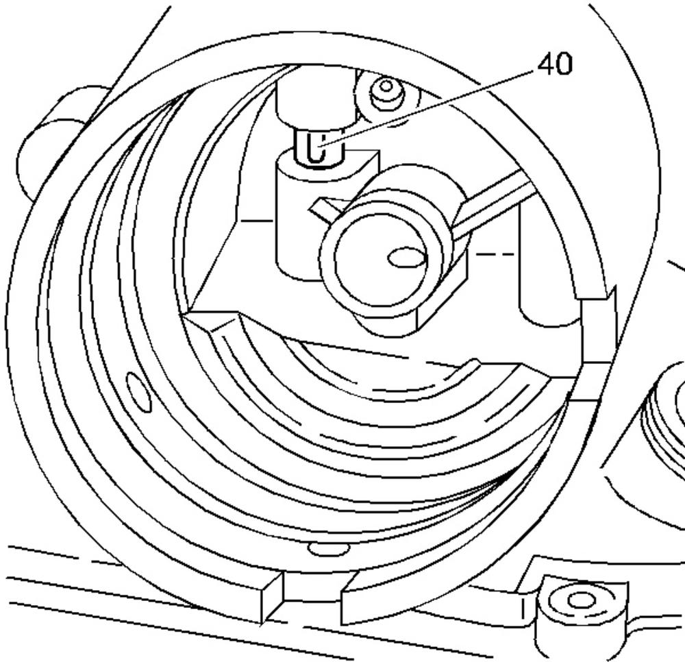
**Fig. 96: Aligning Third Accumulator Retainer And Ball Assembly With Retainer Slot**
