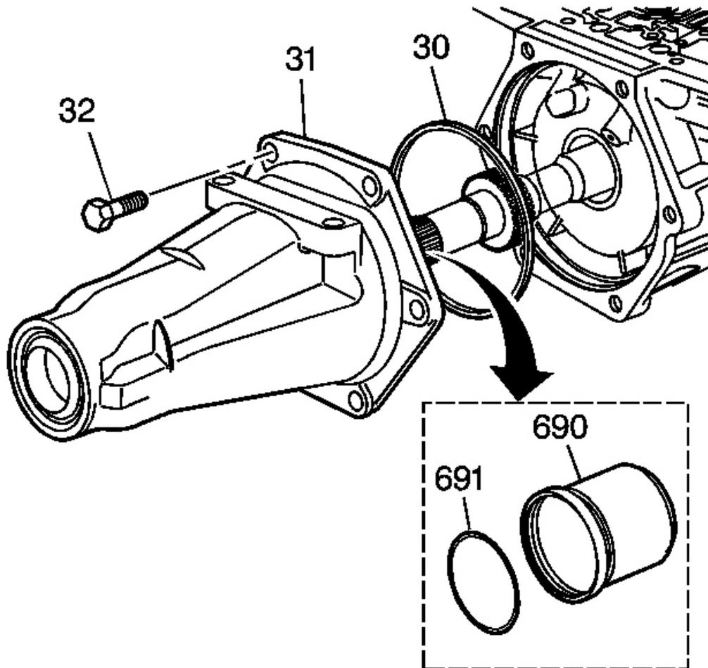
**Fig. 34: Identifying Output Shaft Components**
