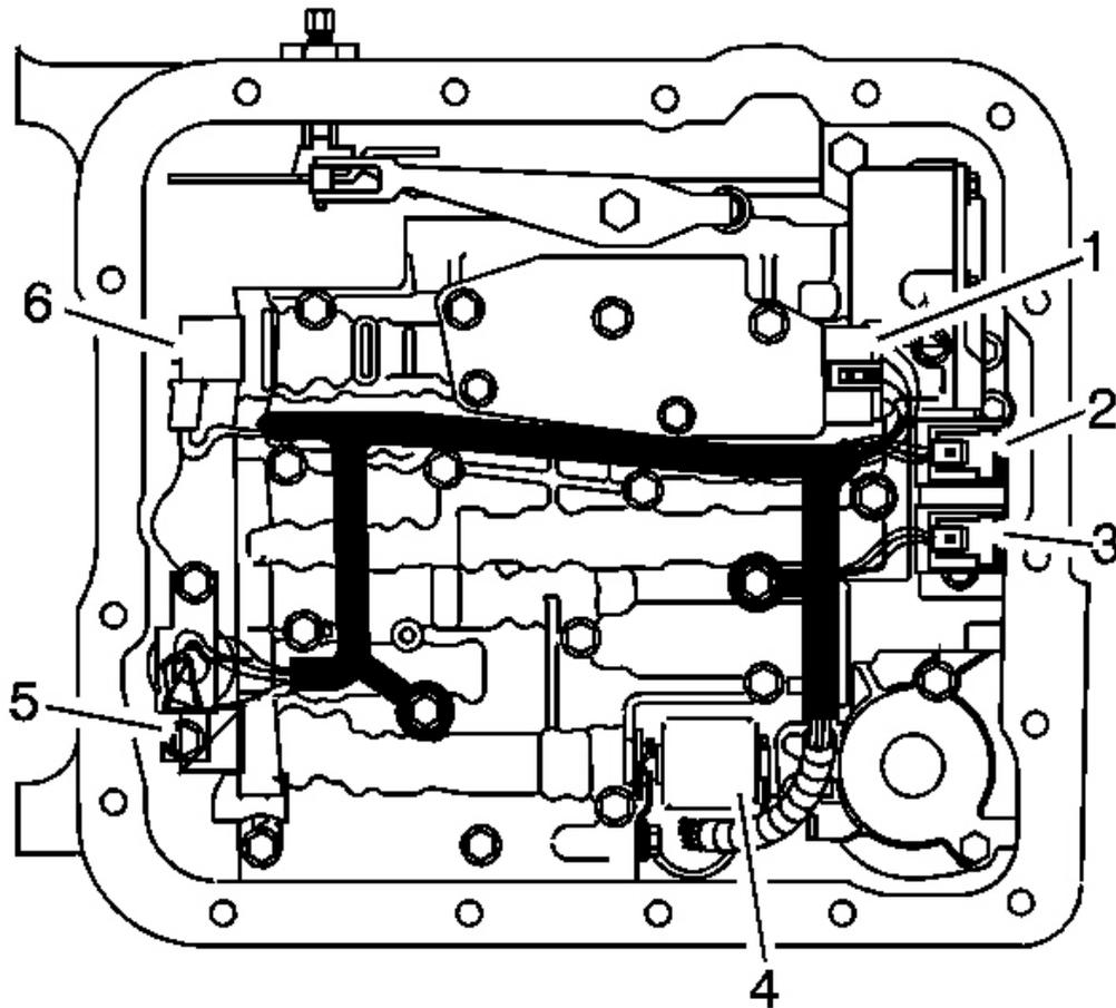
**Fig. 292: Identifying Electrical Components In Valve Body**
