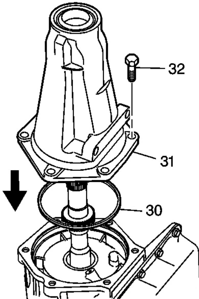
**Fig. 315: Locating Case Extension Case Seal**
