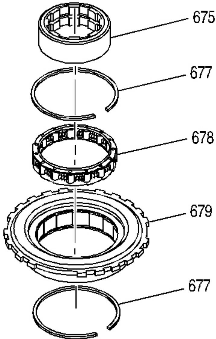
**Fig. 116: Low and Reverse Clutch Support Components**
