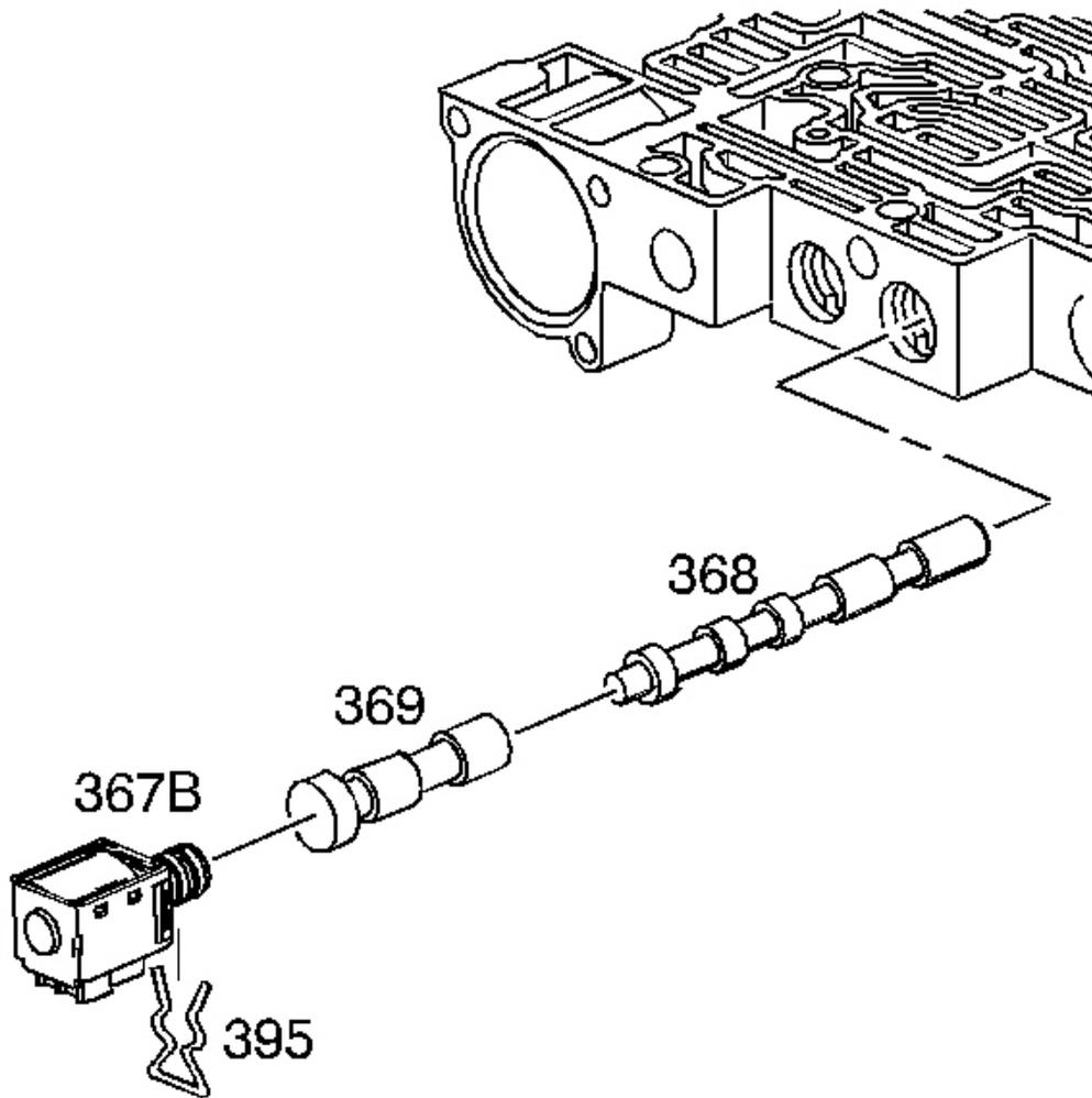
**Fig. 252: Identifying 2-3 Shuttle Valve & Solenoid Components**
