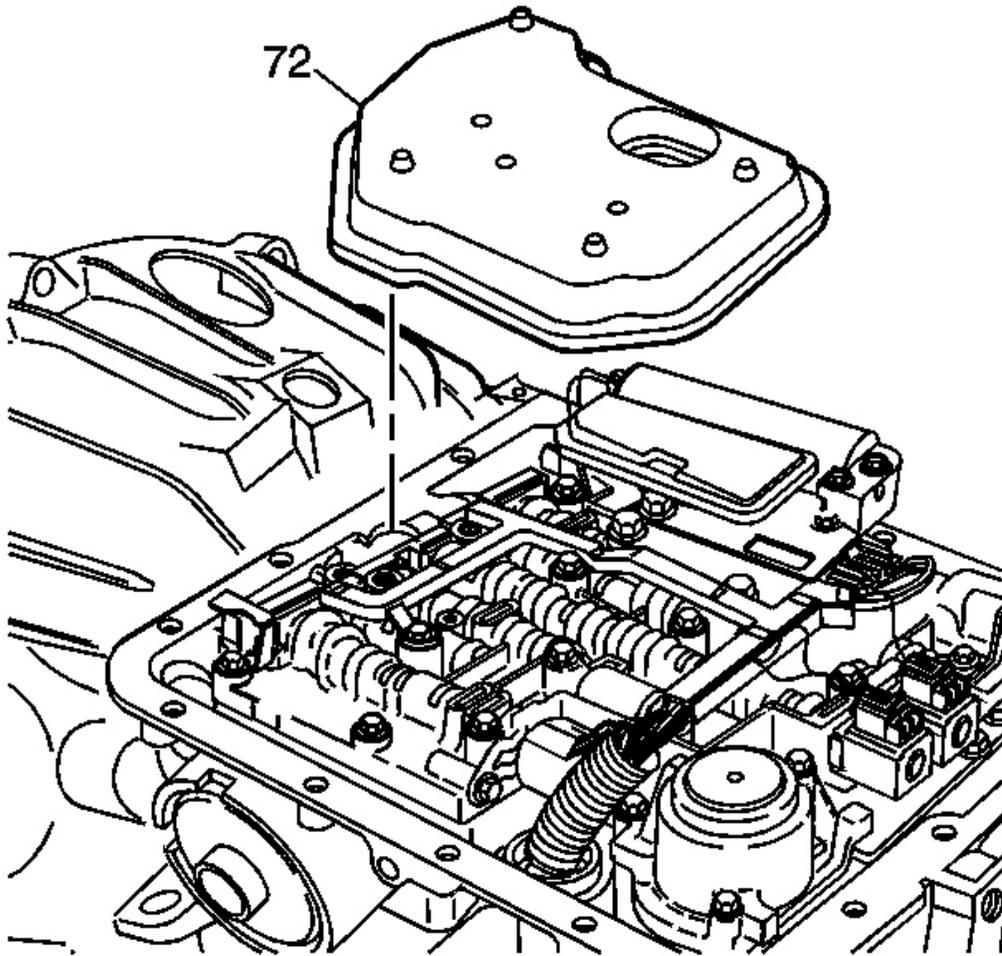
**Fig. 297: View Of Transmission Oil Filter Assembly**
