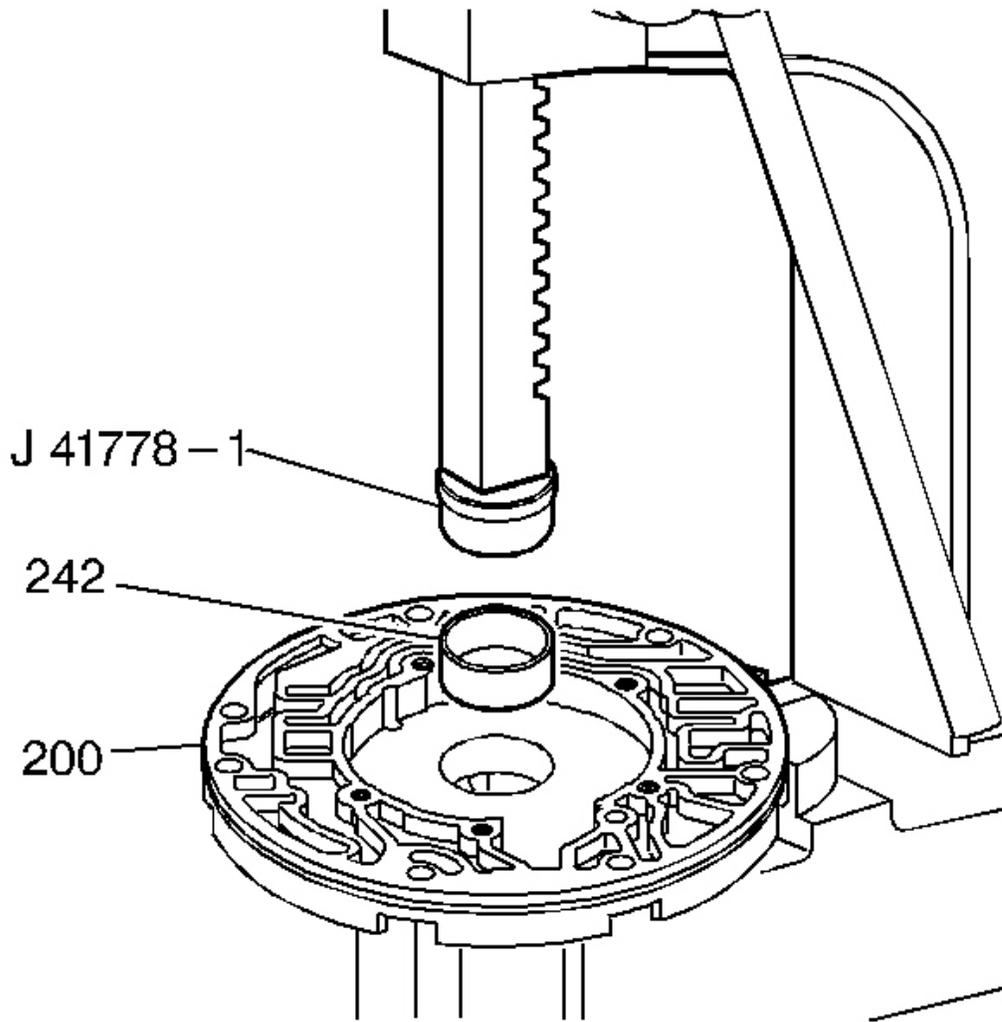
**Fig. 215: Pressing In Pump Body Bushing**
