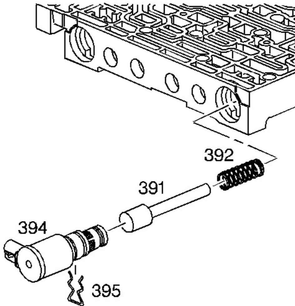
**Fig. 255: Identifying 3-2 Control Valve & 3-2 Control Solenoid**
