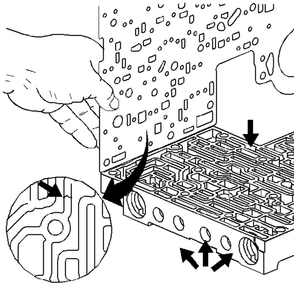
**Fig. 260: Inspecting Control Valve Body For Channel Witness Marks**
