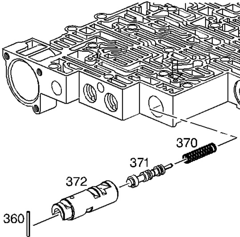
**Fig. 267: View Of 1-2 Accumulator Valve & 1-2 Accumulator Valve Sleeve**
