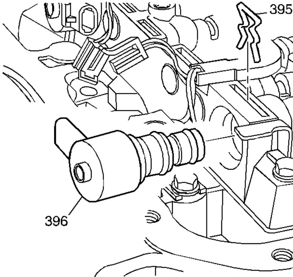
**Fig. 42: Removing TCC/PWM Solenoid & Clip**
