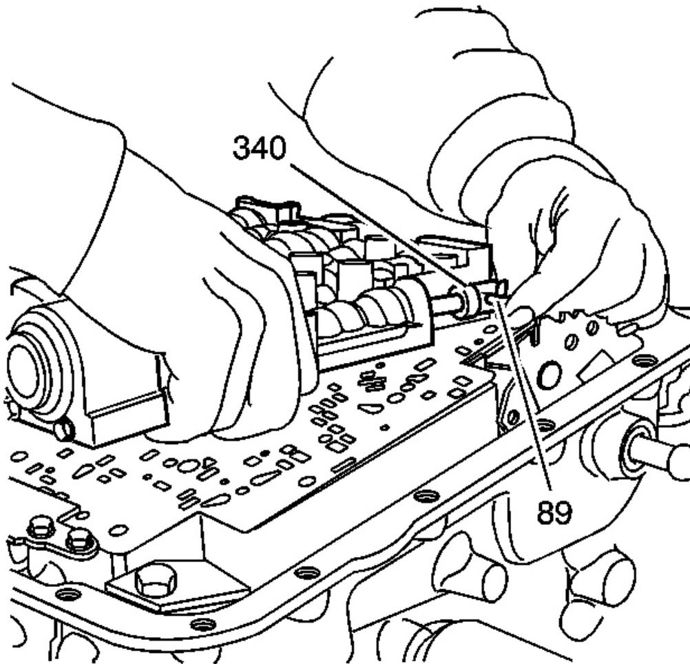
**Fig. 48: Disconnecting Manual Valve Link**
