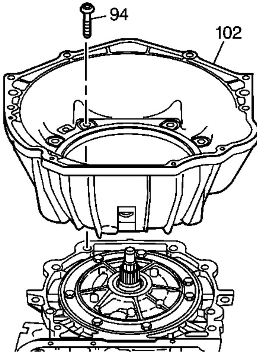
**Fig. 25: View Of Converter Housing Bolts**
