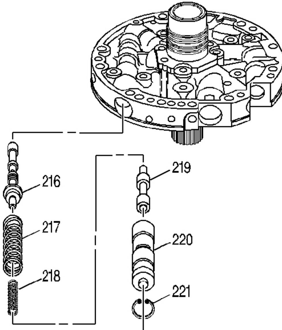
**Fig. 222: View Of Reverse Boost Valve & Pressure Regulator Components**
