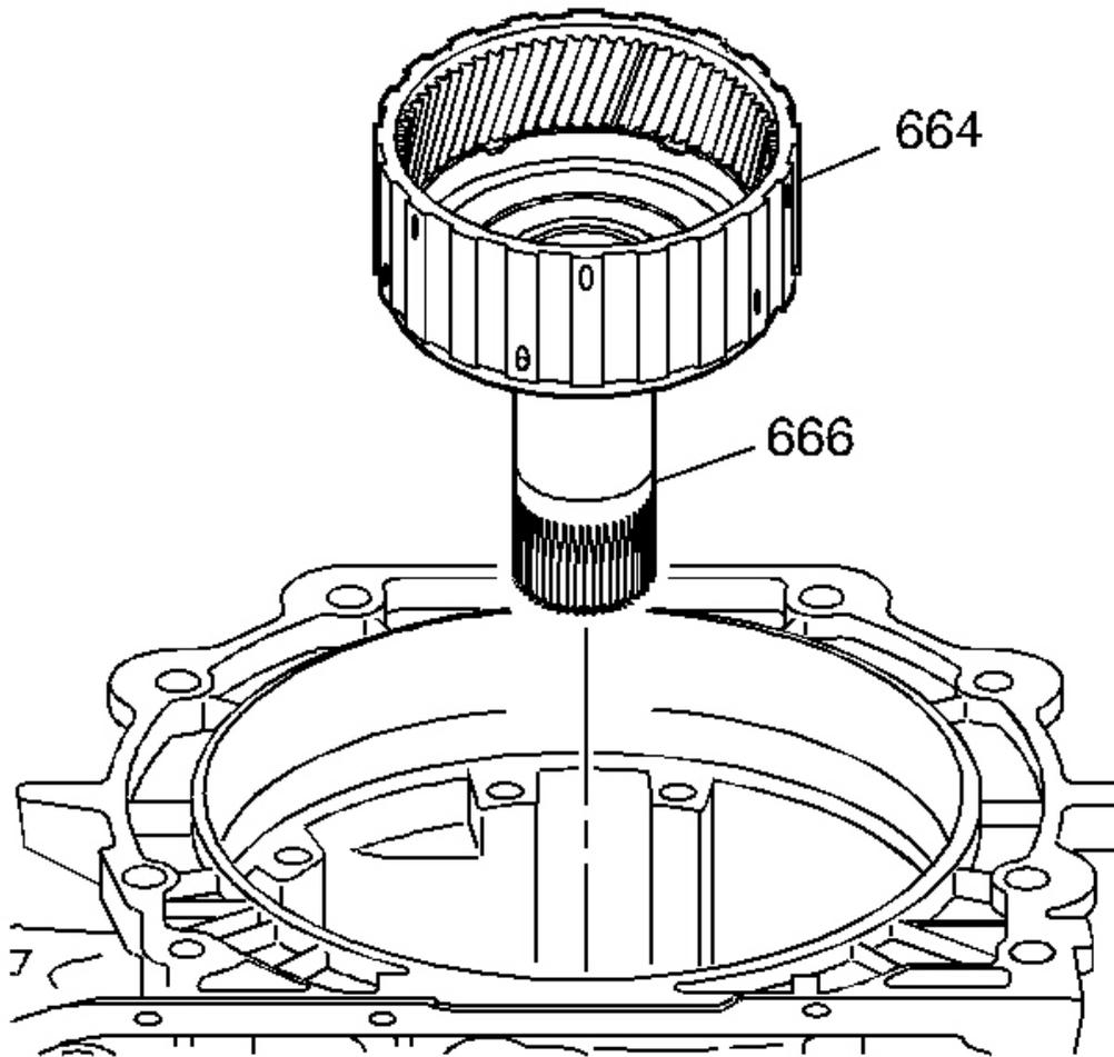
**Fig. 68: Reaction Carrier Shaft Assembly & Input Internal Gear**
