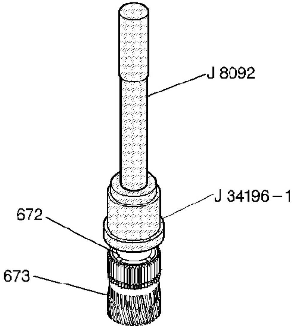
**Fig. 124: Installing Reaction Sun Bushing**
