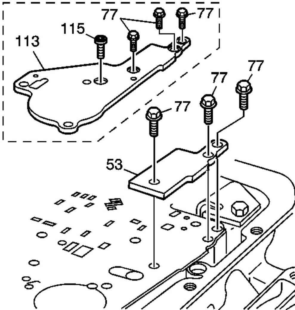
**Fig. 51: View Of Spacer Plate Support Plate & Bolts**
