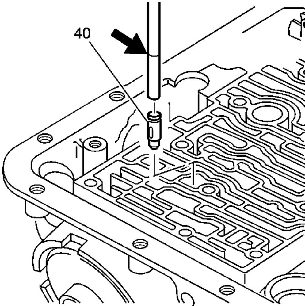
**Fig. 94: Installing Third Accumulator Retainer And Ball Assembly**
