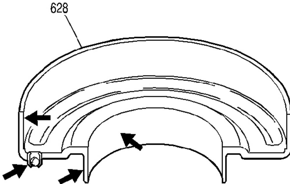
**Fig. 155: Forward Clutch Housing Inspection Areas**
