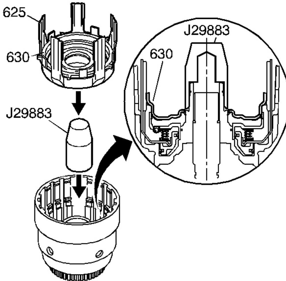
**Fig. 159: View Of J 29883 Installed In Input Housing**
