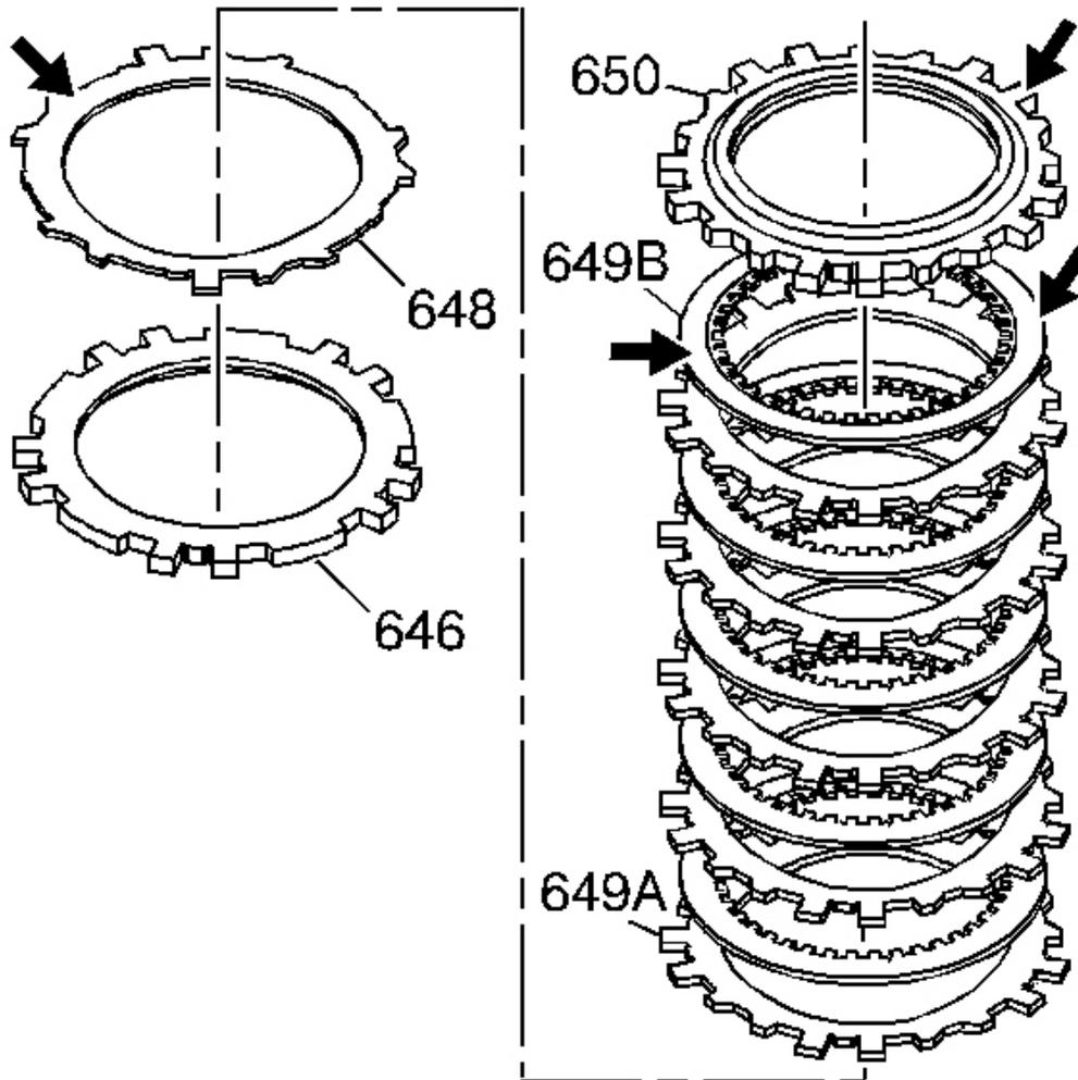
**Fig. 176: Inspecting Forward Clutch Assembly For Wear Or Damage**
