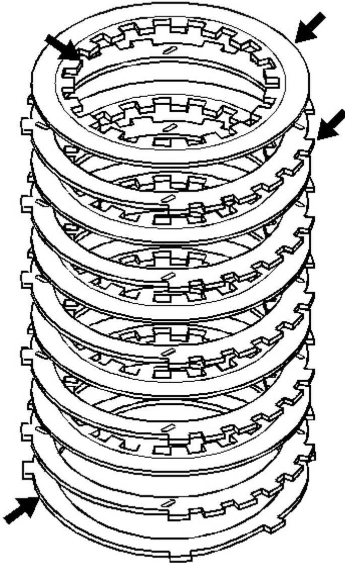
**Fig. 111: Locating Inspection Areas On Low And Reverse Clutch Plates**
