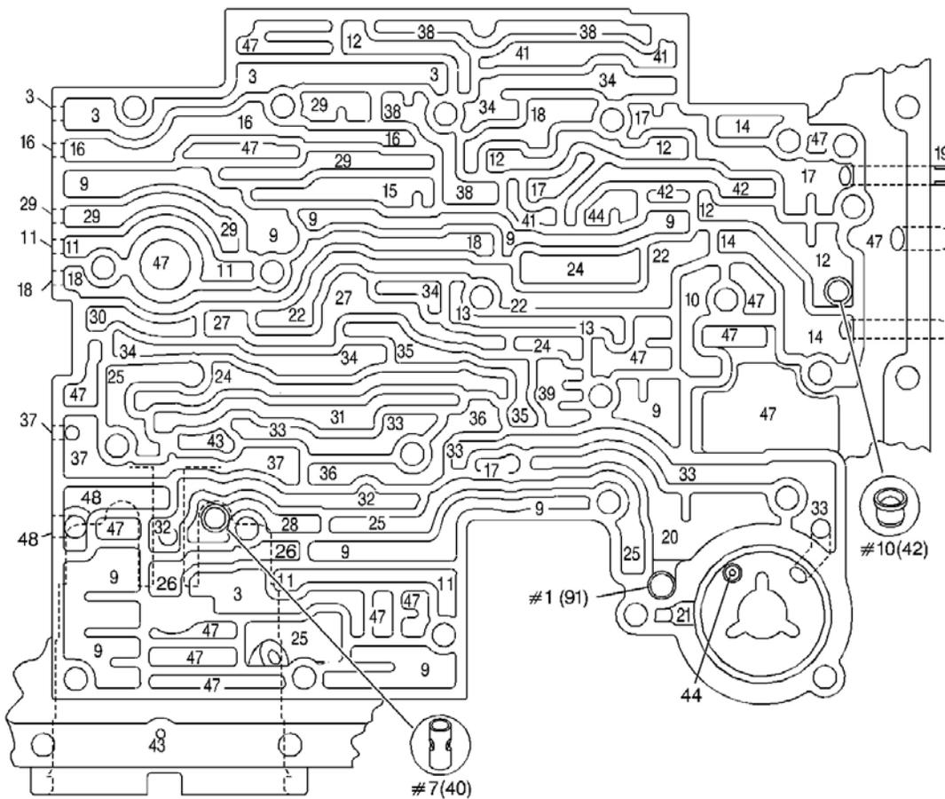
**Fig. 339: Case Fluid Passages (Control Valve Body Side)**
