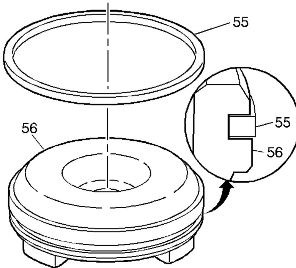
**Fig. 275: Inspecting 1-2 Accumulator Piston**
