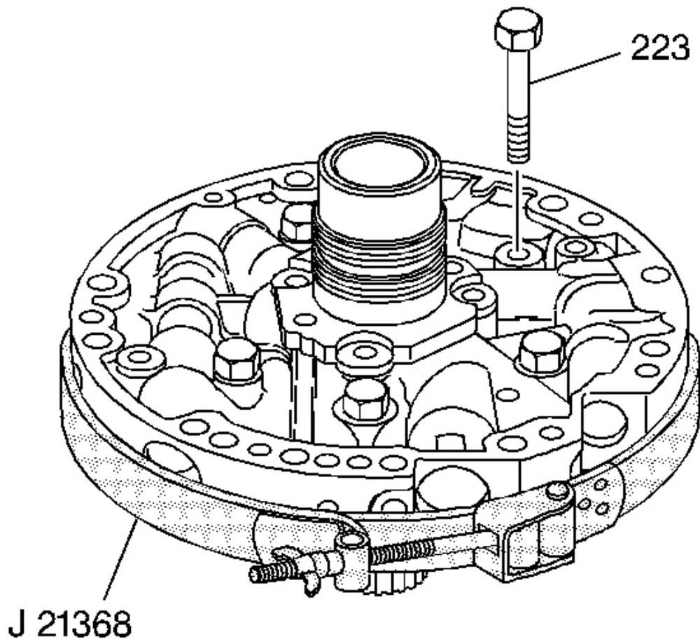
**Fig. 236: Locating Pump Cover Bolts**
