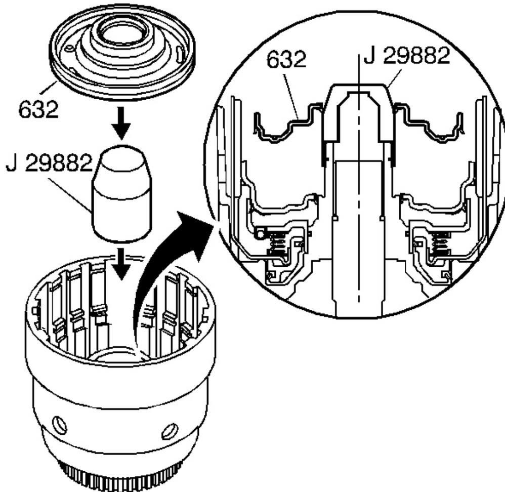
**Fig. 161: Identifying Overrun Clutch Piston**
