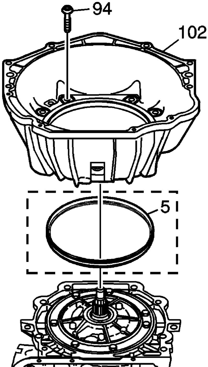
**Fig. 247: Locating Oil Pump Seal**
