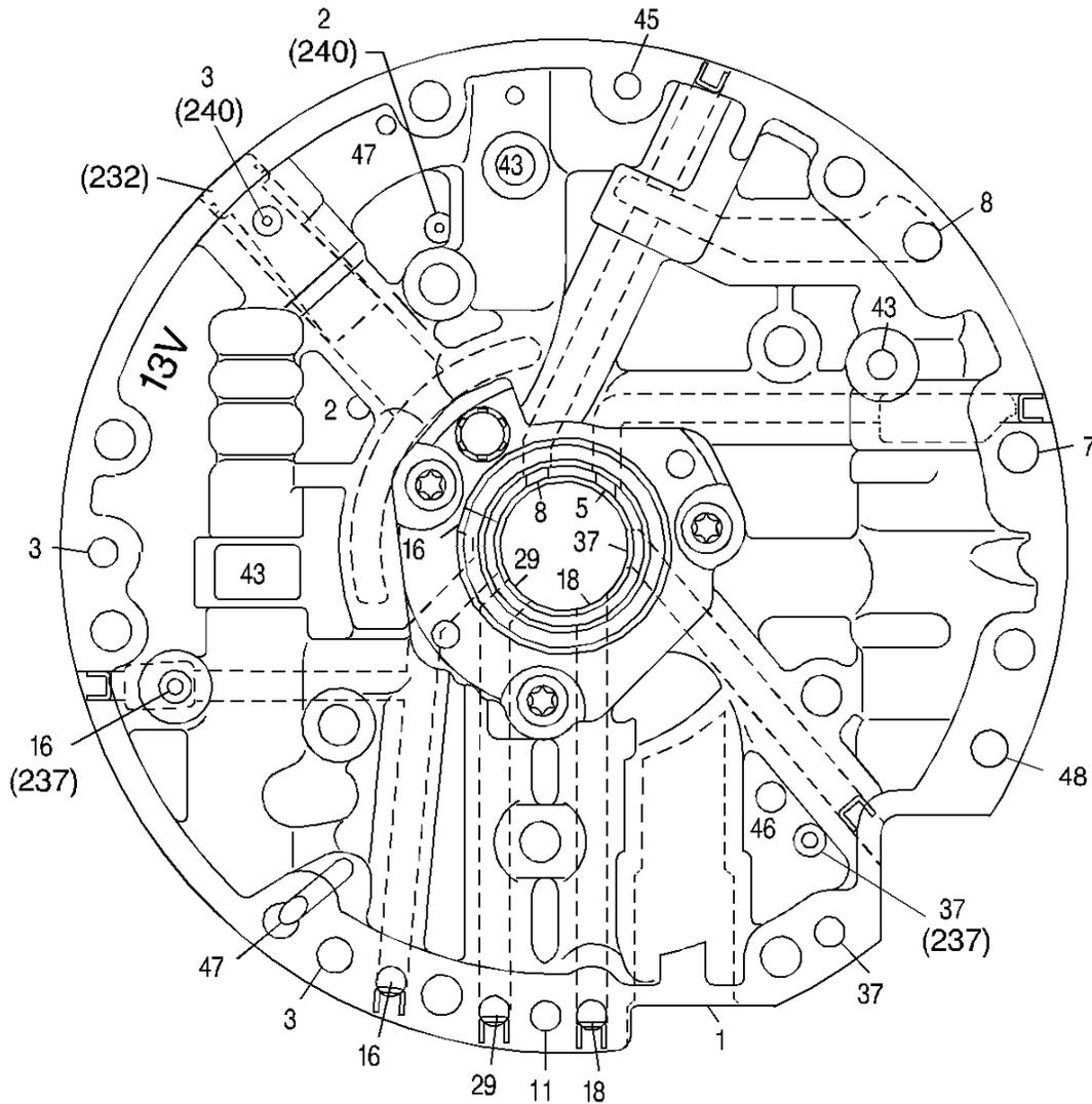
**Fig. 337: Pump Cover Fluid Passages (Case Side)**
