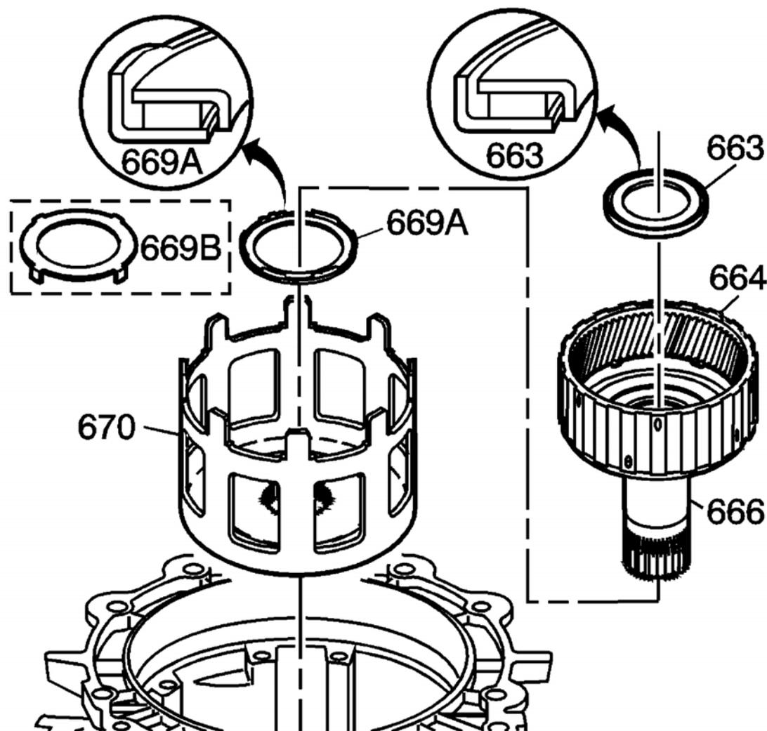
**Fig. 132: Installing Reaction Sun Shell Into Reaction Sun Gear**
