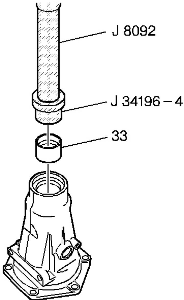
**Fig. 313: Installing Case Extension Bushing**
