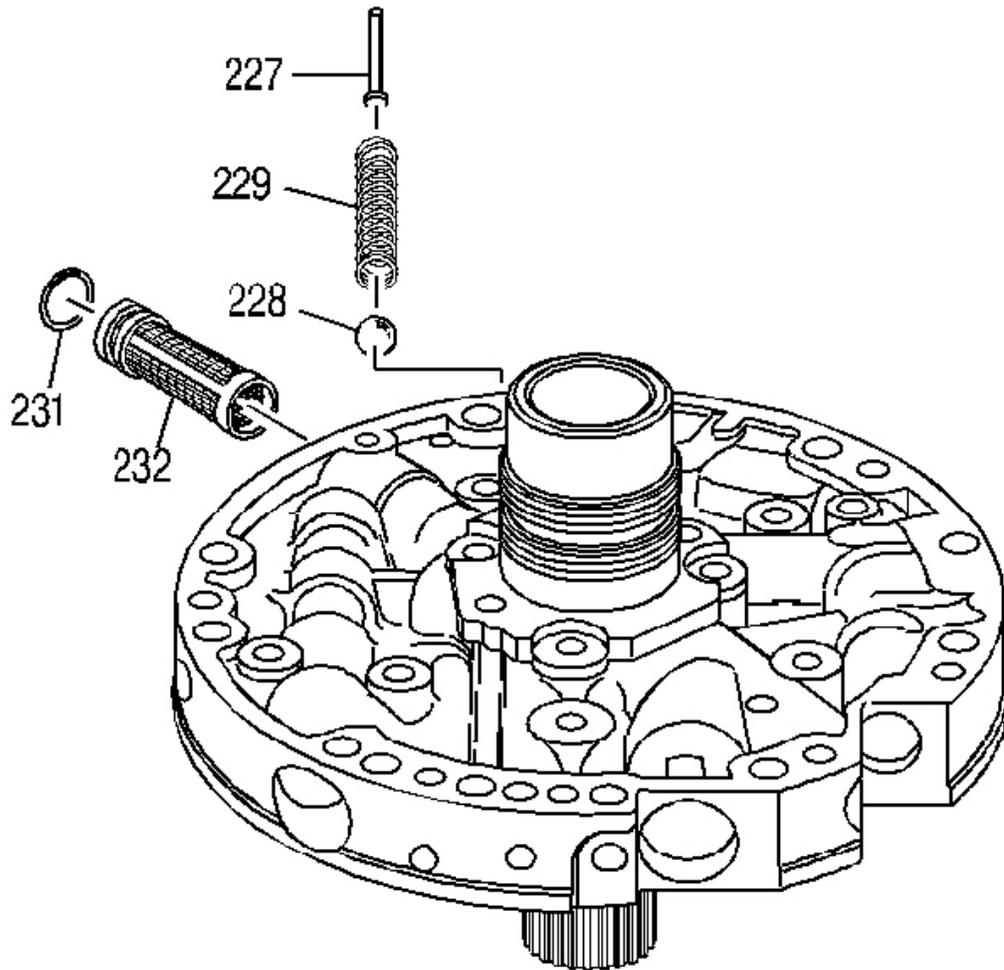
**Fig. 224: Removing Oil Pump Cover Screen & Pressure Relief Components**
