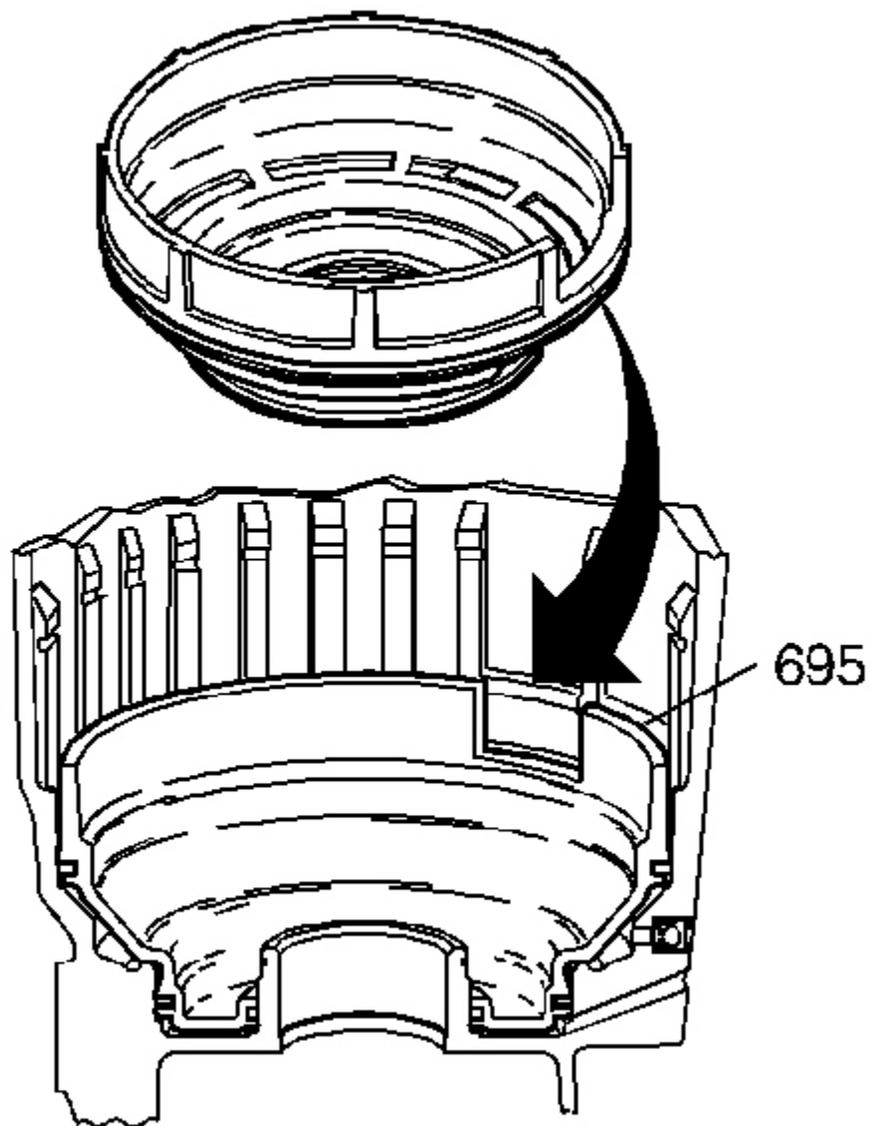
**Fig. 101: Aligning Parking Brake Pawl Window With Notch In Piston**
