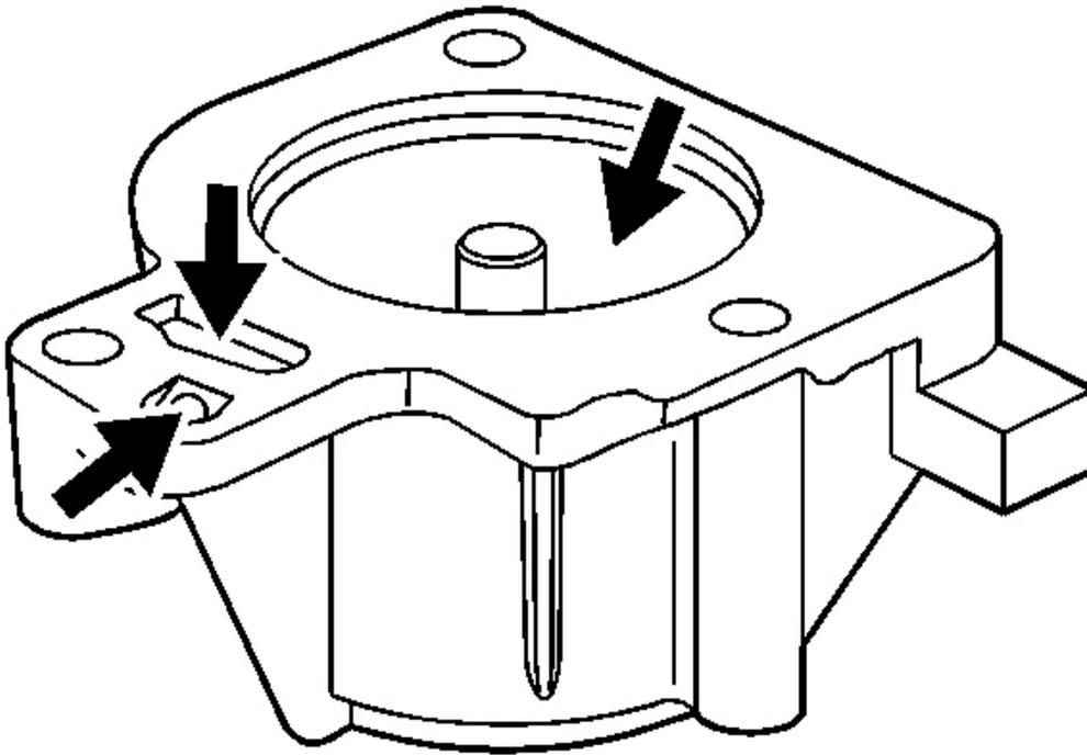
**Fig. 276: Locating 1-2 Accumulator Housing Inspection Areas**
