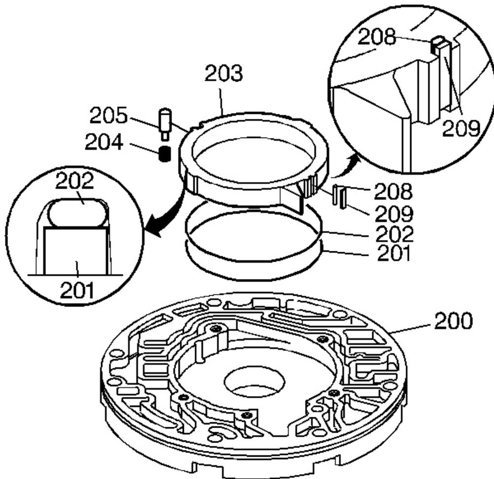
**Fig. 219: Identifying Pump Slide Components**
