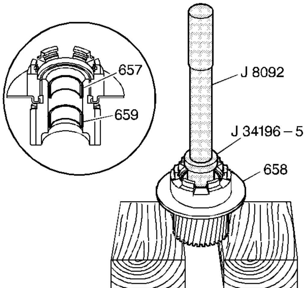
**Fig. 139: Removing Input Sun Gear Front Bushing**
