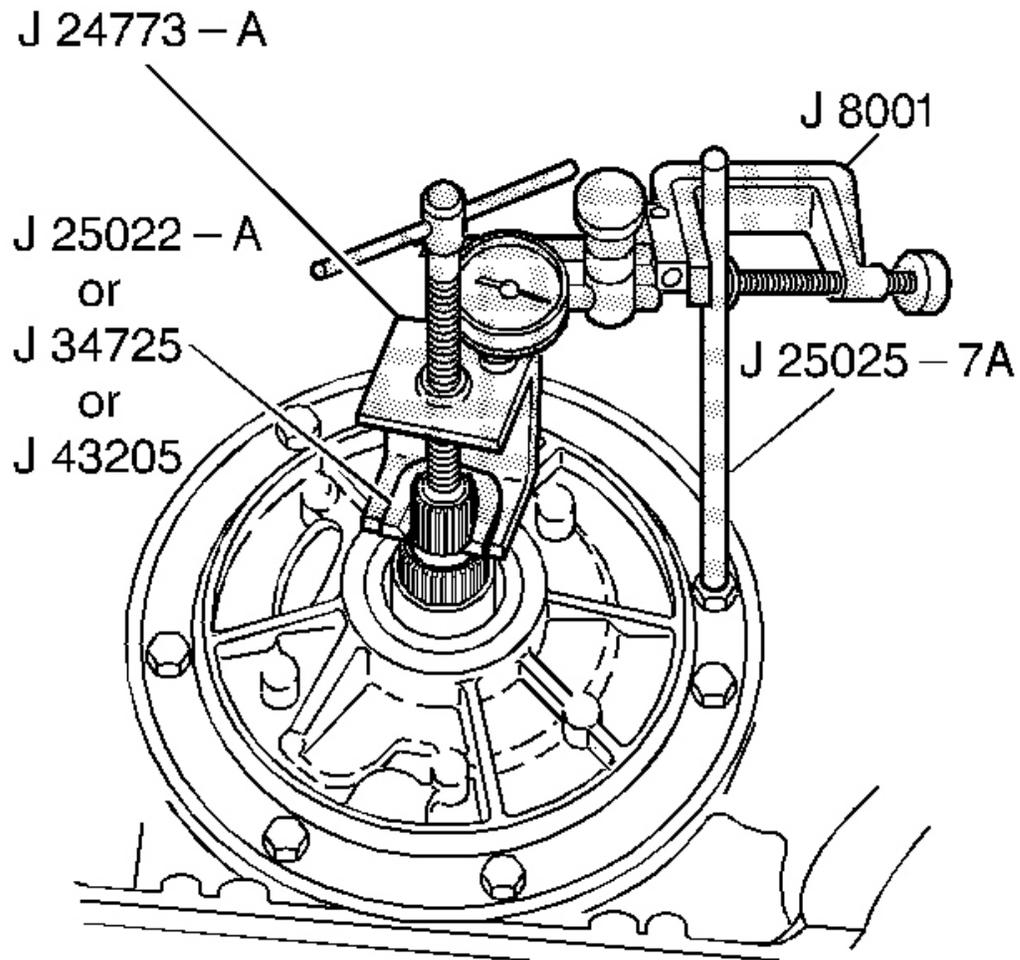
**Fig. 245: Installing J 25025-7A With J 8001**
