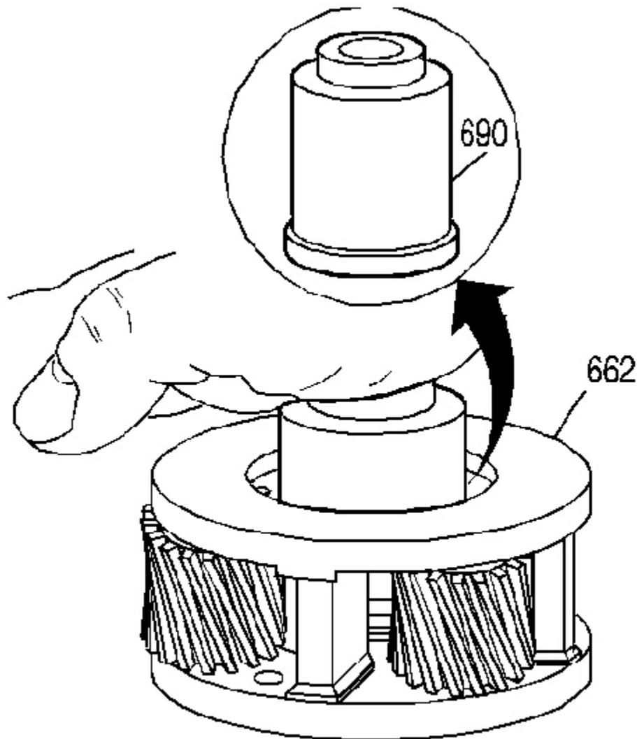
**Fig. 141: View Of Input Carrier Captive Thrust Bearing Assembly**
