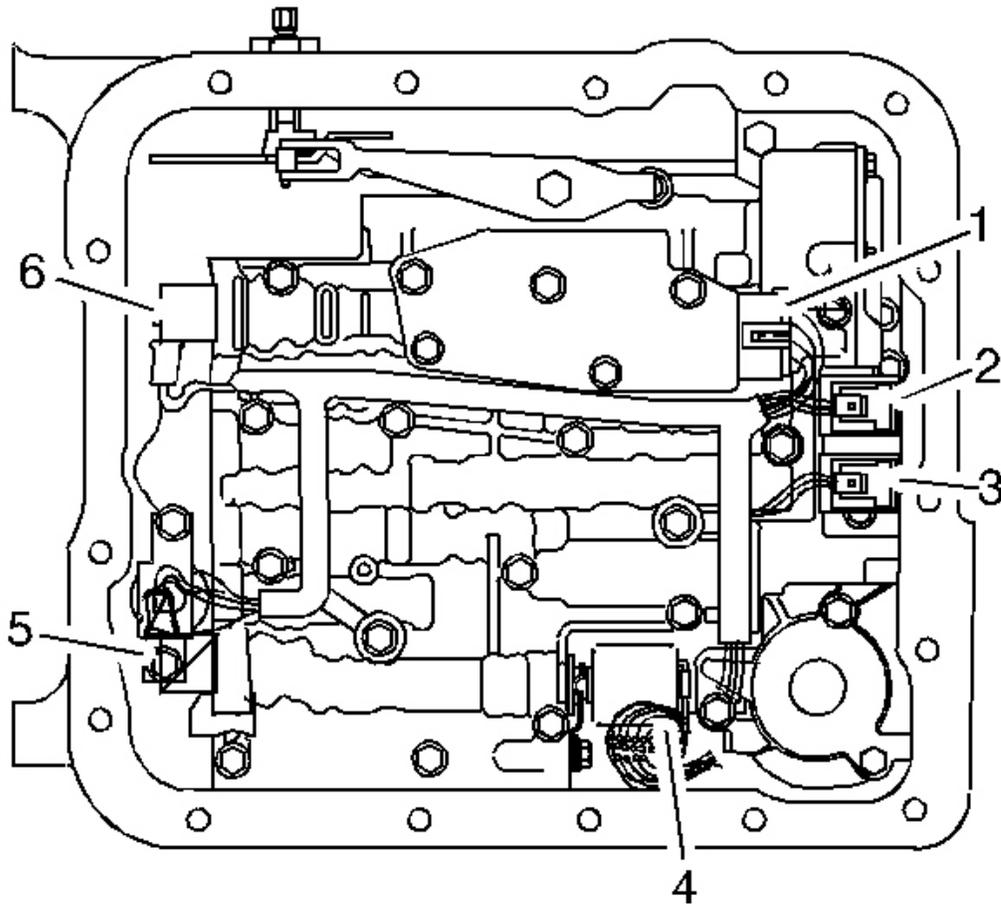
**Fig. 41: Identifying Valve Body Electrical Connections**
