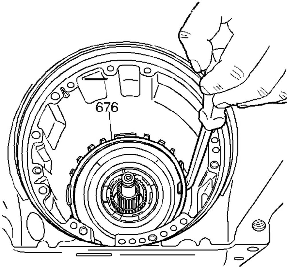
**Fig. 71: Removing Low And Reverse Support Retainer Ring**
