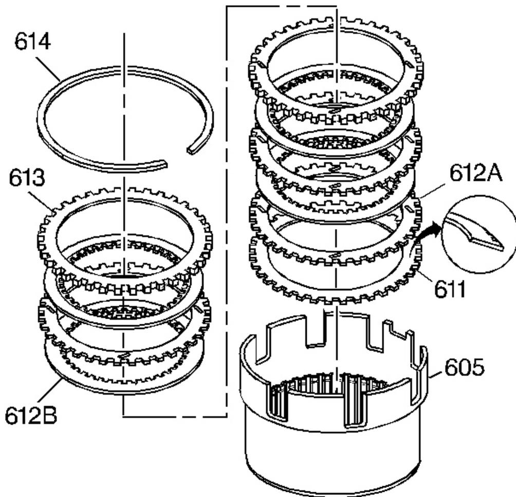
**Fig. 187: Locating Reverse Input Clutch Plates**
