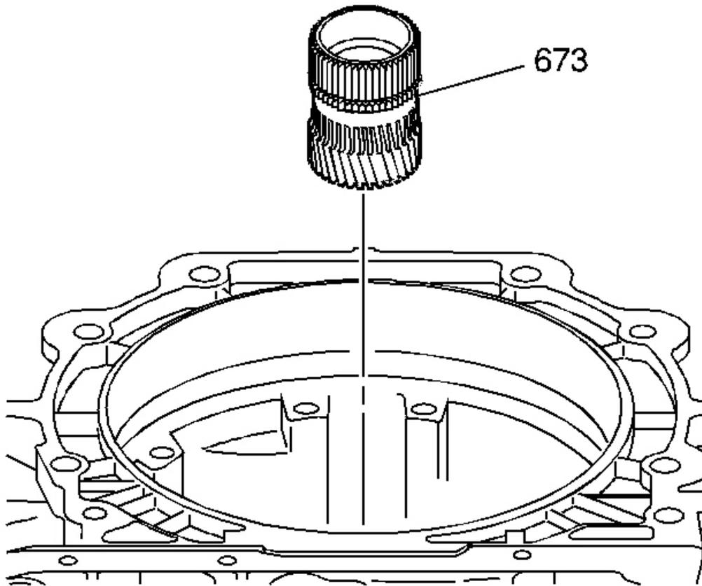
**Fig. 125: Identifying Reaction Sun Gear**
