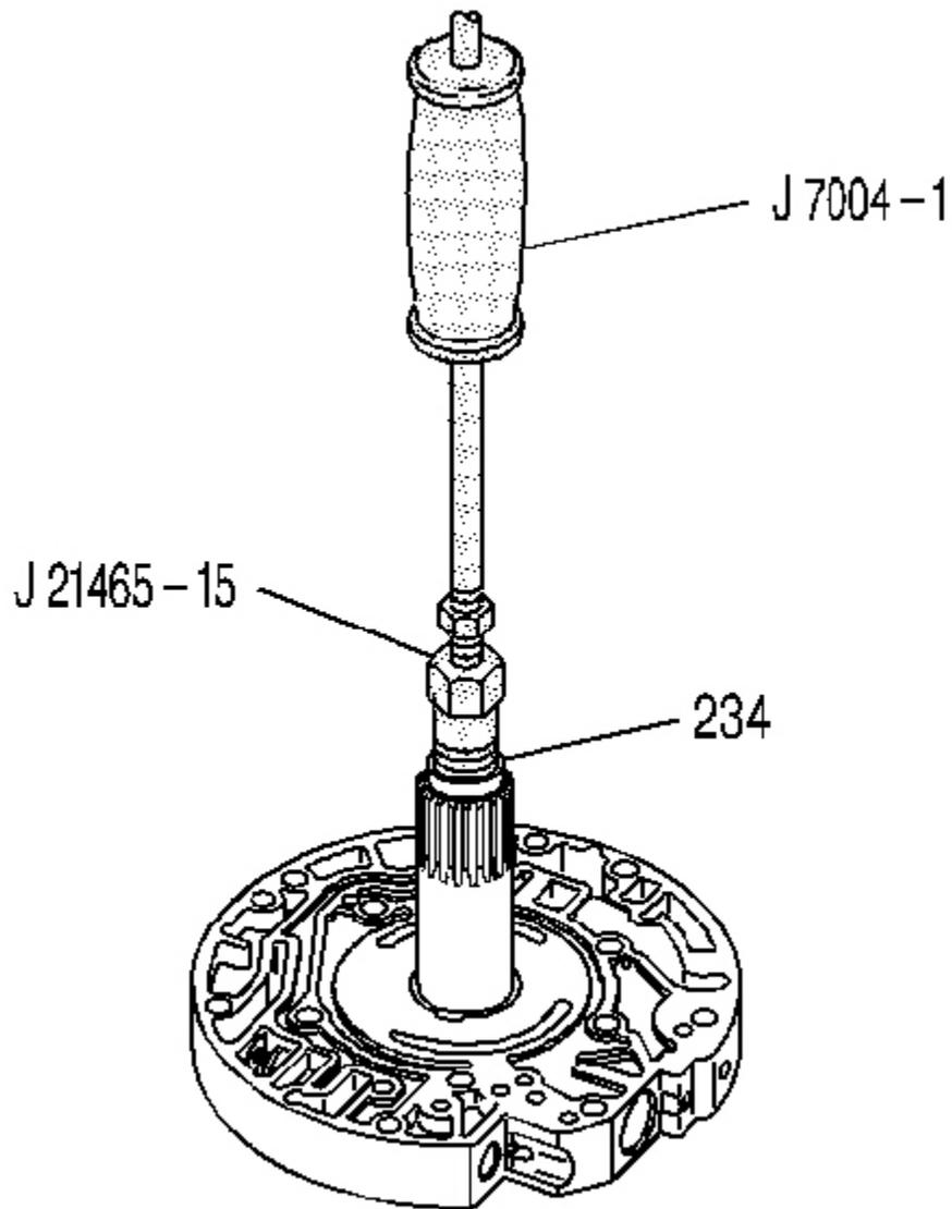
**Fig. 228: Locating Stator Shaft Front Bushing**
