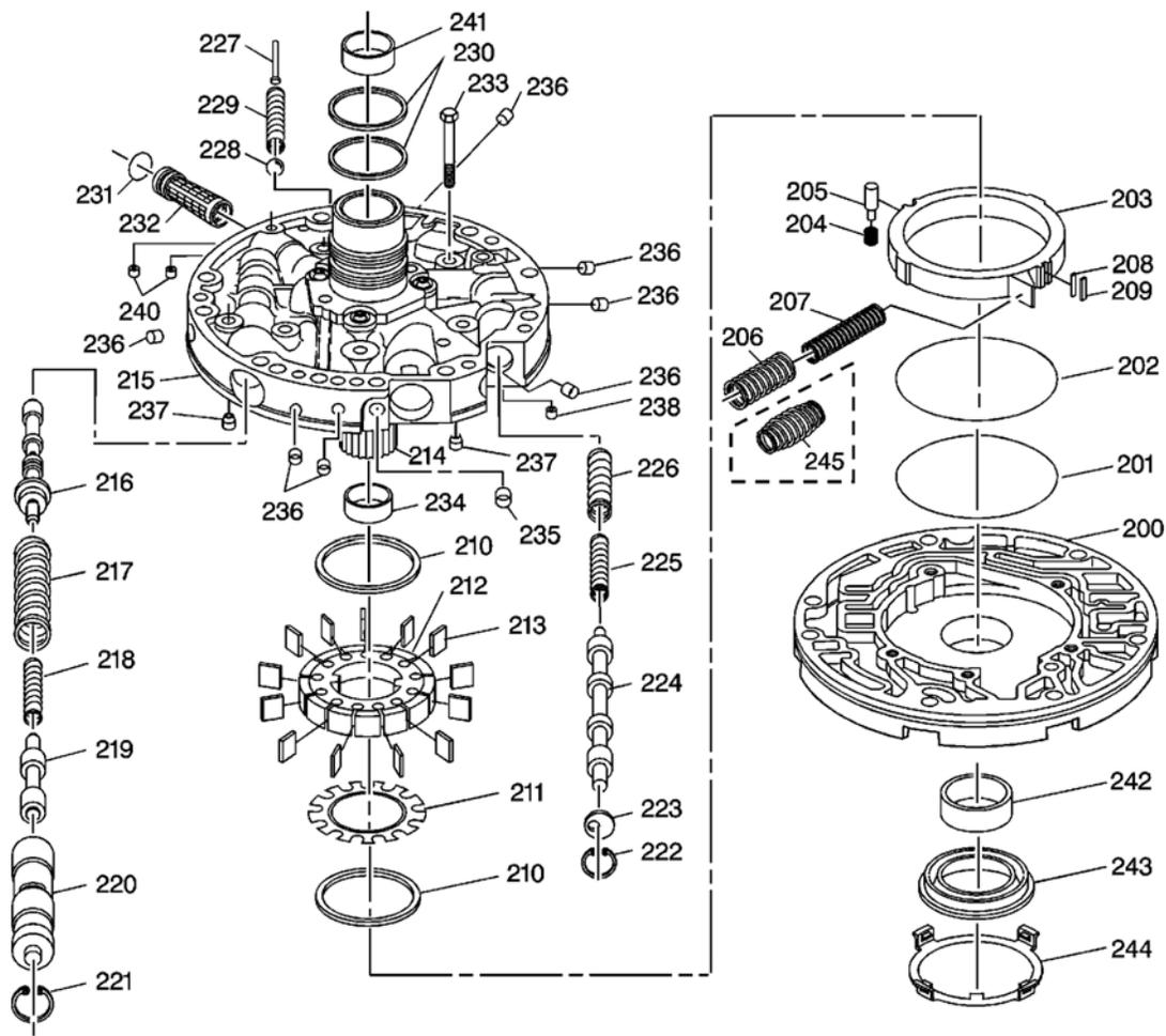
**Fig. 5: Oil Pump Assembly Disassembled View**
