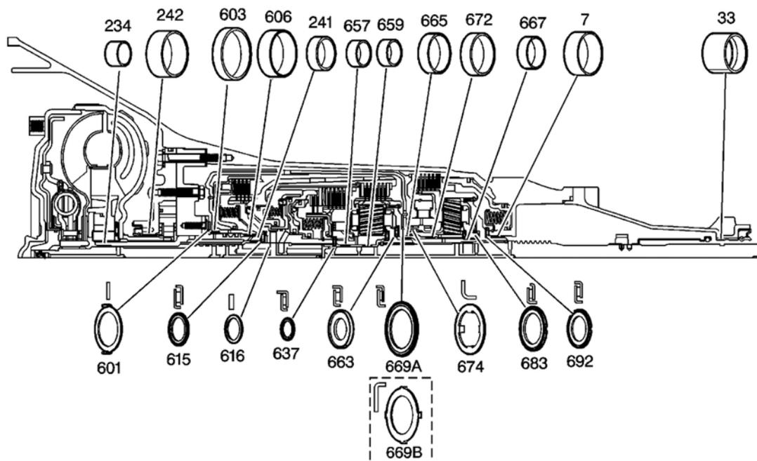
**Fig. 17: Bearings & Bushings Component Location**
