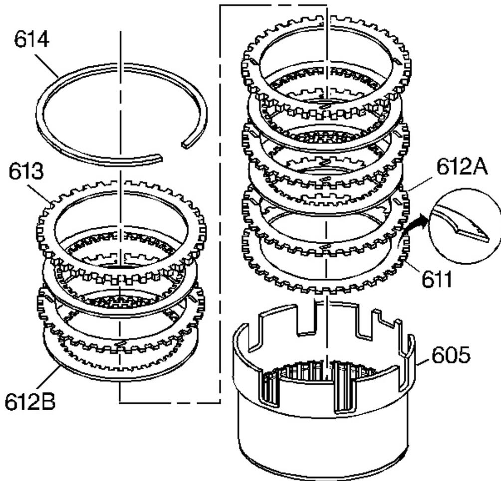
**Fig. 200: Exploded View Of Reverse Input Clutch Plates**
