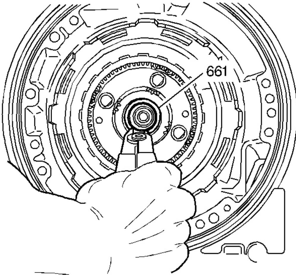
**Fig. 66: View Of Output Shaft To Input Carrier Retainer**
