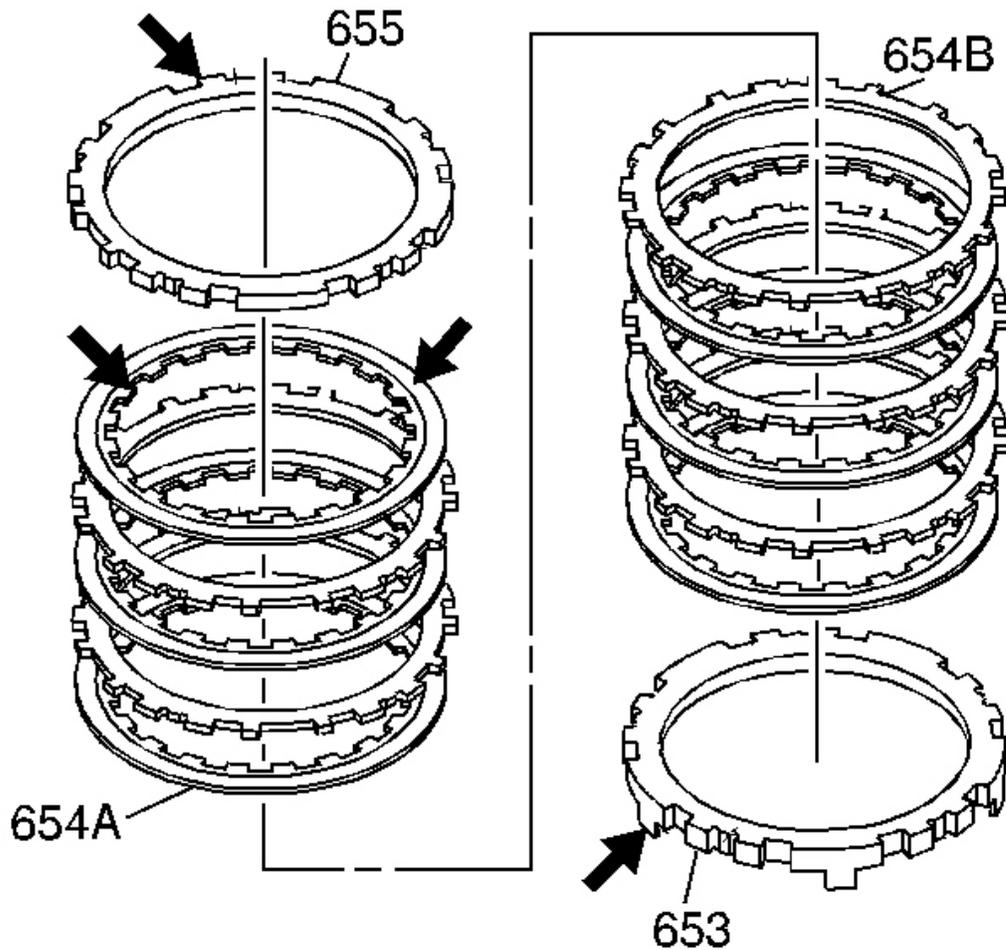
**Fig. 179: View Of Inspection Areas On Clutch Apply Plates**
