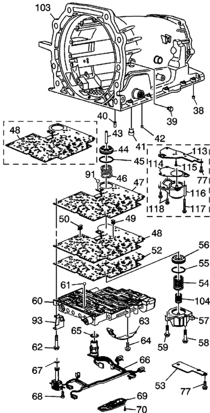
**Fig. 3: Case & Associated Parts Disassembled View (2 Of 2) - M30/M32**
