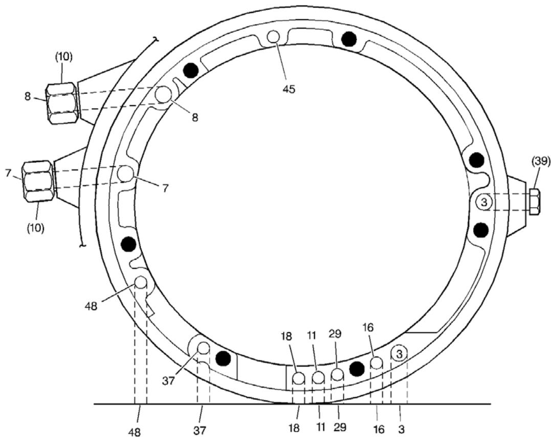
**Fig. 338: Case Fluid Passages (Pump Cover Side)**
