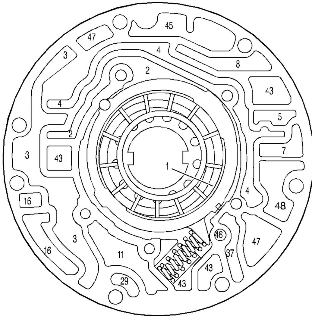
**Fig. 335: Pump Body Fluid Passages (Pump Cover Side)**
