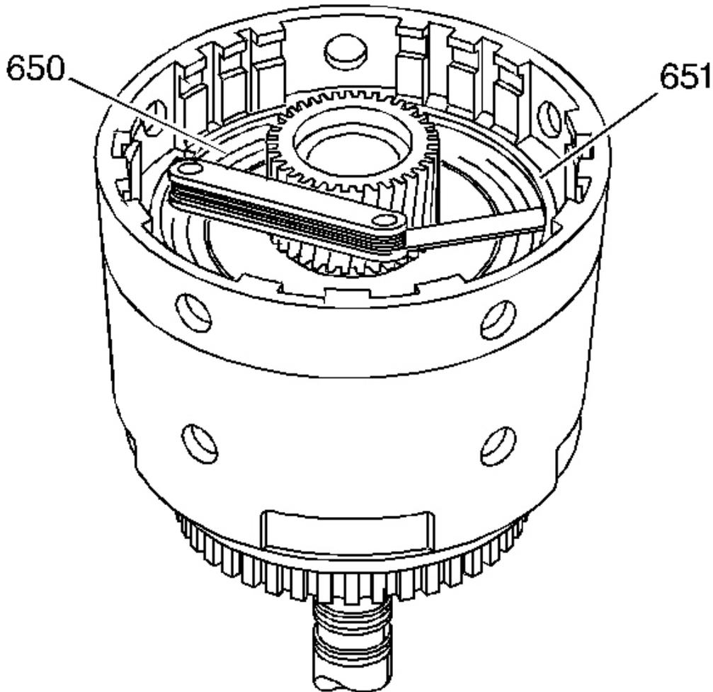
**Fig. 178: Measuring Forward Clutch Plate Travel**
