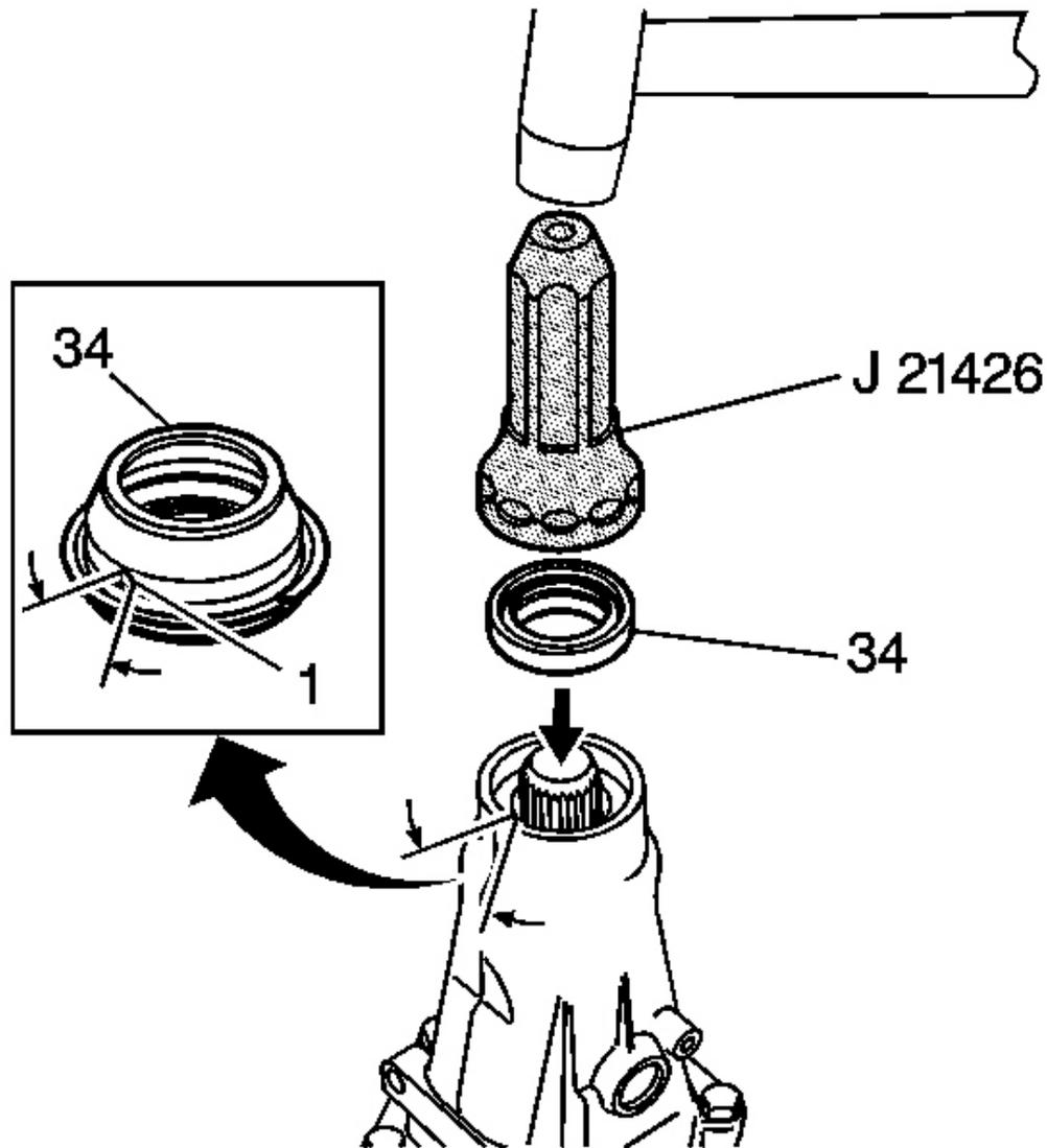
**Fig. 318: Locating Case Extension Oil Seal Assembly**
