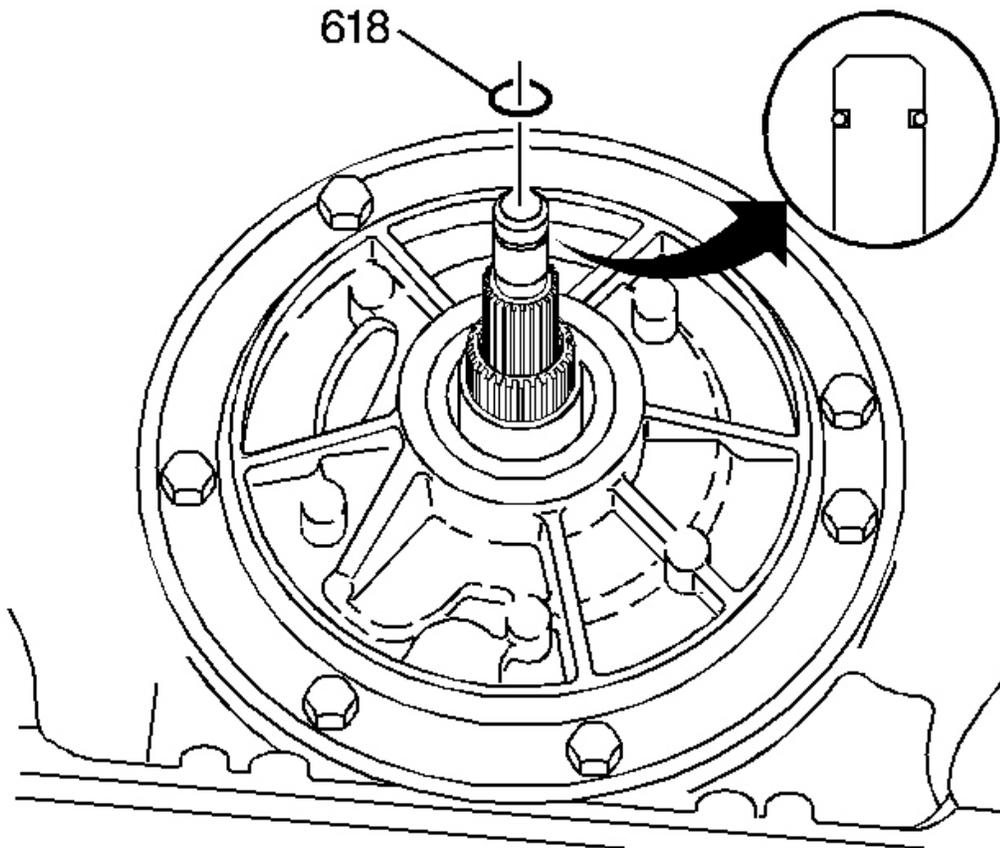
**Fig. 55: Identifying Turbine Shaft O-Ring**
