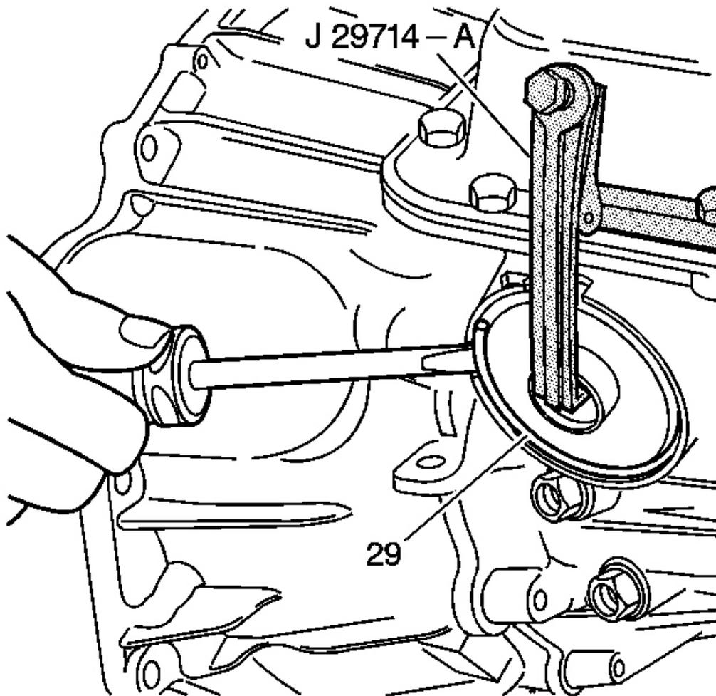
**Fig. 28: Locating Servo Cover Retaining Ring**
