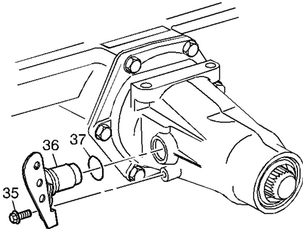
**Fig. 33: View Of Internal Transmission Speed Sensor**
