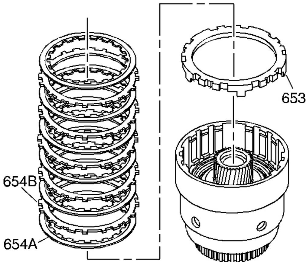
**Fig. 180: Installing Clutch Apply Plates Into Input Housing**
