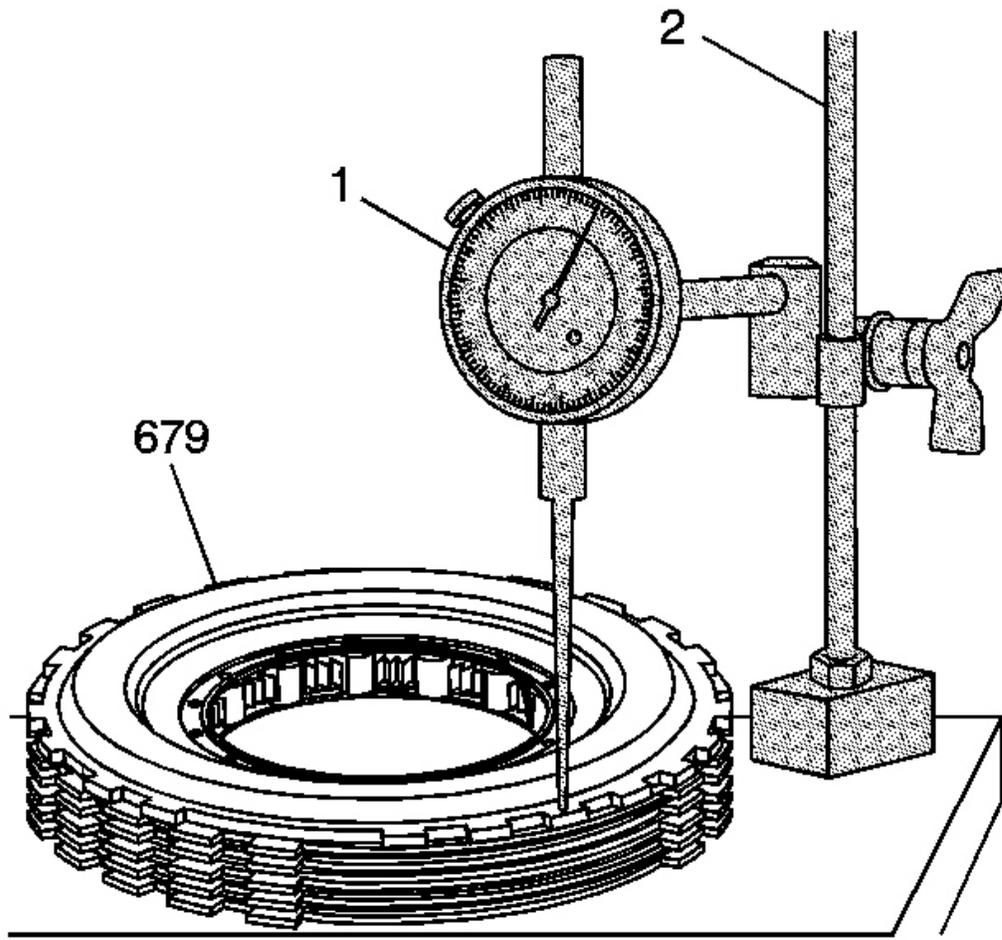
**Fig. 113: Measuring Clutch Pack Height With J 8001**
