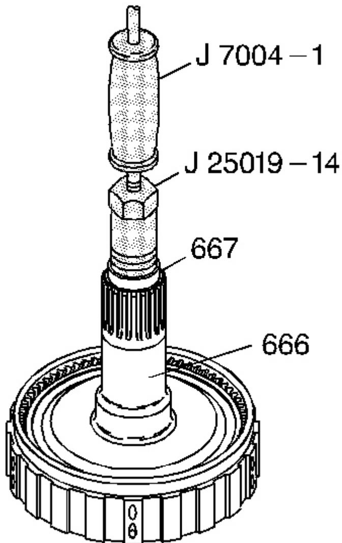
**Fig. 129: Using J 25019-14 & J 25019-14 To Remove Reaction Carrier Shaft Rear Bushing**
