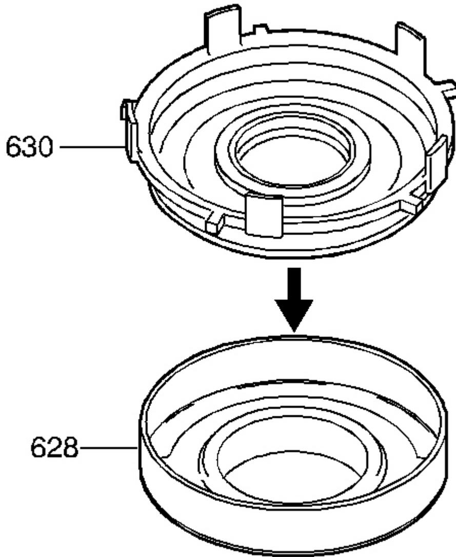
**Fig. 157: Installing Forward Clutch Piston**
