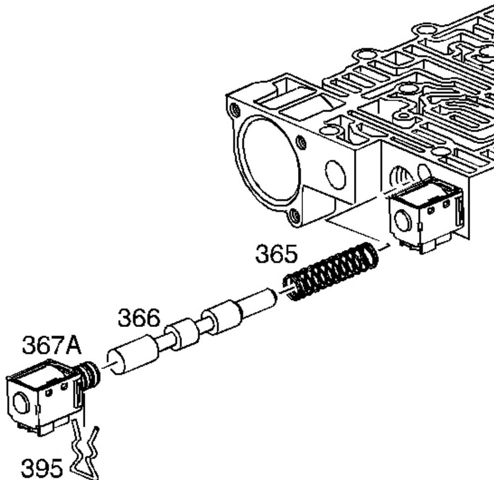
**Fig. 269: Locating 1-2 Shift Valve & Solenoid Components**
