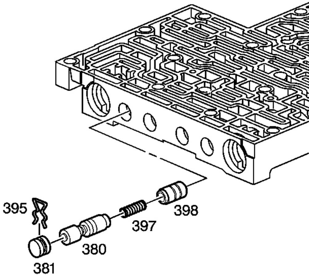
**Fig. 258: Identifying Isolator Valve & Regulator Apply Valve**
