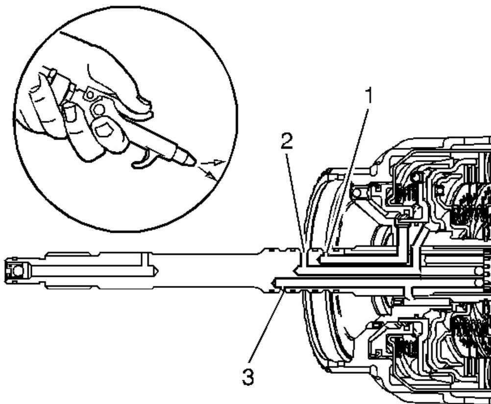
**Fig. 185: Applying Air To Check Overrun Clutch**
