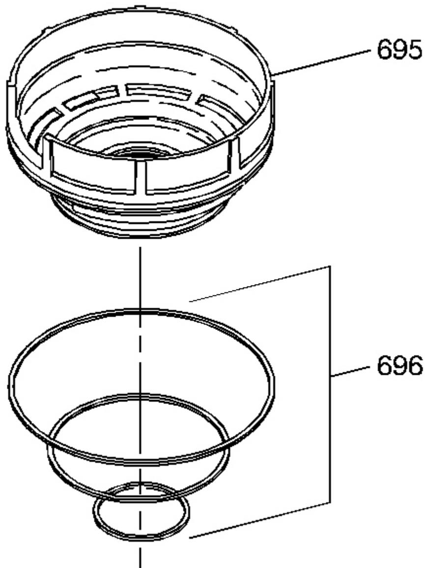
**Fig. 100: Installing Transmission Seals Onto Low And Reverse Clutch Piston**
