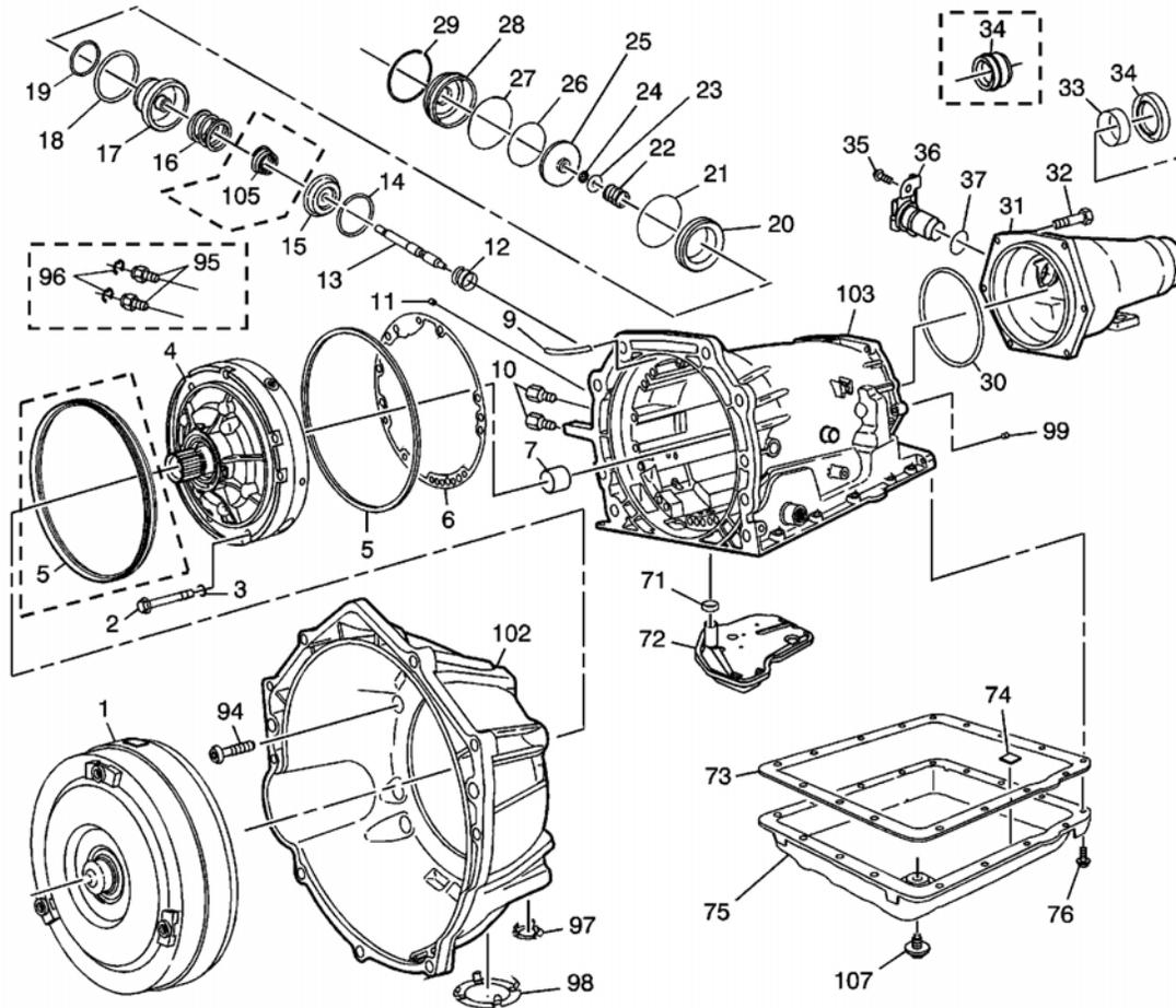
**Fig. 2: Case & Associated Parts Disassembled Views (1 Of 2)**
