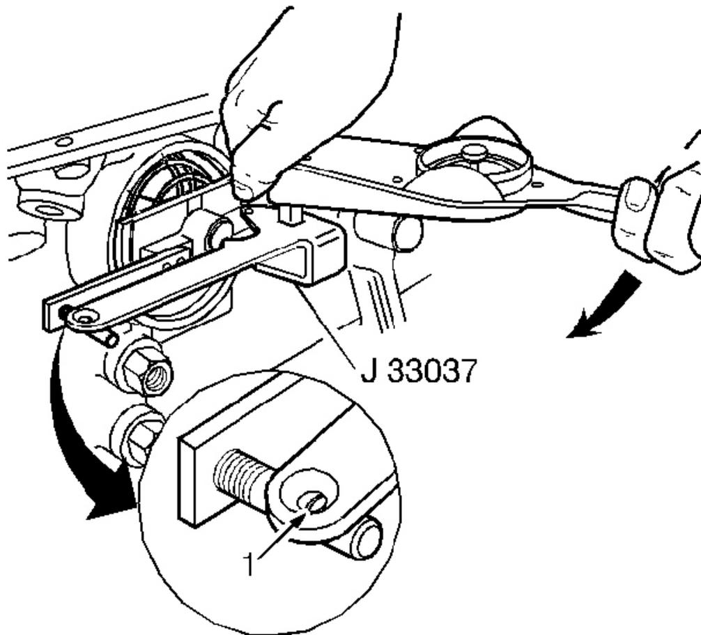
**Fig. 302: Identifying Gage Slot**
