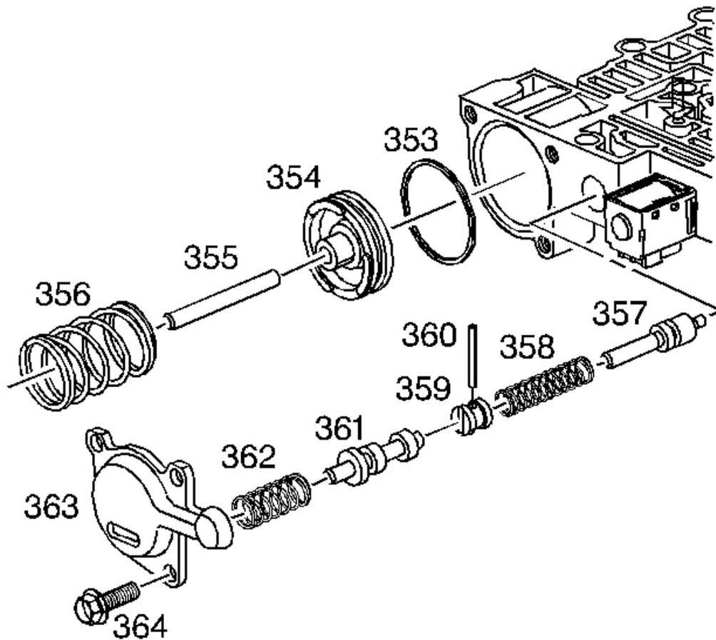
**Fig. 250: Exploded View Of Forward Abuse & Low Overrun Components**
