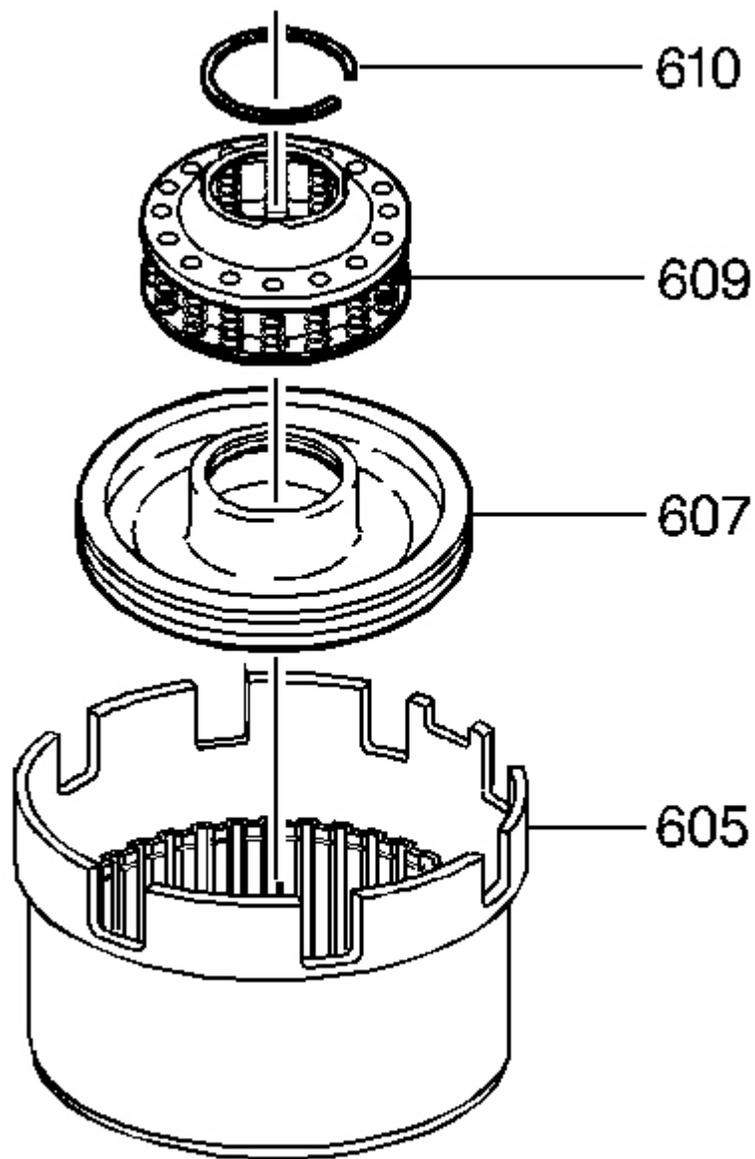
**Fig. 189: Identifying Reverse Input Clutch Spring & Piston Assemblies**
