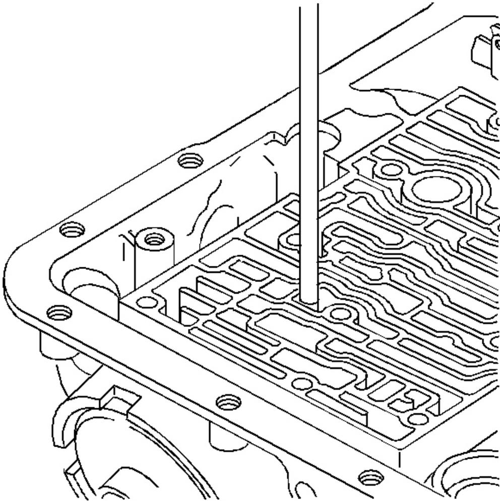
**Fig. 95: Checking Third Accumulator Retainer And Ball Assembly Alignment**
