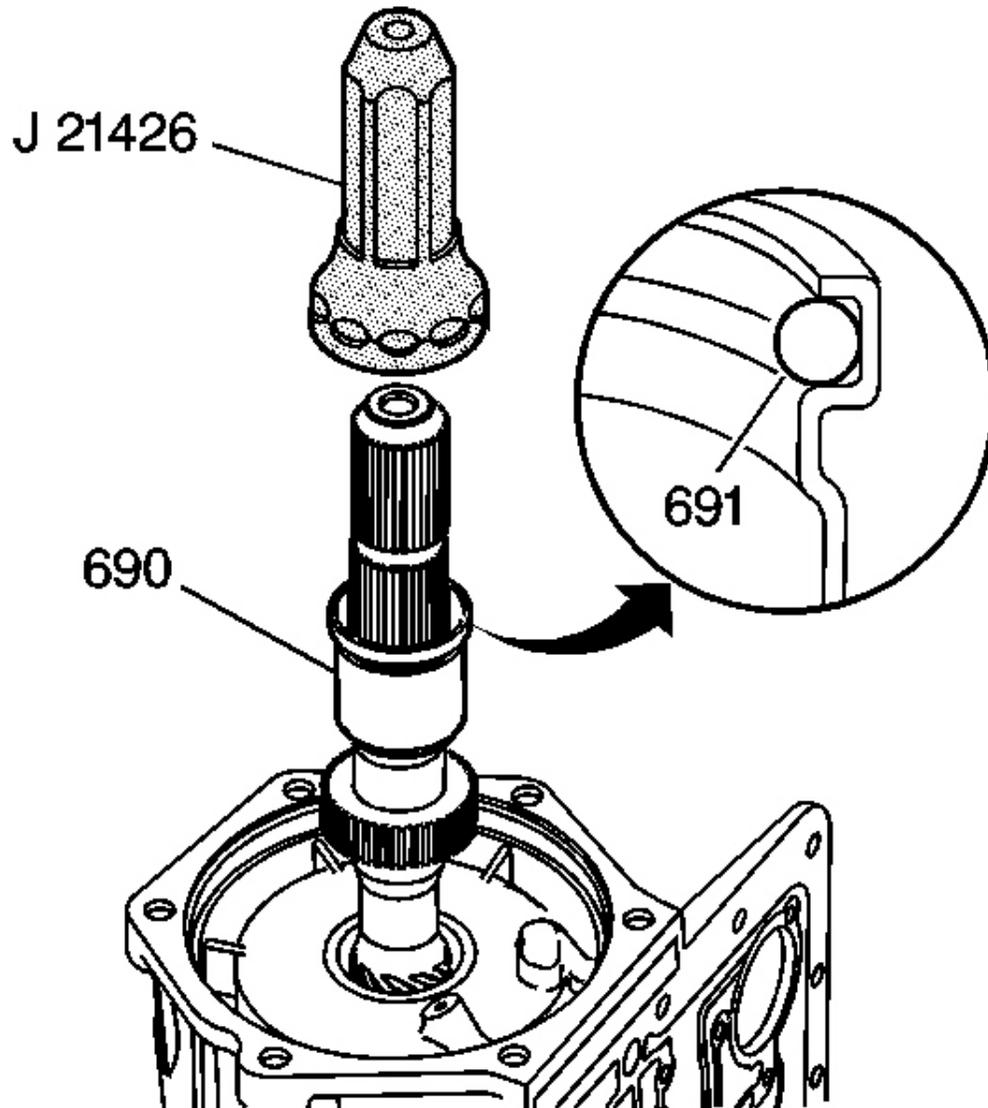
**Fig. 314: Cross Sectional View Of Output Shaft Seal**
