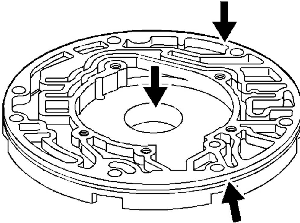
**Fig. 212: Identifying Oil Pump Body Inspection Areas**
