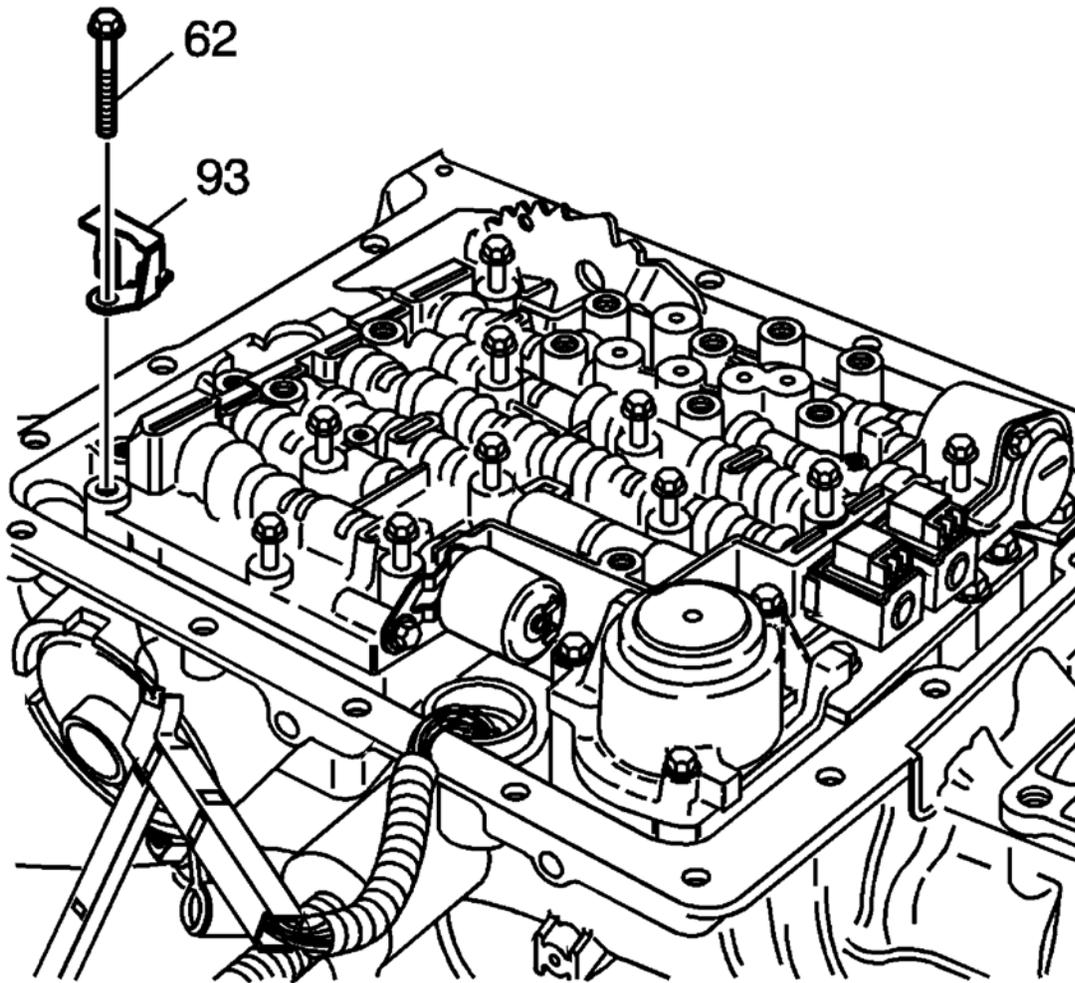
**Fig. 286: Locating Fluid Level Indicator Stop Bracket & Valve Body Bolts**
