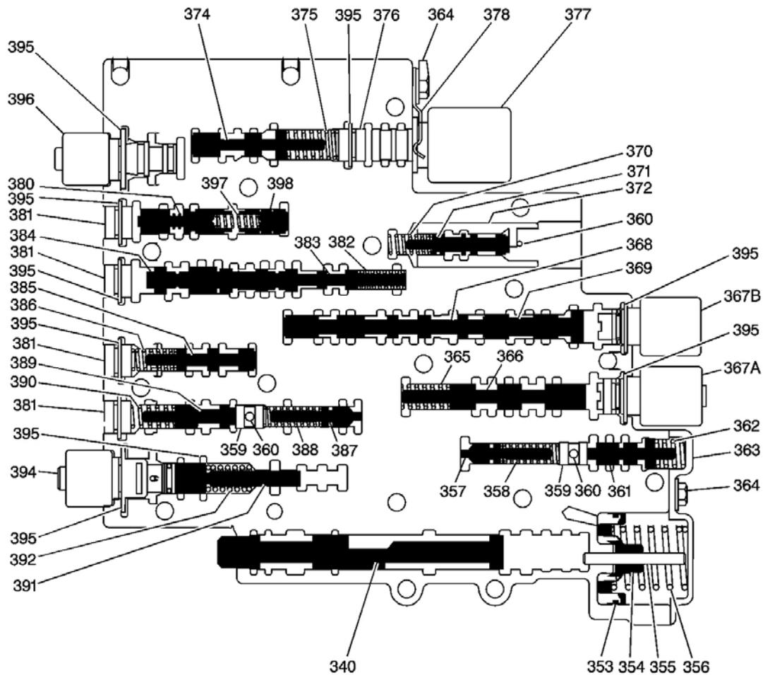
**Fig. 18: Valve Trains Component Location**
