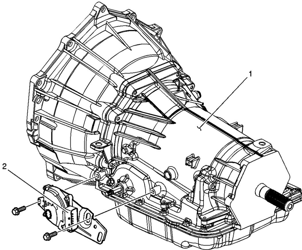
**Fig. 12: Park Neutral Position (PNP) Switch Component View**
