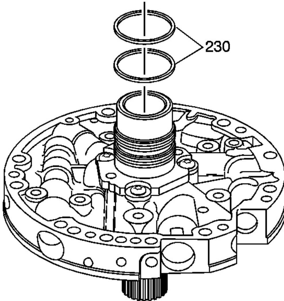
**Fig. 225: Locating Stator Shaft Oil Seal Rings**
