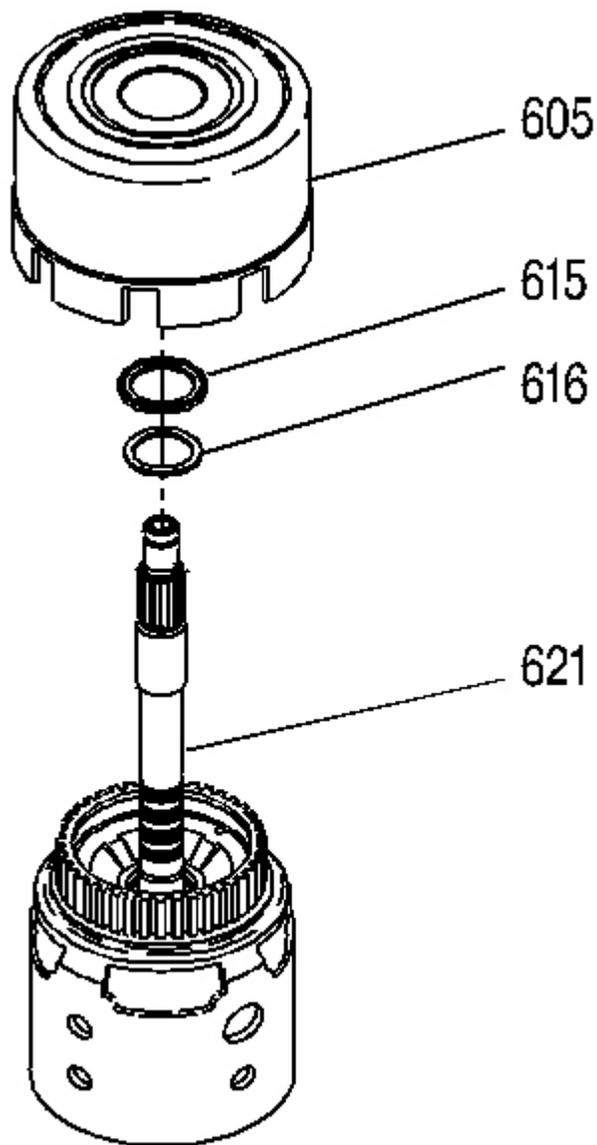
**Fig. 145: View Of Stator Shaft/Selective Washer Bearing Assembly**
