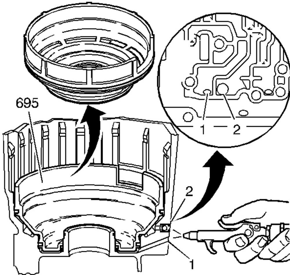
**Fig. 84: Blowing Air Into Case Passage**
