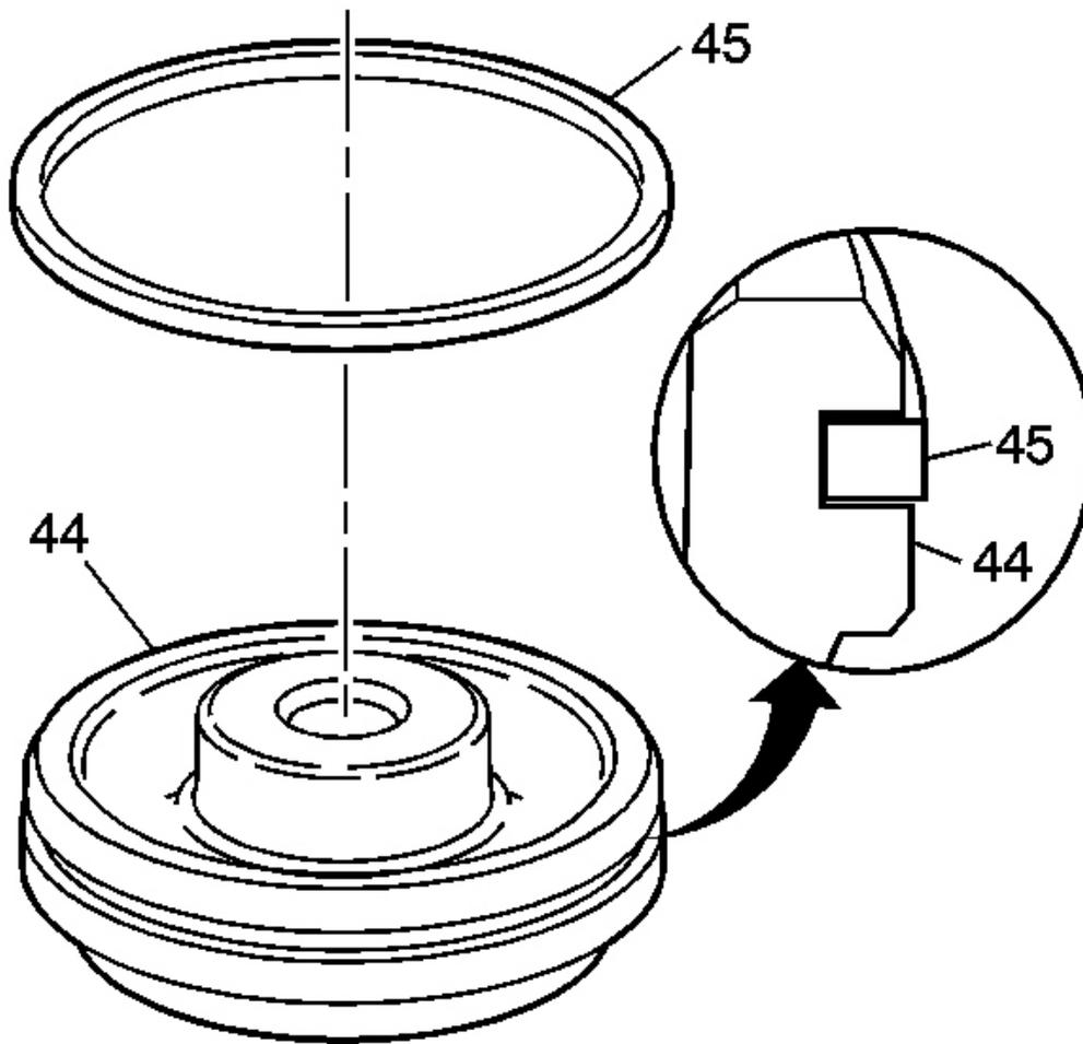
**Fig. 272: Identifying Inspection Areas On 3-4 Accumulator Piston**
