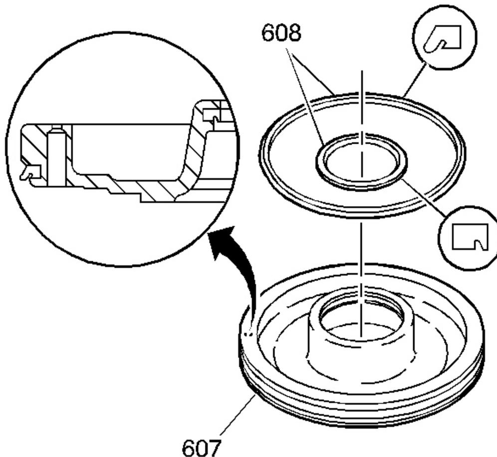
**Fig. 195: Locating Inspection Areas On Reverse Input Clutch Piston**
