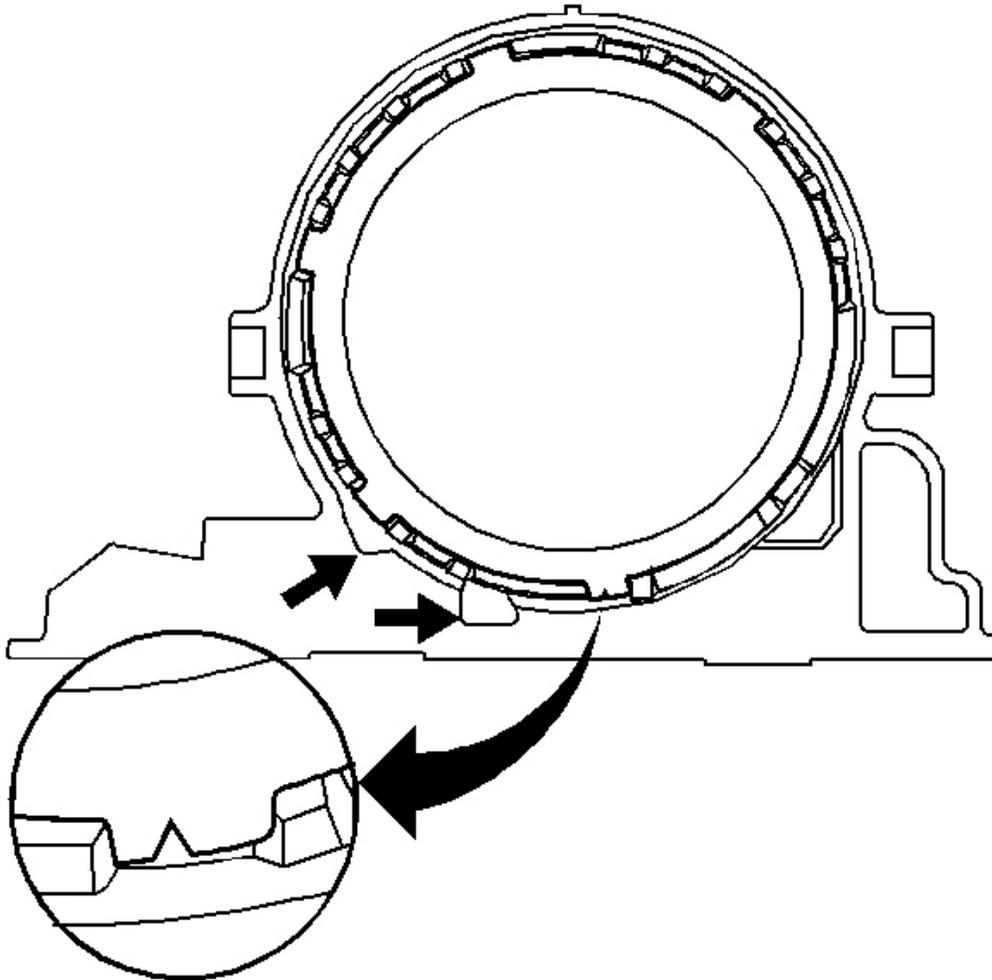
**Fig. 115: Illustrating Steel Plate Spline Alignment**
