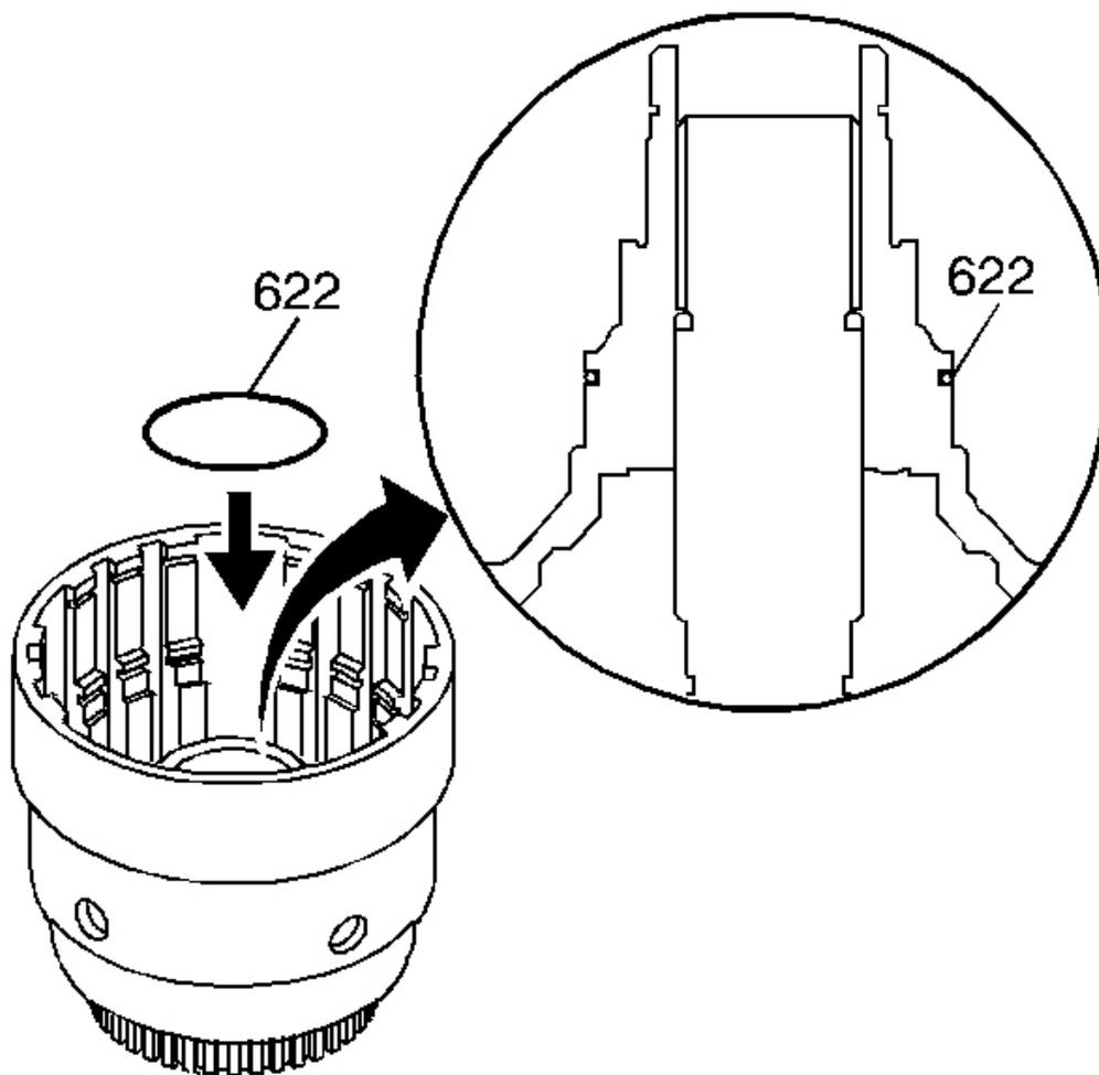
**Fig. 153: Locating Forward Clutch Housing O-Ring Seal**
